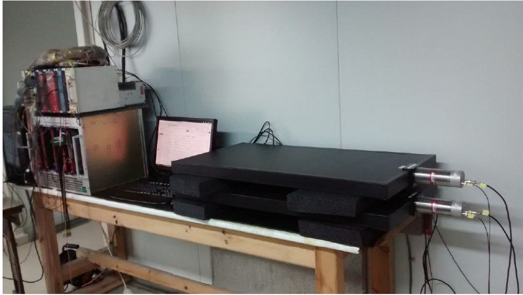
Figure 2.20: Plastic scintillators test bench set-up at LSC.
