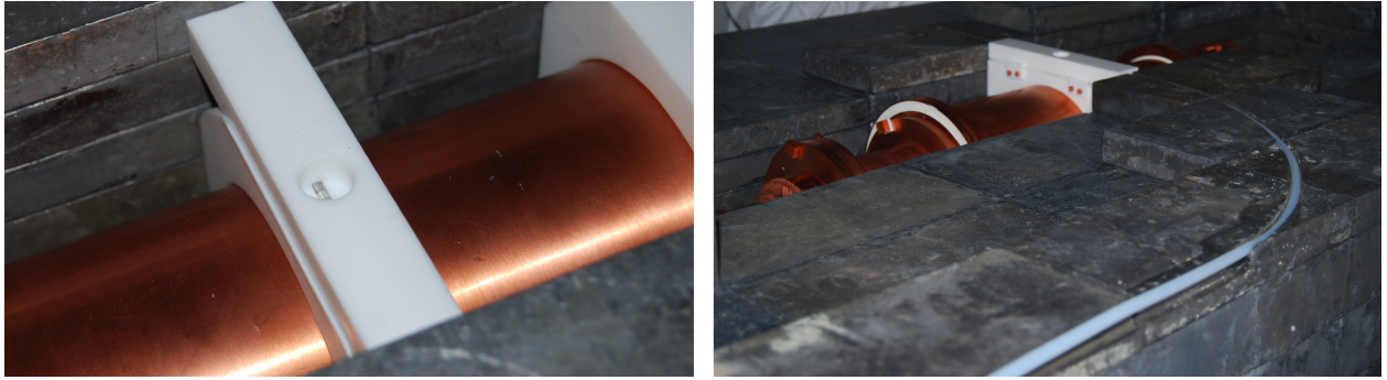
Figure 2.14: New calibration system with two radioactive sources ( ^{57}\text{Co} and ^{109}\text{Cd} ) mounted along a flexible wire.
