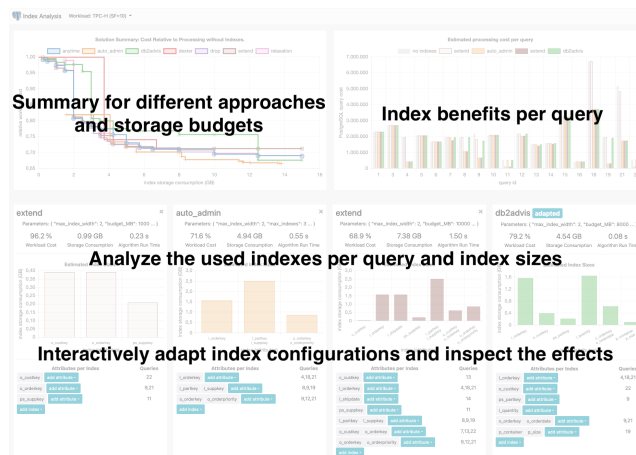
Figure 1: Demo summary: Evaluating database index selection approaches and analyzing the chosen indexes.
