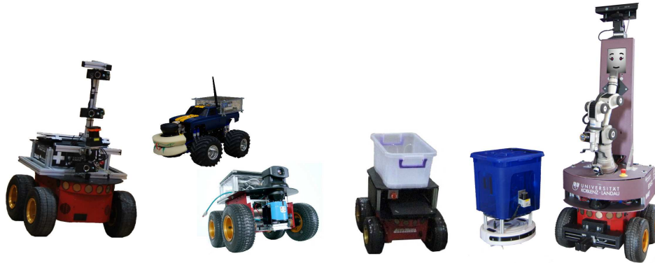
Figure 1: Our robots using the Robbie system architecture. From left to right: Rescue robot Robbie (2011), robots for SICK Robot Day (on commercial racing car (2007) and with a Pioneer3AT-platform (2010)), cleaning and disposal robot Waylon (2010) and GiGo (Roomba 531 from iRobot as platform, 2011), household robot Lisa for RoboCup@Home (2011).
