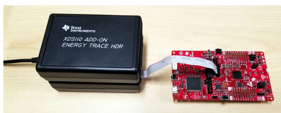
Figure 2-23. CC3235x Device Test Setup With XDS110 System
