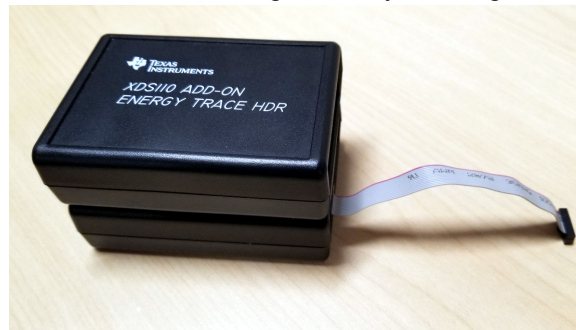
Figure 2-15. XDS110 Probe and ETHDR System
