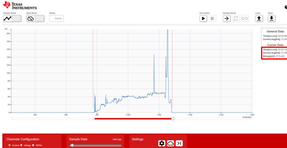
Figure 2-12. Average Current Measurement With IMETER-BOOST Device
