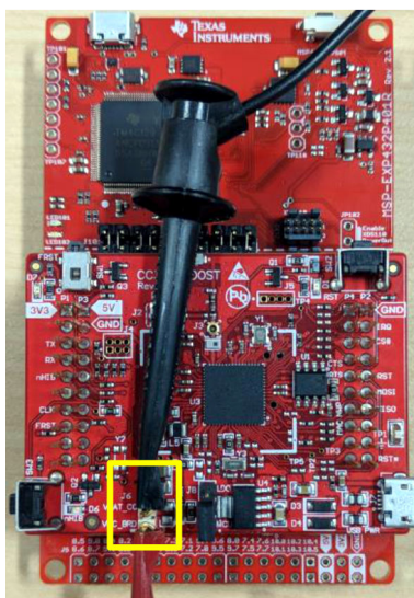
Figure 2-9. Current Measurement Tool Connection to CC3135 Device
