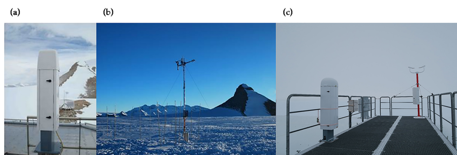
Figure 3. (a) The Vaisala CL-31 ceilometer on the roof of PE station; (b) the IMAU automatic weather station at PE; (c) the Vaisala CL-51 ceilometer on the roof of Neumayer III station (credits: Hauke Schulz).
