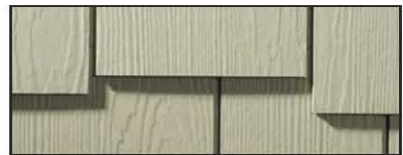
CEMETITIUS SHINGLE - STAGGERED EDGE 6" MIN. TALL SIDING EXPOSURE Thickness: 1/4" Height: 1.9 lbs./sq. ft. Size: 48" x 15.875" panels
