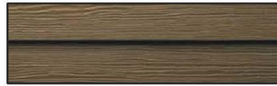
CEMENTITIOUS LAP SIDING - CEDARMILL 8" TALL SIDING EXPOSURE Actual Width: 9.25" Thickness: 5/16" Height: 2.3 lbs./sq. ft. Length: 12' planks
