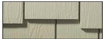
EMERALD SHINGLE - STAGGERED EDGE 6" MIN. TALL SIDING EXPOSURE Thickness: 1/4" Weight: 1.9 lbs./sq. ft. Size: 48" x 15.875" panels
