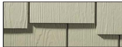
CEMENTITIOUS SHINGLE - STAGGERED EDGE 6" MIN. TALL SIDING EXPOSURE Thickness: 1/4" Height: 1.9 lbs./sq. ft. Size: 48" x 15.875" panels
