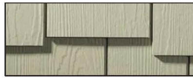
EMERALD SHINGLE - STAGGERED EDGE 6" MIN. TALL SIDING EXPOSURE Thickness: 1/4" Height: 1.9 lbs./sq. ft. Size: 48" x 15.875" panels
