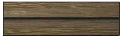
CEMETITIOUS LAP SIDING - CEDARMILL 8" TALL SIDING EXPOSURE Actual Width: 9.25" Thickness: 5/16" Height: 2.3 lbs./sq. ft. Length: 12' planks
