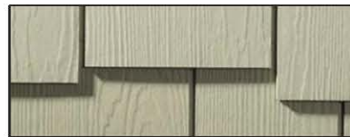
EMERALD SHINGLE - STAGGERED EDGE 6" MIN. TALL SIDING EXPOSURE Thickness: 1/4" Height: 1.9 lbs./sq. ft. Size: 48" x 15.875" panels
