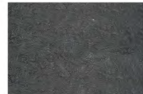
ALL BLACK In Rough&Ready: 7x15 cm | 2.8x5.9" Recycled industrial and agriculture plastics 100% Recycled PE & PP Density: 800 kg/m 2
