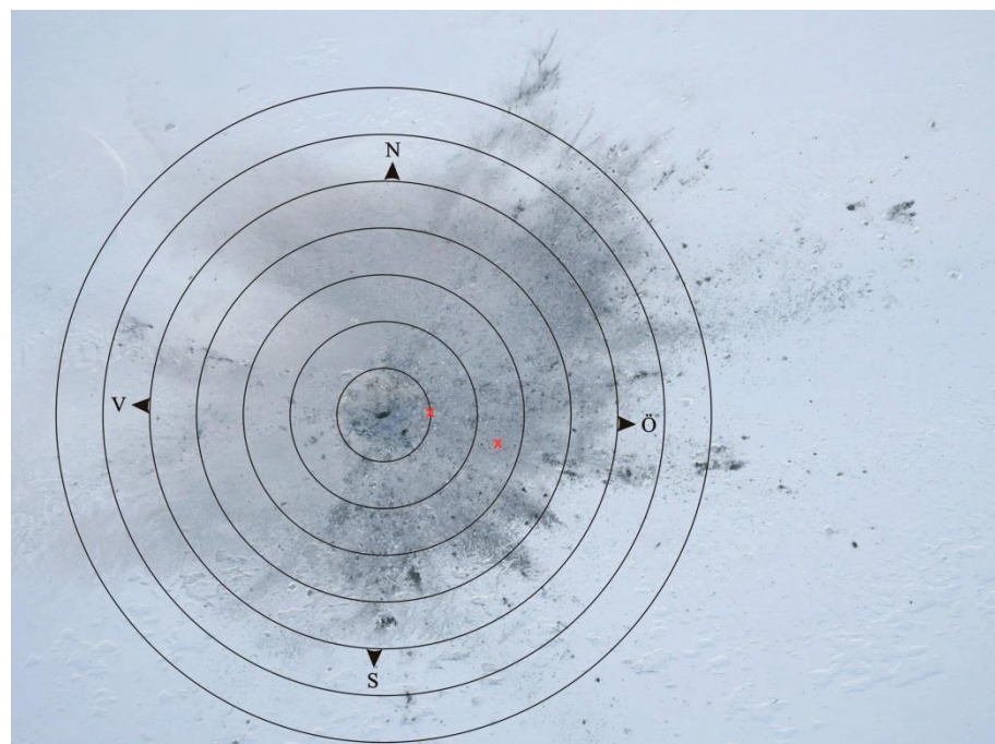
Figure 5. Accident site with 10 meter distance circles. CVR was found at the red cross closest to the center, FDR at the second cross. (Photo: Swedish Police).
