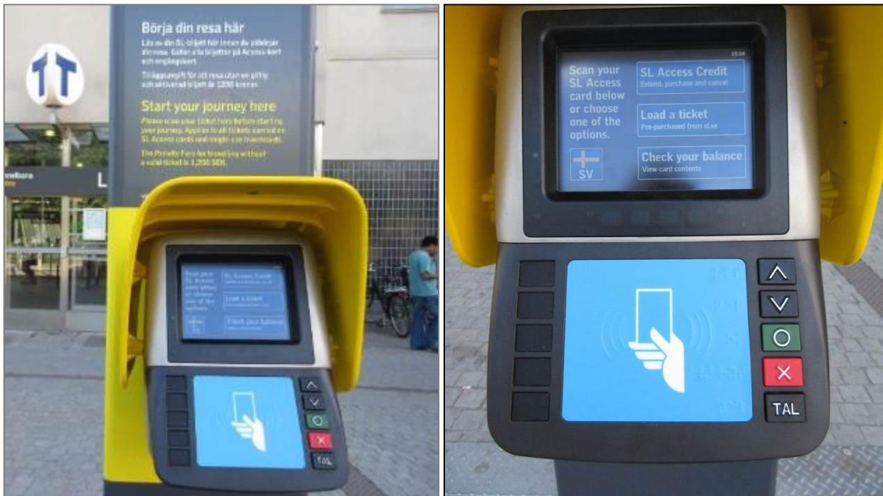
Image 2: Close-up of an accessible ticket machine in Stockholm for activating, changing and validating tickets (Trafikförvaltningen Stockholms Läns Landsting, 2018).
