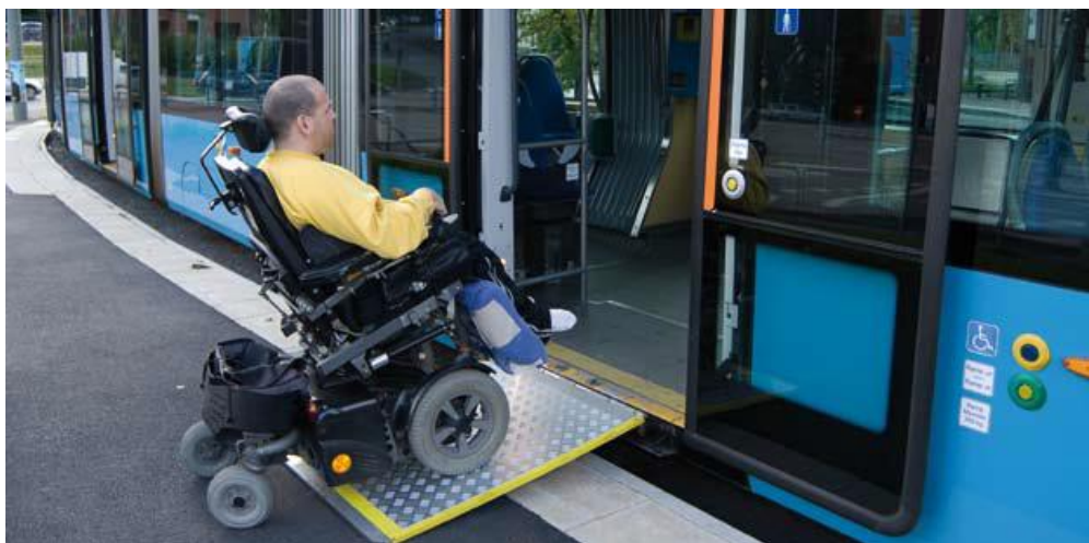
Figure 122: Electric and manual ramp for helping people in wheelchairs (Source: Peter Svenson, Stig Hedström, Lillemor Bulukin)
