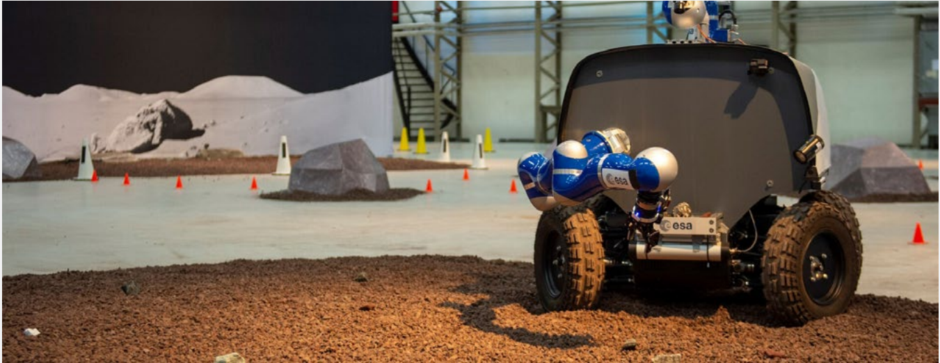
Figure 2. The ESA ground robot collecting rock samples, controlled from space.
