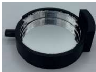
Supplementary Figure 39: reactor support bottom part with mirror.
