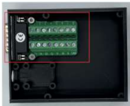
Supplementary Figure 47: Installation of 15 pin male connector (Step 1).
