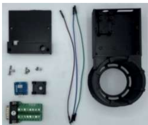
Supplementary Figure 32: 3D printed and electronic components of the Phototemperature sensor Module.
