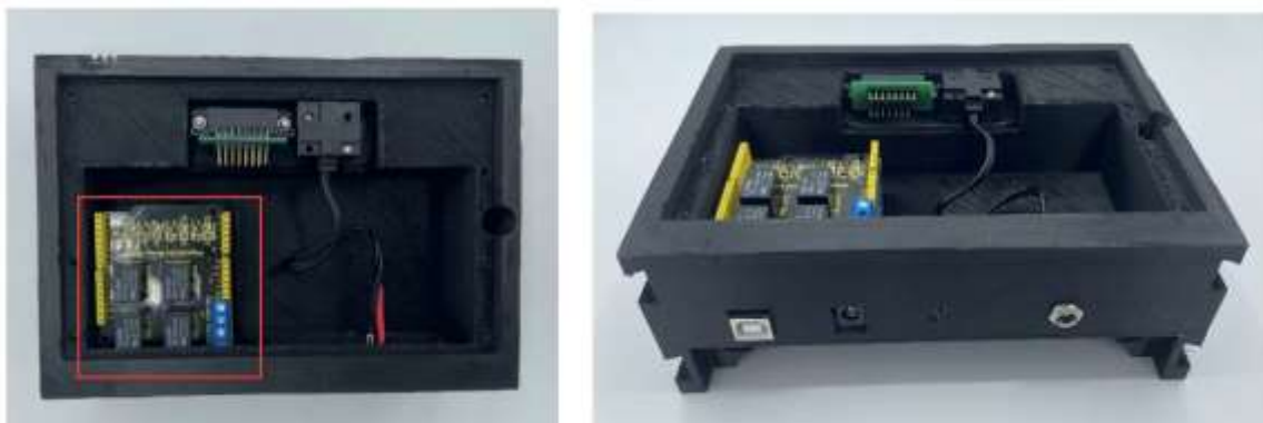
Supplementary Figure 12: installation of the relay shield.
