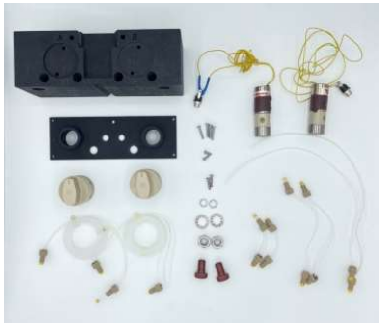
Supplementary Figure 66: Components of the Injection block.
