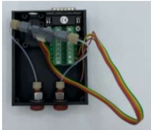
Supplementary Figure 49: Wire connections of the sensor.
