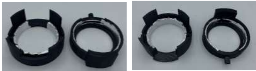
Supplementary Figure 38: reactor support covered in reflective aluminium film.
