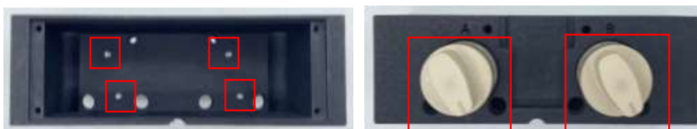
Supplementary Figure 69: installation of two 6-port loop injection valves.
