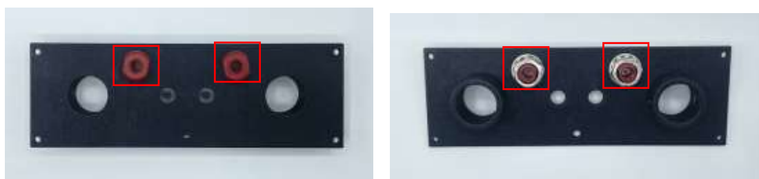
Supplementary Figure 67: installation of union body, lock washer and nut to the injection block lid.
