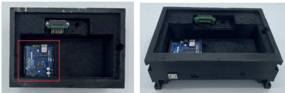
Supplementary Figure 11: installation of the Arduino board.
