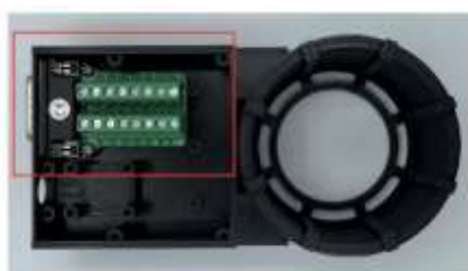
Supplementary Figure 33: Installation of 15 pin male connector (Step 1).
