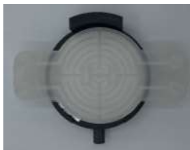
Supplementary Figure 40: 3D printed reactor on top of the reactor support bottom part.
