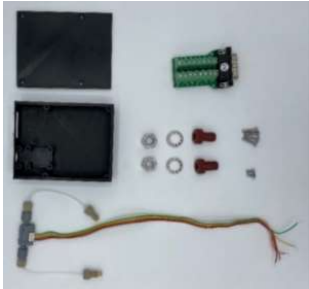
Supplementary Figure 46: 3D printed and electronic components of the flow rate sensor Module.
