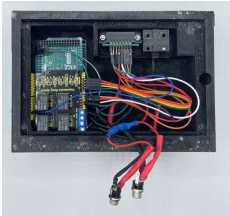
Supplementary Figure 59: Arduino Mega board wire connections.
