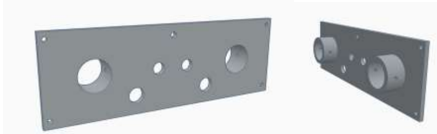
Supplementary Figure 62: Tinkercad design illustrating the scale up Injection block lid.
