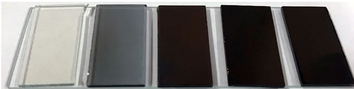
Fig. S1 Pristine FTO-coated silica glass substrate (whitish, far left) and such substrates overlain with gray to darkish films by PLA of rutile polycrystal target for 30 min in vacuum under 200, 400, 600, and 800 mJ/pulse, respectively from left to right.
