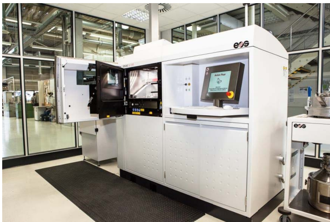
Fig. S5 EOS DMLS System (for details see: http://www.shapetec.at/kompetenzen/metall-laser-sintern (accessed October 20, 2017)).
