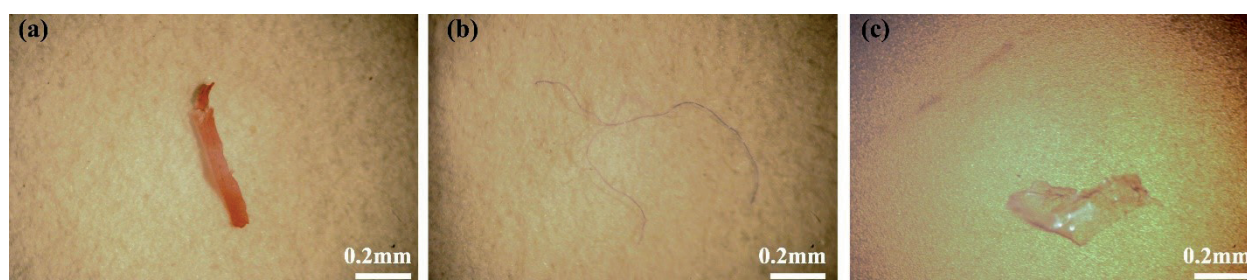
Fig. 1. Stereoscopic microscope (Optika SZM-2) MPs photographs illustrating shapes: fragment, fiber, and d film.
