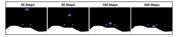
More specifically, the agent observes eight aspects of the state, including six continuous and two discrete elements. Based on the observed elements, the agent knows its location, direction, speed of movement, and whether it has (partially) landed. However, it does not know where it should be moving using its available actions or observe the inner state of the environment in the sense of understanding the rules that govern its motion.
