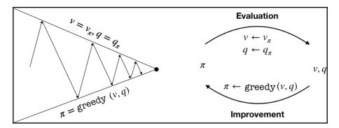
Convergence requires that the value function is consistent with the policy, which in turn needs to stabilize while acting greedily with respect to the value function. Thus, both processes stabilize only when a policy has been found that is greedy with respect to its own evaluation function. This implies that the Bellman optimality equation holds, and thus that the policy and the value function are optimal.
