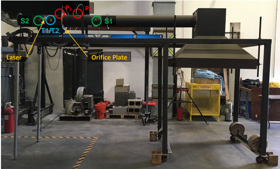
Figure 4-1 100 kW Calorimeter Located at the Jensen Hughes Baltimore Test Facility
