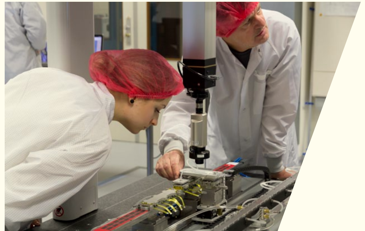
Testing sensor staves for ALICE.
