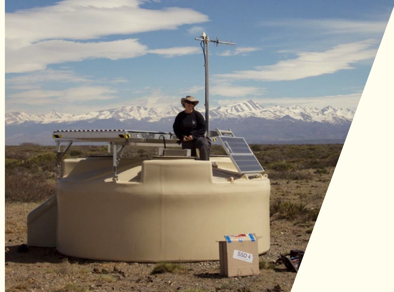
Water tank detector at the Pierre Auger cosmic ray observatory, Argentina.
