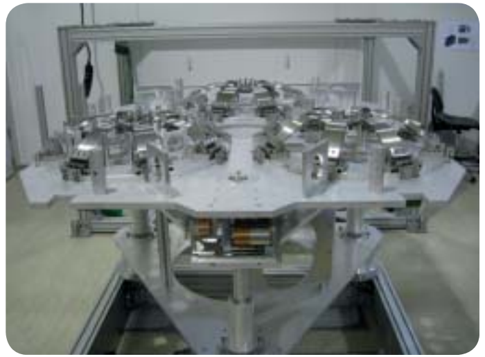
Figure 2.5.3. A seismic isolation system for optical benches. In the horizontal direction, the attenuation is done by three inverted pendula, in the vertical direction by a system of blade springs.
