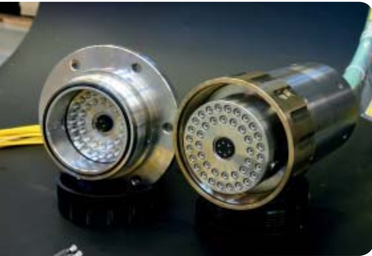
Figure 6.2.1. Optical marine cable prototype ready for pressure test at 5km below sealevel.
