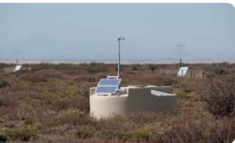
Figure 2.6.1. A particle detector in the foreground and two radio detection stations in the background.
