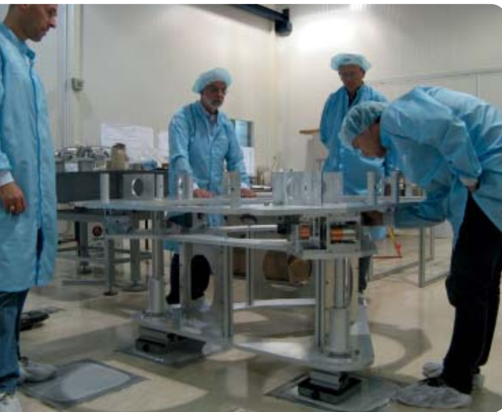
Figure 6.1.1. Assembly of the seismic attenuation system for the external injection bench of Advanced Virgo in one of Nikhef's clean rooms.
