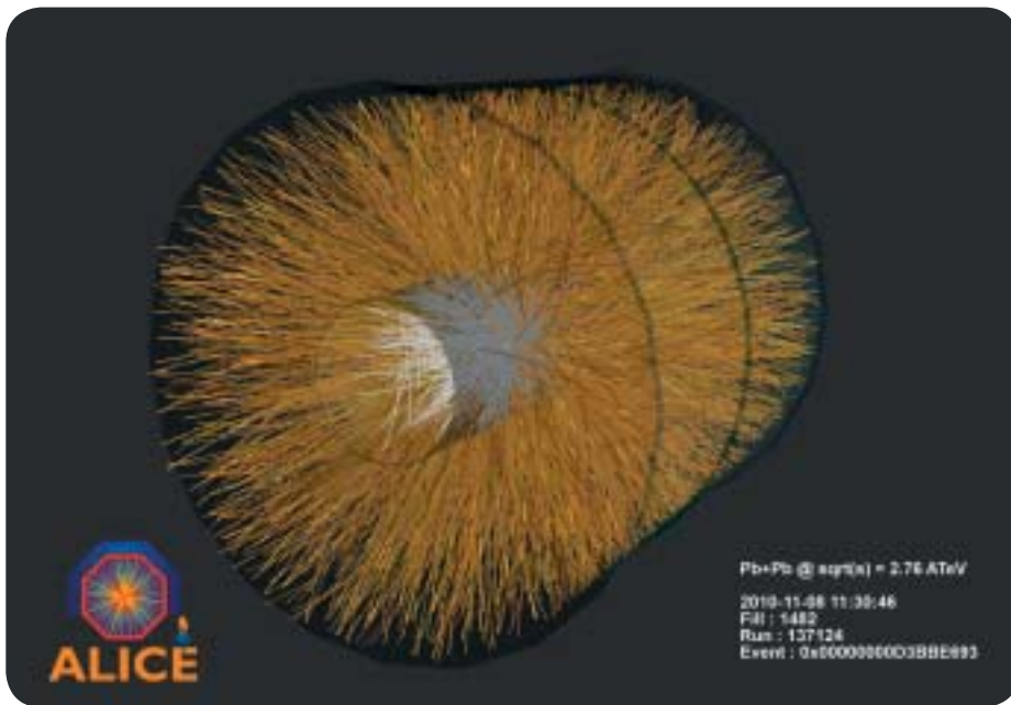
Figure 2.1.3.1. Tracks in the ALICE detector from a Pb-Pb interaction at the first heavy-ion run of the LHC in 2010.
