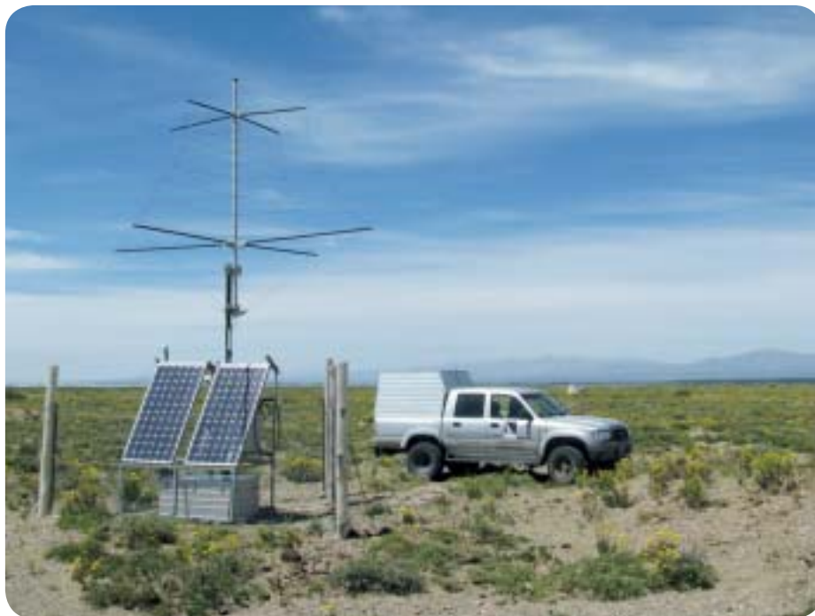
Figure 2.2.3.1. Prototype radio antenna deployed on the Pampa.
