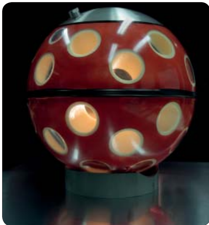
Figure 3.2.2: KM3NeT optical-module prototype –built in the Nikhef workshop– consisting of a 17 inch pressure resistant glass sphere and 31 small photo-multiplier tubes (the pressure gauge is used to measure the applied under-pressure required for water tightness of the two hemispheres at all depths).
