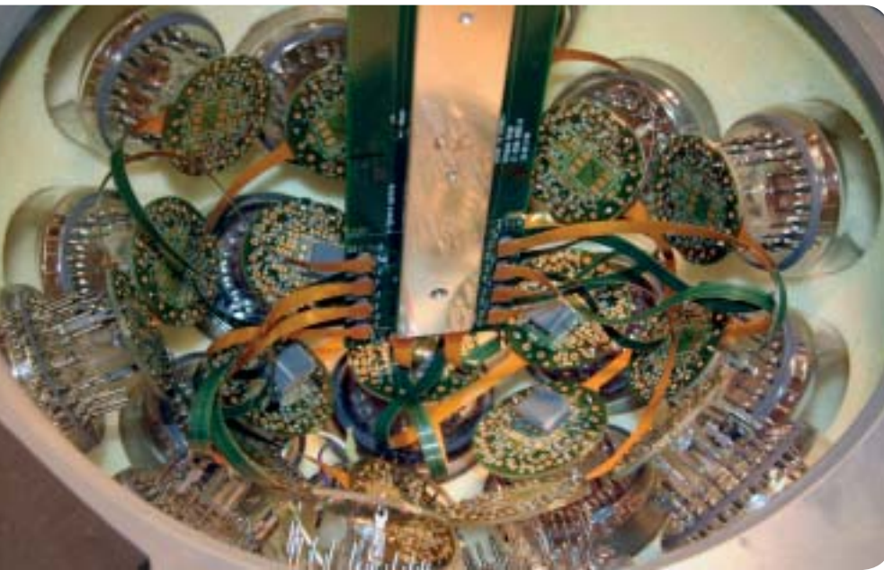
Figure 3.3.2. Bases and HV power supplies for a KM3NeT detector.
