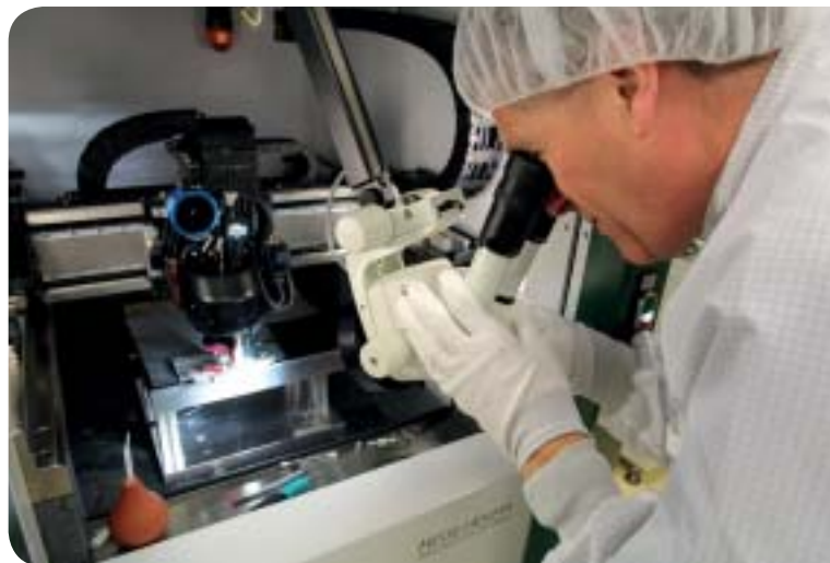
Figure 3.3.1. The automatic bonding machine, operated by Joop Rövekamp.
