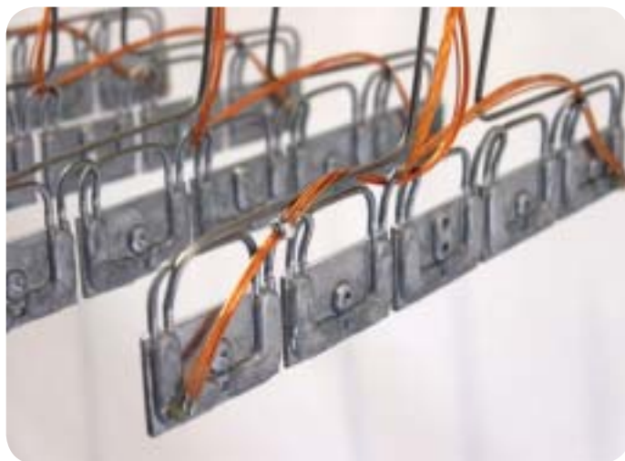
Figure 4.2.1. CO 2 evaporator cooling blocks of LHCb VELO modules with temperature sensors.
