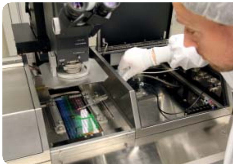
Figure 2.3.2.1. PhD student Marten Bosma, probing chips in 45 nm technology on a 300 mm wide test wafer from NXP Semiconductors.
