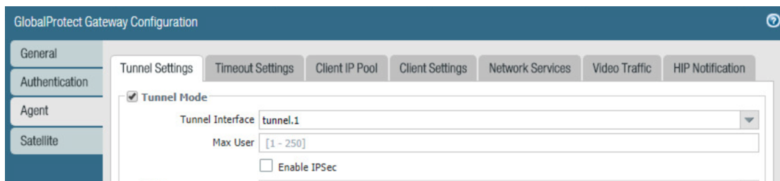
1081 Figure 2-73 GlobalProtect Tunnel Configuration
