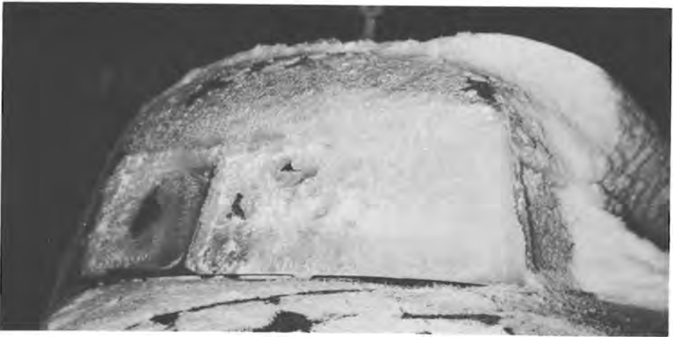
The critical need for icing research is revealed in these two photographs from the mid-1940s. Above, interior view of a B-17 windshield during flight in moderate ice conditions; the left windshield has a double-panel heated-air installation. The DC-3 pictured below had just landed at Seattle, Washington, at 3 in the afternoon. (ARC)
