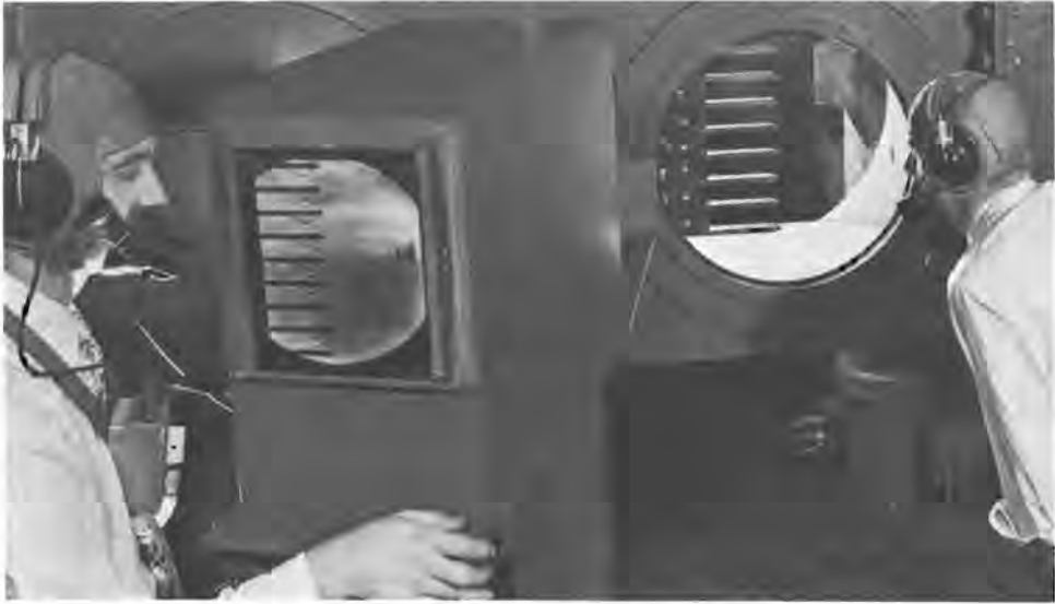
This is the kind of expensive, highly technical research for which Chairman Hunsaker and Director Dryden requested funds from President Eisenhower: a wedge rake is being used to calibrate the Lewis laboratory's 2- by 2-foot supersonic tunnel at mach 3.5. (LeRC)
