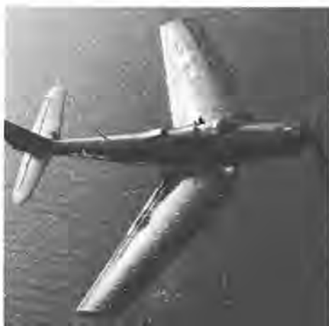
This swept-wing propeller-driven aircraft reveals the mixture of old and new that faced the NACA in 1947. The tufts of yarn on the wings reveal patterns of air-flow. (LaRC)
