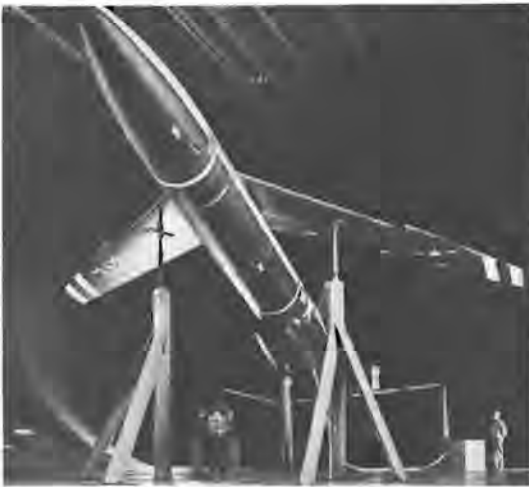
The NACA did some missile research in its wind tunnels. Here, a Northrup Snark missile stands ready for testing in the Ames full-scale wind tunnel. (ARC)
