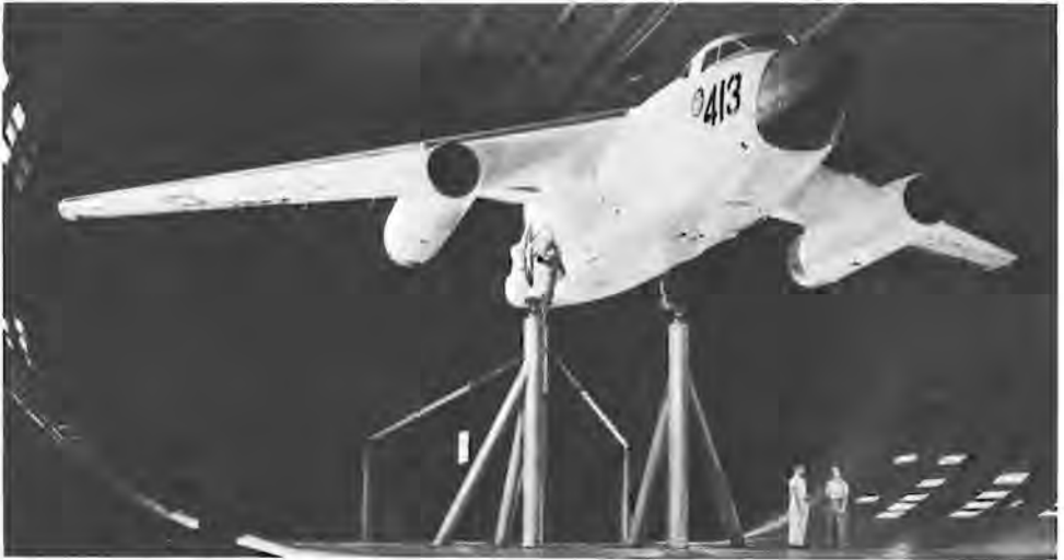
The Ames 40- by 80-foot full-scale wind tunnel could just accommodate the 72.5-foot wingspan of the Douglas A3D Skywarrior. (ARC)
