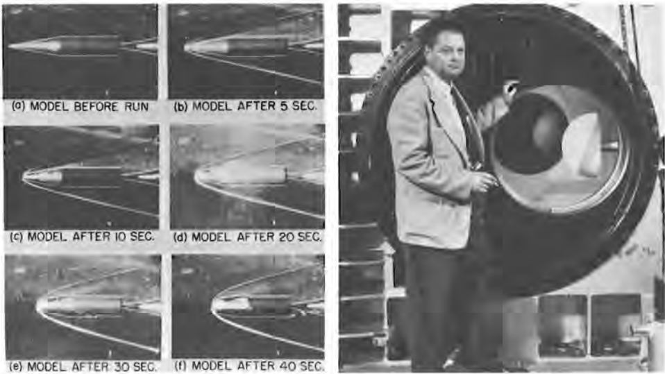
Left, a 20° cone-cylinder is melted in a wind tunnel by the friction of air passing it at 6.9 times the speed of sound, much as a similarly shaped spacecraft would melt on reentering the earth's atmosphere. (LaRC) Right, H. Julian (Harvey) Allen stands beside the test section of the Ames 8- by 7-foot unitary plan wind tunnel, in which is mounted a test model of the blunt-body concept he pioneered to counteract this heating problem in reentry vehicles. (ARC)
