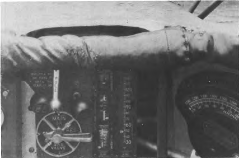
The primitiveness of early NACA research is shown in these two 1921 photographs. Above, a model helicopter rotor is tested in Langley's wind tunnel #1, an exception to the NACA pattern of ignoring helicopter research before World War II. Below, a cockpit is equipped with a new airspeed indicator (next to the empty space on the right side of the panel) to aid flight research. (LaRC)
