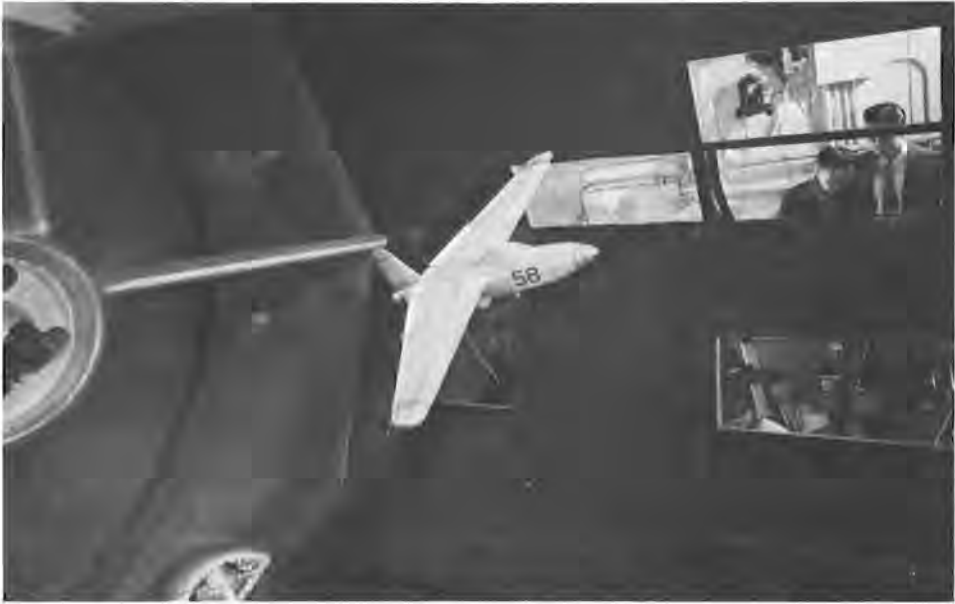
Among the unique facilities of the NACA was Langley's free-flight wind tunnel. In this 1946 test of a fighter model with forward-swept wings, the "pilot" at lower left maneuvers the model while the tunnel operators keep watch at right. (LaRC)
