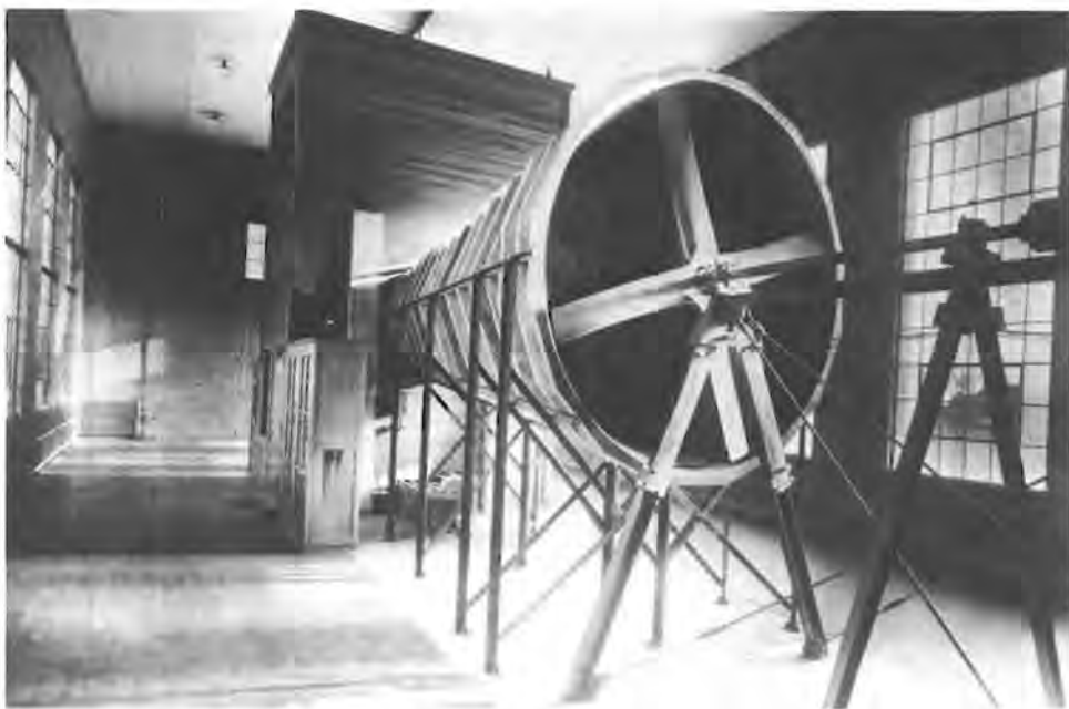
Langley laboratory's wind tunnel #1, shown here in about 1921, was part of the very modest facilities with which the NACA began its career in aeronautical research. (LaRC)
