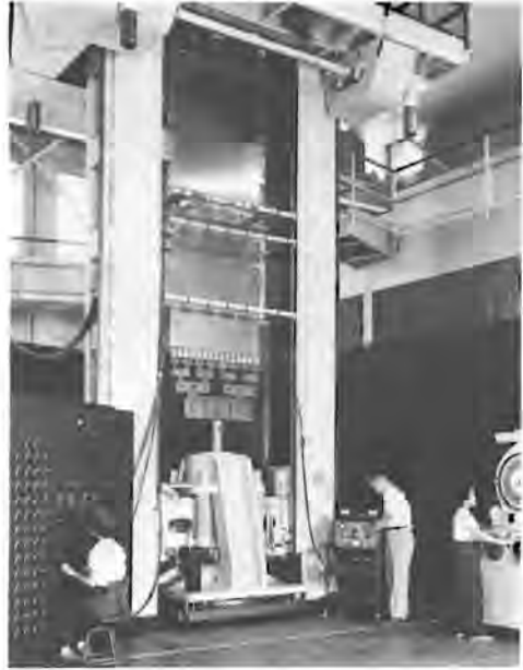
Not all NACA research was conducted in wind tunnels. This million-pound testing machine was used at the Langley laboratory for structures research. (LaRC)
