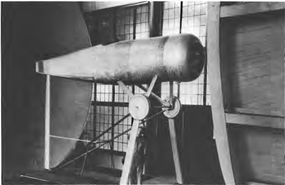
An aircraft fuselage with a NACA cowling is installed in the propeller-research tunnel at Langley laboratory, 1929. (LaRC)
