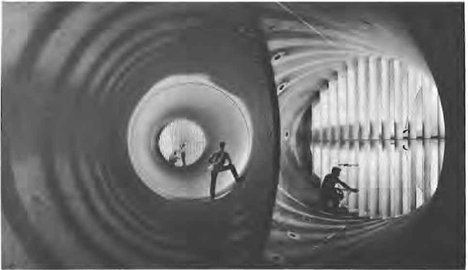
The unitary plan supersonic wind tunnel at the Langley laboratory had two test sections; the exit passages joined at this irregularly shaped section of the tunnel. Technicians in both passages are working on the guide vanes. (LaRC)
