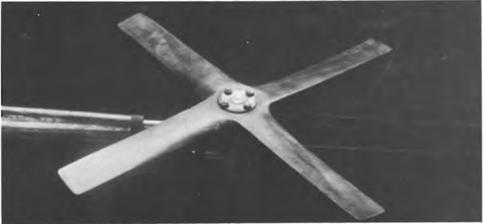
The primitiveness of early NACA research is shown in these two 1921 photographs. Above, a model helicopter rotor is tested in Langley's wind tunnel #1, an exception to the NACA pattern of ignoring helicopter research before World War II. Below, a cockpit is equipped with a new airspeed indicator (next to the empty space on the right side of the panel) to aid flight research. (LaRC)
