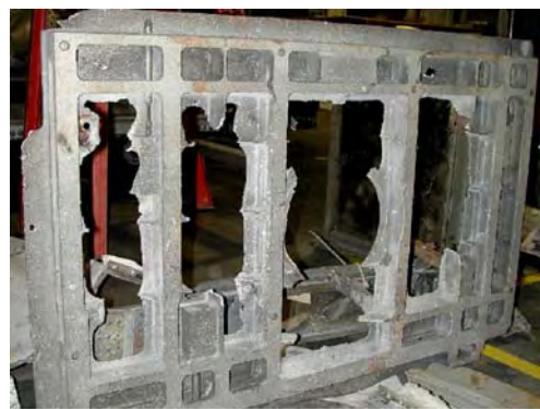
Figure 2.1-38. Lower surface of the recovered lithium hydroxide door, facing the lower equipment bay.
