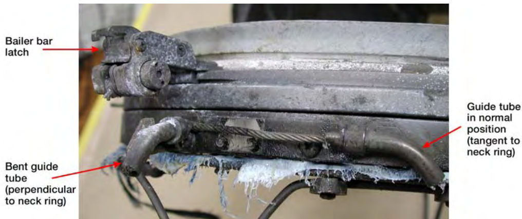
Figure 3.2-24. Hold-down cable guide tube.
