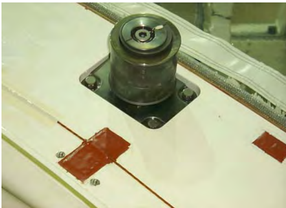
Figure 2.1-52. Payload bay door roller showing inner material and Inconel sleeve.
