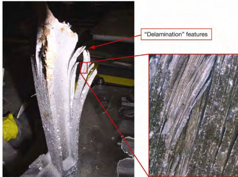
Figure 3.1-16. Example of a “broom-straw” fracture on a Columbia seat leg.
