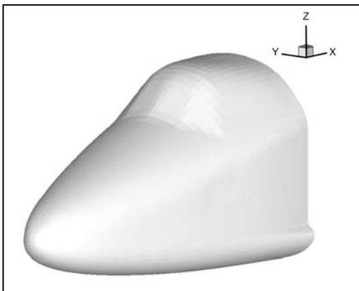
Figure 4-8. Forward fuselage/crew module (forebody) configuration.
