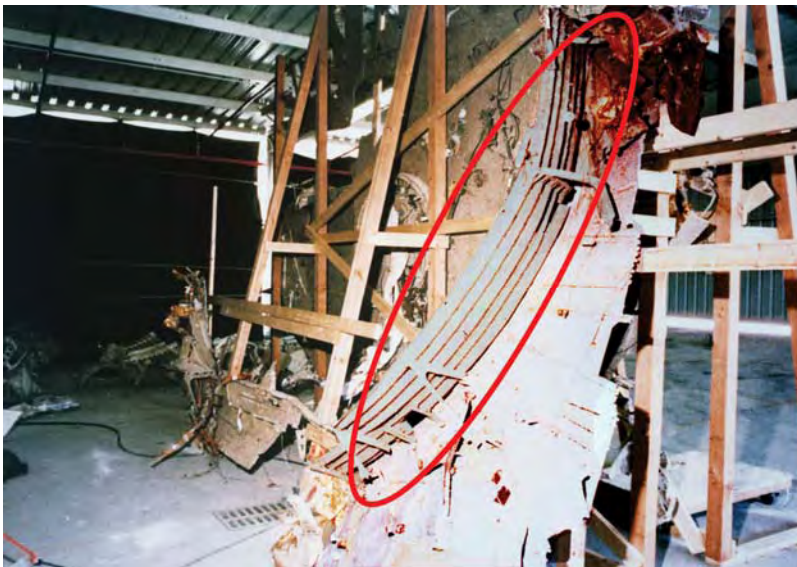
Figure 2.2-30. Recovered X o 576 bulkhead of the Challenger crew module showing a portion of the X o 582 ring frame bulkhead (circled in red).
