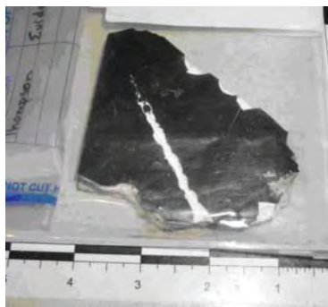
Figure 1.1-16. The Littlefield tile. [Picture from the Columbia Reconstruction Database, debris item no. 14768]
