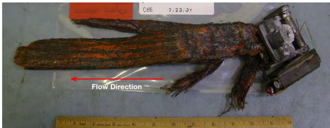
Figure 3.2-31. Directional melting on Seawater Activated Release System/parachute harness strap.
