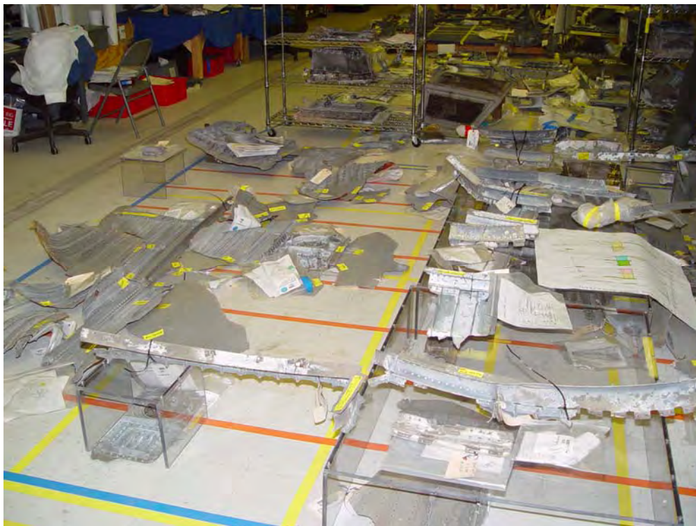
Figure 2.4-40. Lower forward fuselage skin and frame debris.
