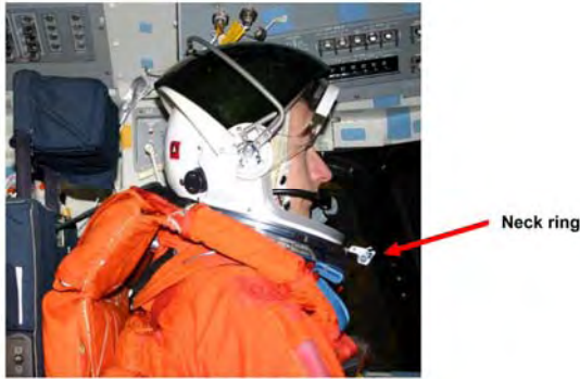
Figure 3.4-18. Demonstration of an integrated seat/suit/crew member in entry configuration.
