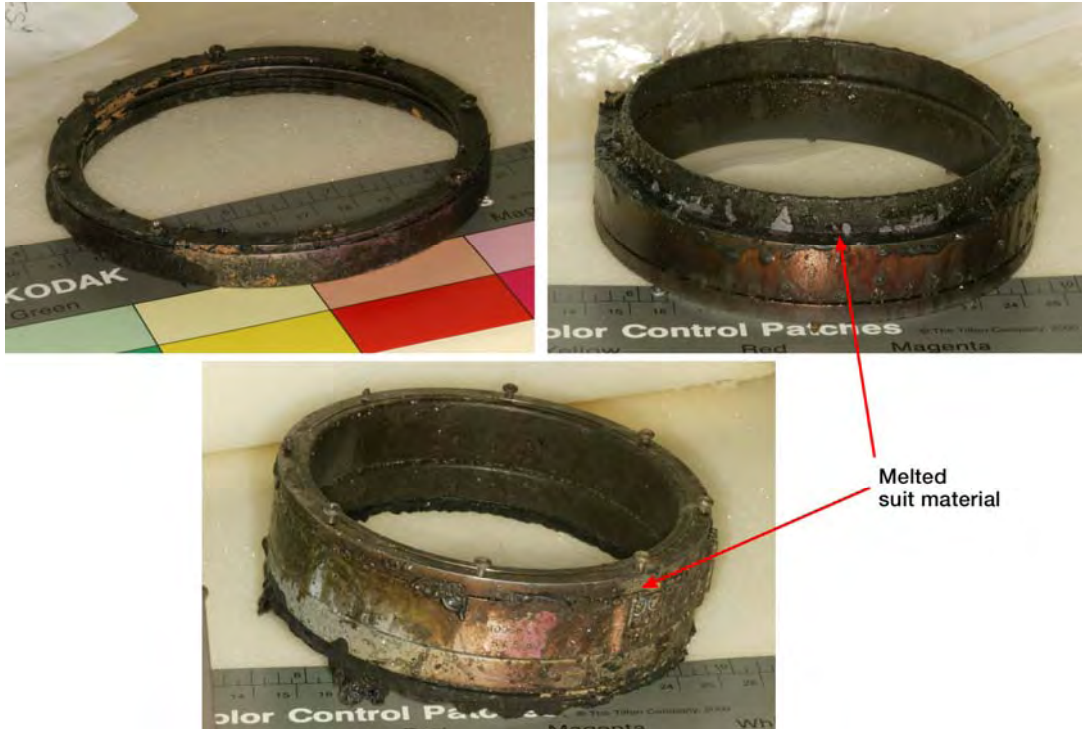
Figure 3.2-26. Recovered suit-side (upper left), glove-side (upper right), and mated (bottom) glove disconnects.
