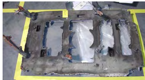
Figure 2.1-36. Top surface of the recovered lithium hydroxide door, facing the middeck.
