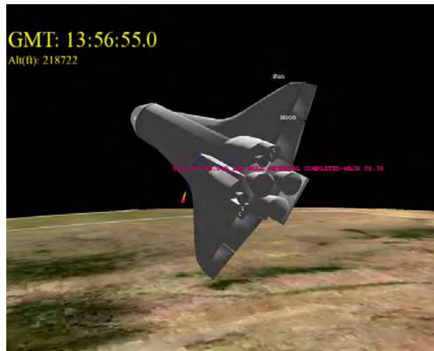
Figure 1.2-30. Attitude at the completion of the roll reversal.
