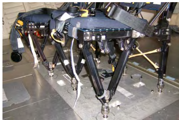
Figure 2.1-34. Example of an intact lithium hydroxide door with seats 6 and 7 attached. [Crew Compartment Trainer]
