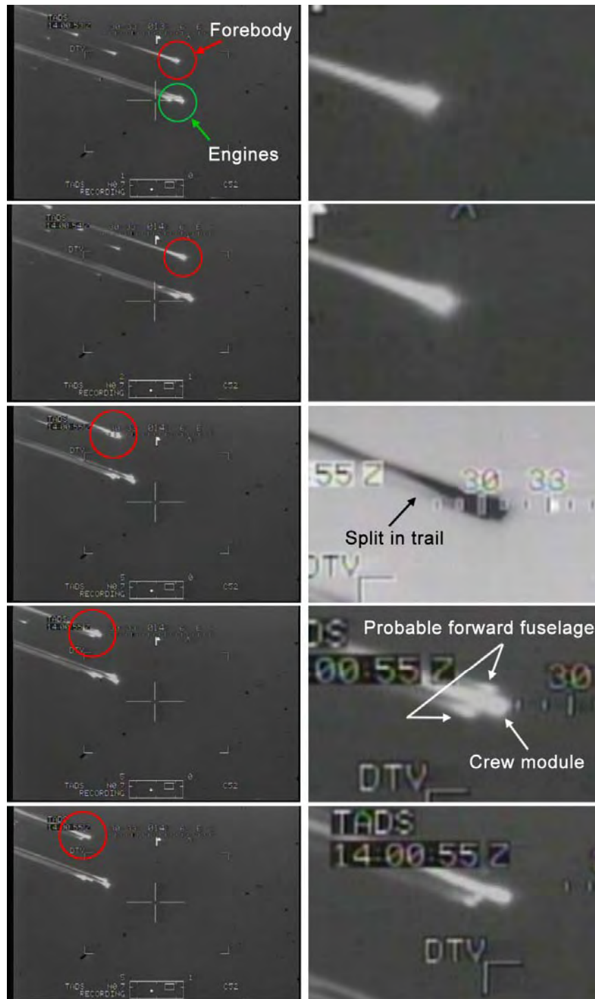
Figure 2.4-1. Five time-paired images covering under 2 seconds of time showing the Crew Module Catastrophic Event. Image on the left is the full frame, image on the right is an enlarged view.
