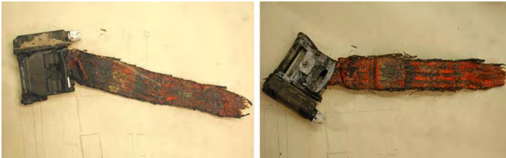
Figure 3.2-30. Seawater Activated Release System with Frost fittings (male/female) still mated, with a segment of harness strap attached (two different SEAWARS are shown).
