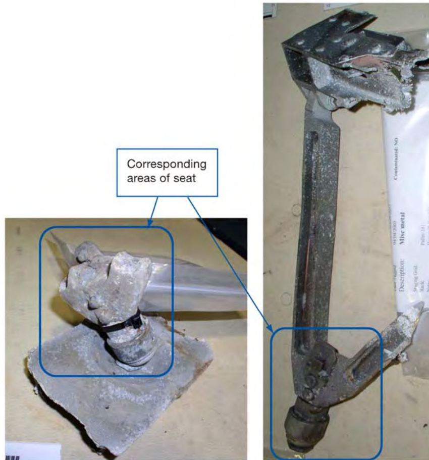
Figure 3.1-10. Comparison of seat debris from a flight deck Mission Specialist seat (left) and a middeck Mission Specialist seat (right).
