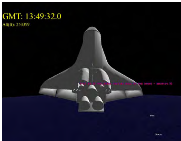
Figure 1.2-17. Attitude of Columbia at the start of the first planned roll.
