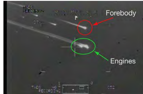
Figure 2.2-10. Clear visual separation of the three main engines.
