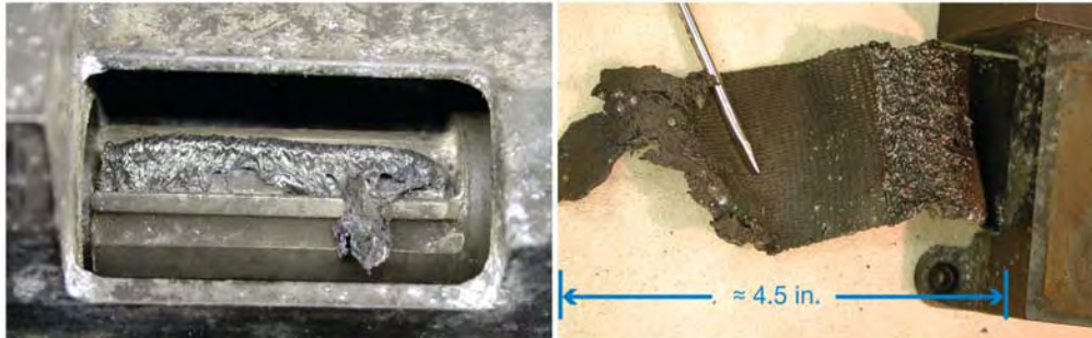
Figure 3.1-26. Seat strap failures: seat 1 (left) and seat 2 (right).
