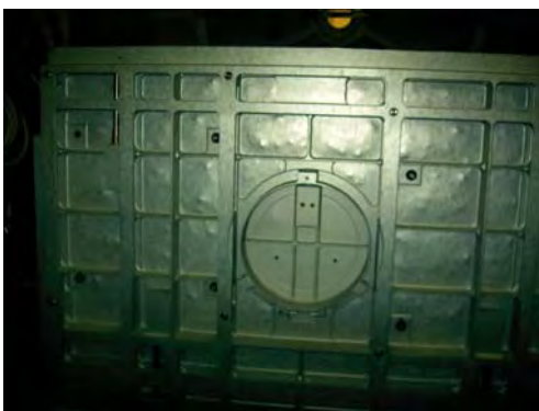
Figure 2.1-37. Lower surface of the lithium hydroxide door, facing the lower equipment bay (mockup).
