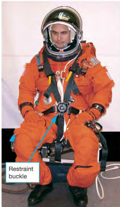
Figure 3.1-39. Demonstration of the five-point seatbelt buckle.
