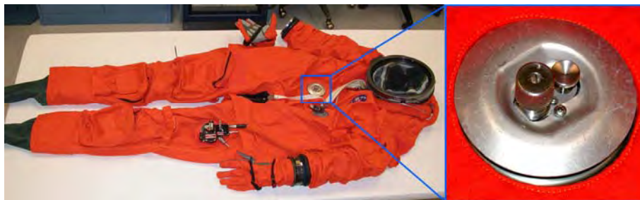
Figure 3.2-27. Example of an intact dual suit controller.
