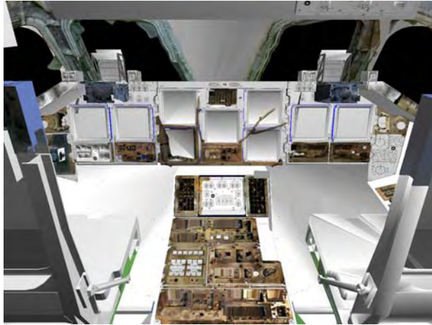
Figure 2.4-56. Virtual reconstruction of the recovered Columbia flight deck panels.
