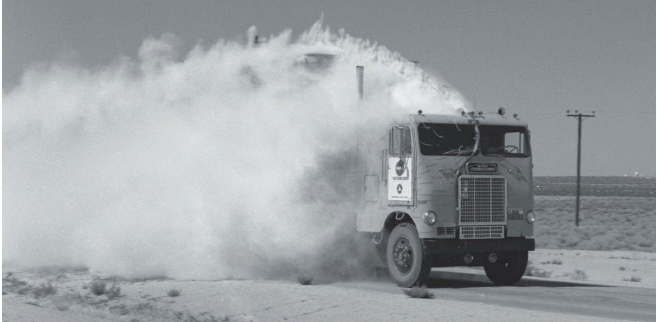
The NASA tractor-trailer carrying various aftermarket devices in a test for the Department of Transportation. Diatomaceous earth is blown through a tube up the cab's front and released between the three running lights at the cab's leading edge, revealing airflow for each device. The cab has also been tufted to show airflow around it while in motion. The bottom image shows the cab with a valance, applied by the FRC and unavailable as an aftermarket item.
