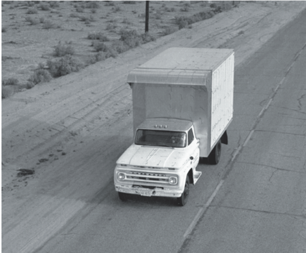
This image reveals the gap at the top of the flow vane, which resembled a fixed leading-edge wing slat. NASA E75-28964
