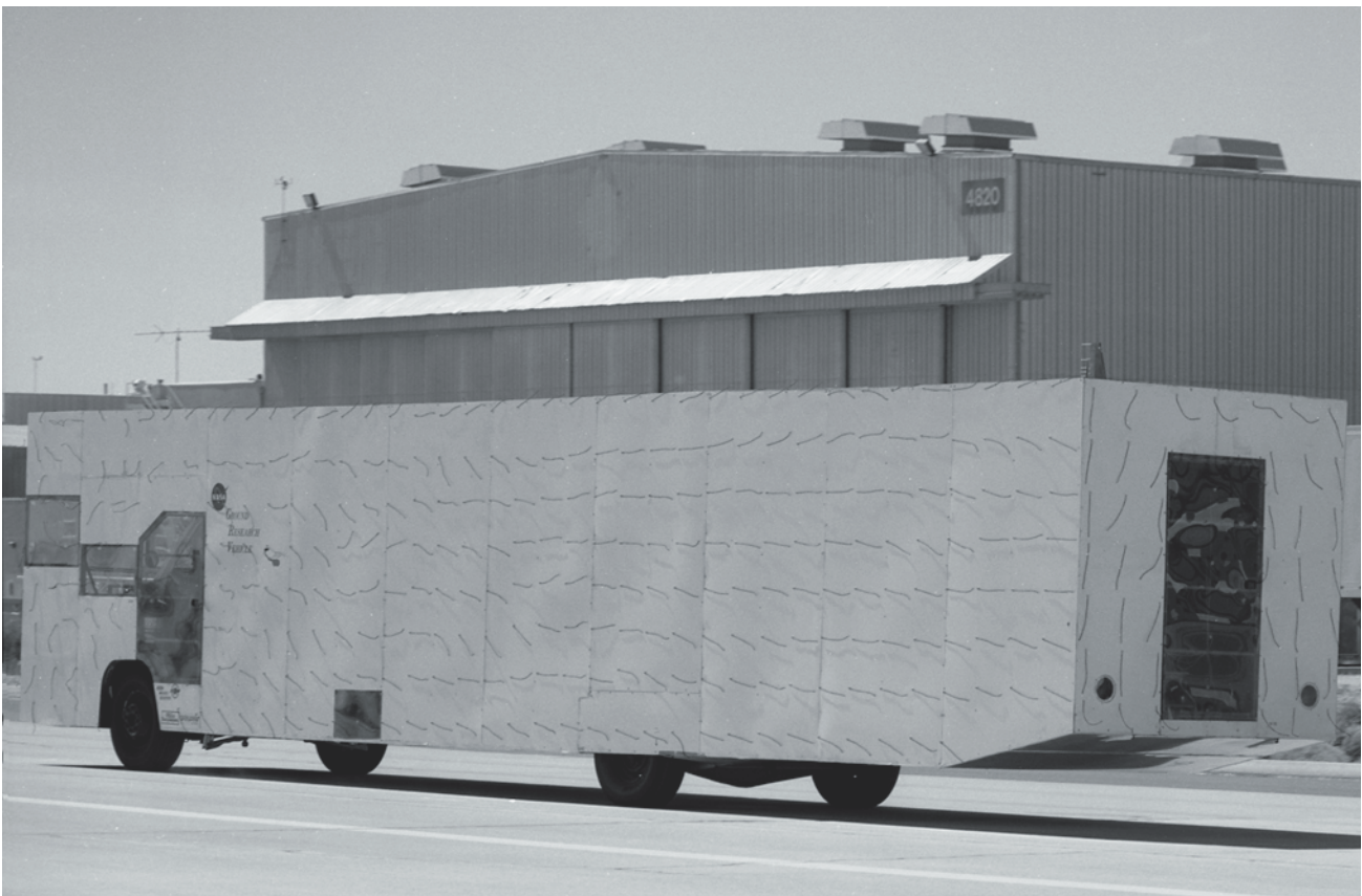
Above and below, the Ground Research Vehicle (Roadrunner) during runs on the NASA Dryden flight line. Tufts of yarn show chaotic airflow over the vehicle's first half but fairly smooth and controlled airflow over the latter half. A rake, used to measure boundary layers, stands above the roofline at the vehicle's aft end.
