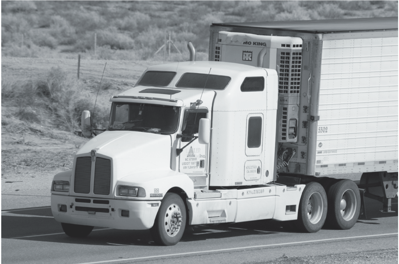
A Kenworth T600 pulling a refrigerated trailer. The chiller is mounted on the nose. NASA
