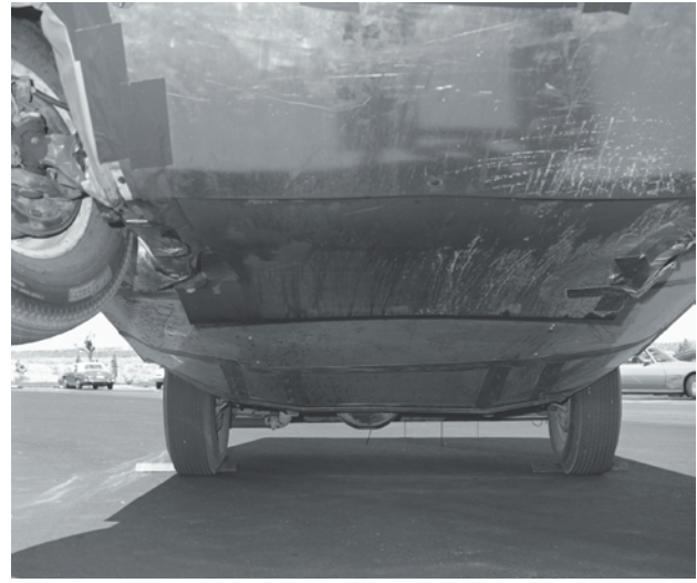
The image at left shows the underbody of the Shoebox in its stock configuration. The image at right shows the same underside after it had been sealed. This modification alone, including sealing the wheel wells, reduced aerodynamic drag by 15 percent.
