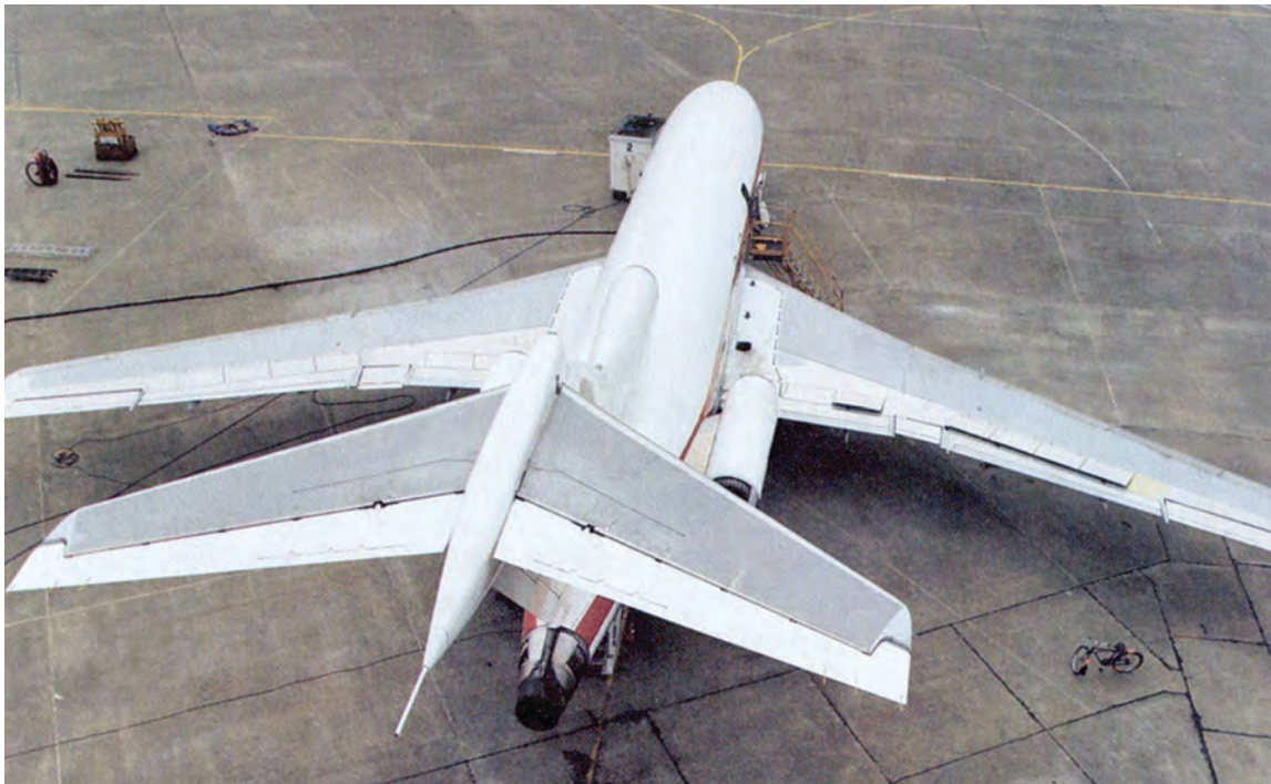
Composite elevators in flight evaluations on Boeing 727 during ACEE Program.
