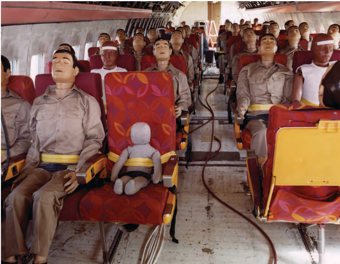
Instrumented dummies in Boeing 720 for CID test.
