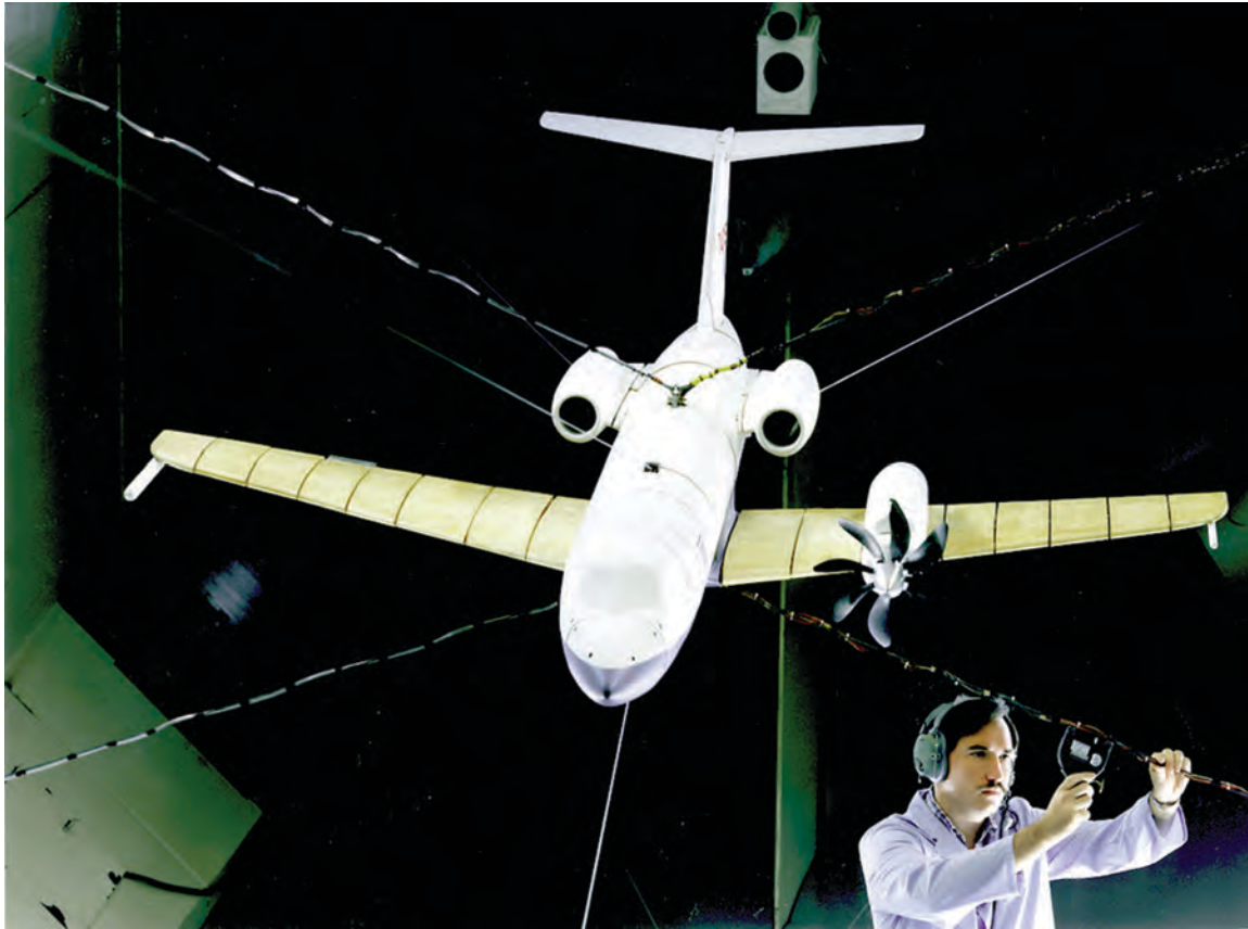
Propeller Test Assessment configuration in TDT with Langley's Michael Durham.
