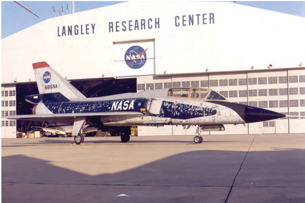
F-106B (NASA 816) research aircraft during Storm Hazards Program in 1982. Note paint spots applied to aircraft that denote lightning attachment points.
