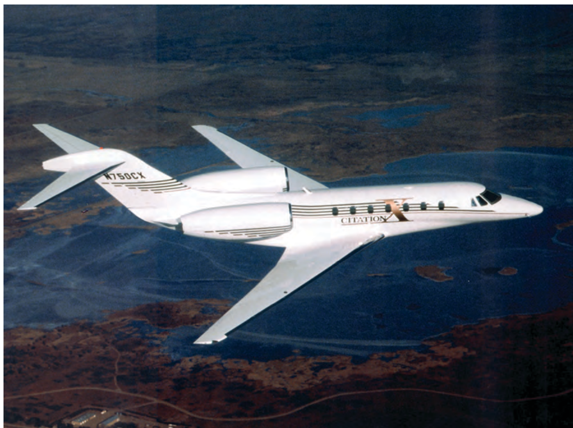
Cessna Citation, a current T-tail aircraft, designed to avoid potential for deep stall.
