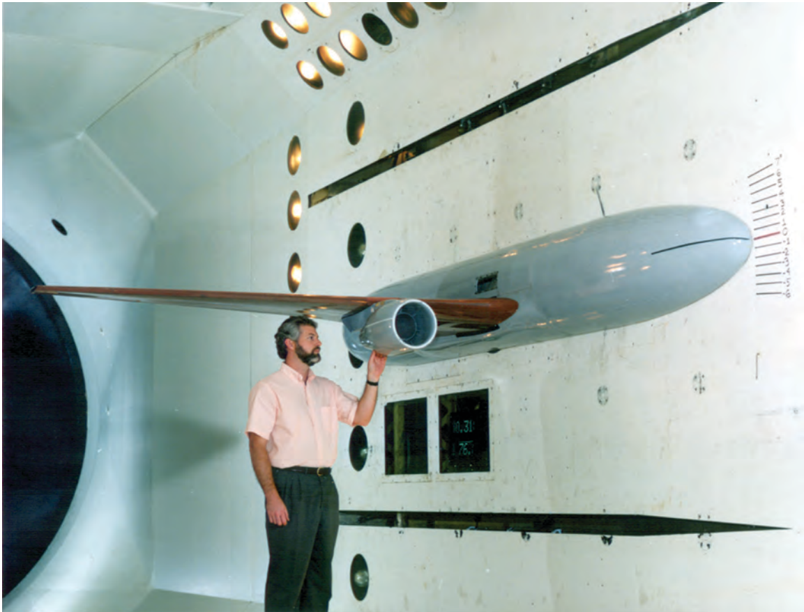
Stanley Cole with representative Boeing 767 model mounted for general research on limit cycle oscillations in TDT.
