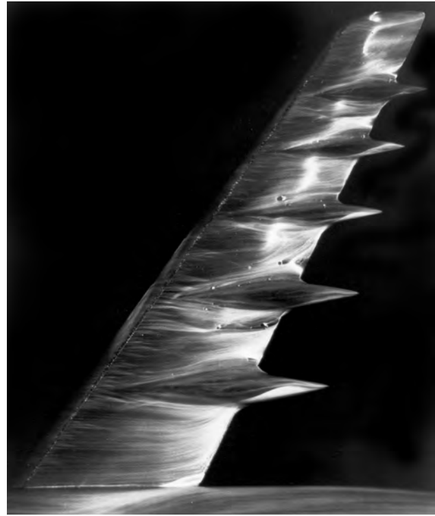
Oil flow visualization of model wing with 35° sweepback at Mach number of 0.90 and angle of attack of 4° (flow is left to right). A significant amount of unacceptable flow separation is evident for basic wing (left) on rearward part of wing; the addition of antishock bodies (right) greatly reduces separation.
