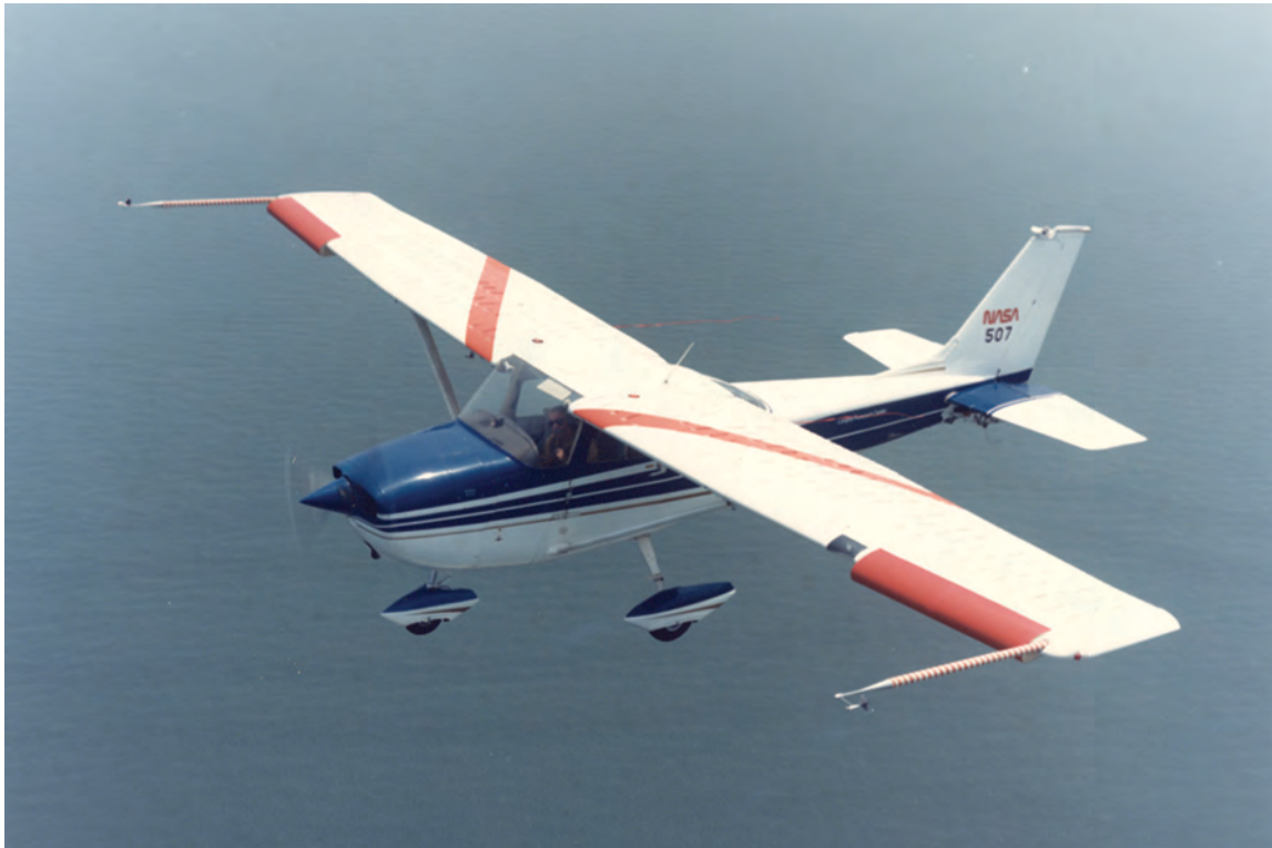
Cessna 172 research aircraft with outer wing leading-edge-droop modification.
