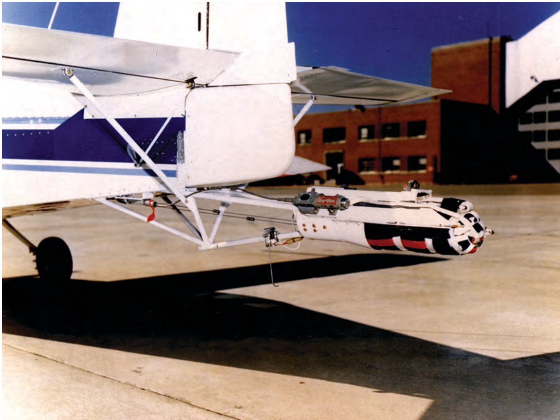
Pyrotechnically deployed spin parachute developed in Langley program.
