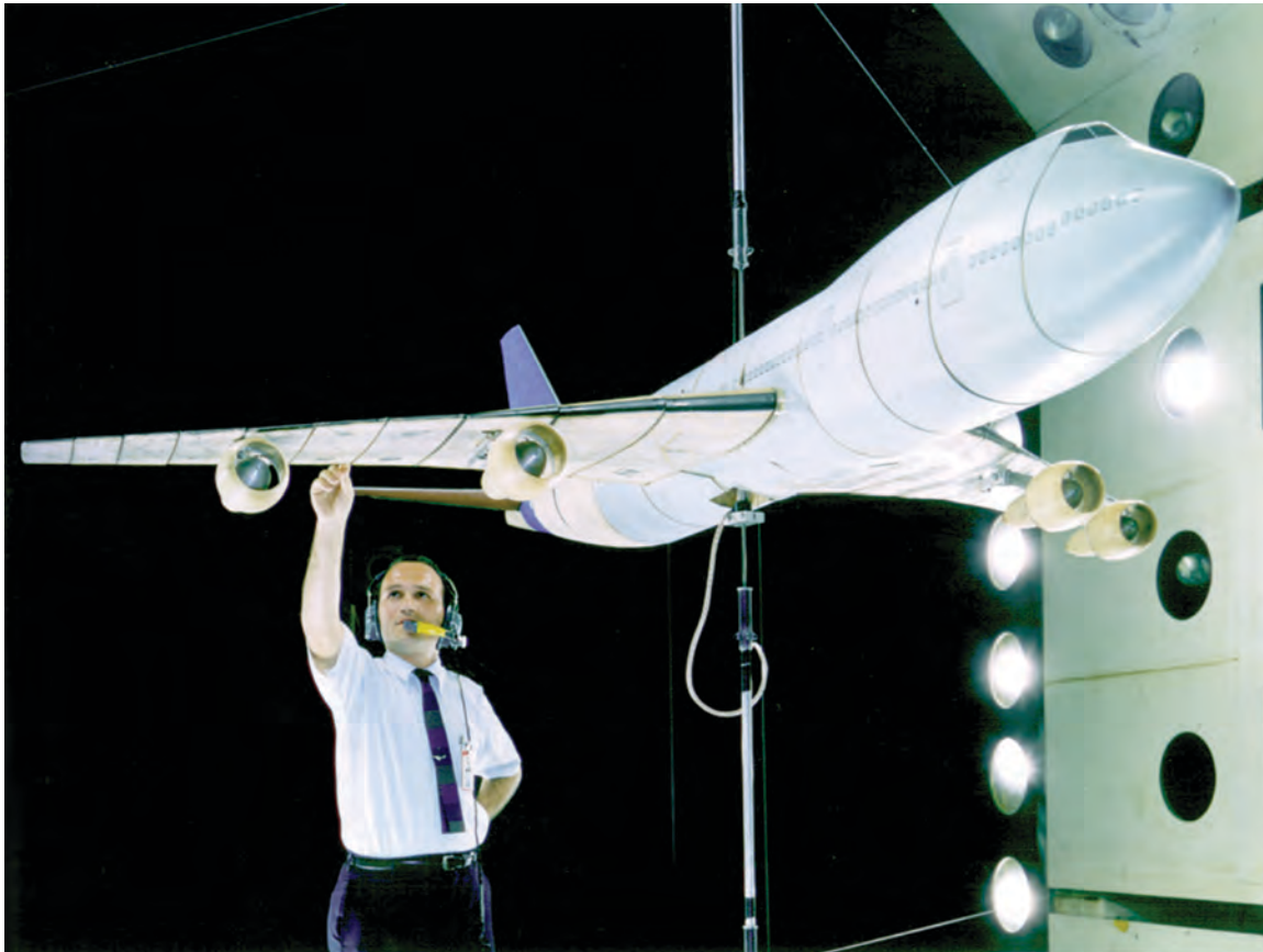
Researcher Irving Abel with Boeing 747 flutter model.
