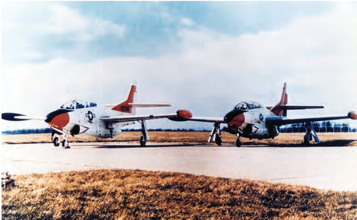
Basic T-2 (left) and modified T-2 with 17-percent-thick supercritical wing (right).
