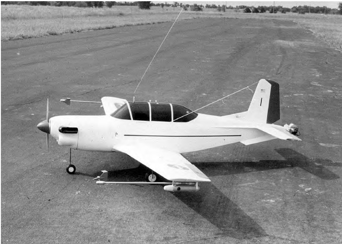
Radio-controlled model of YT-34C aircraft used in Beech study of spin characteristics.
