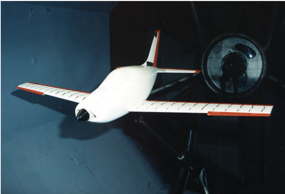
Model of Questair Venture aircraft in Langley 12-Foot Low-Speed Tunnel during tests to develop spin-resistant wing configuration.
