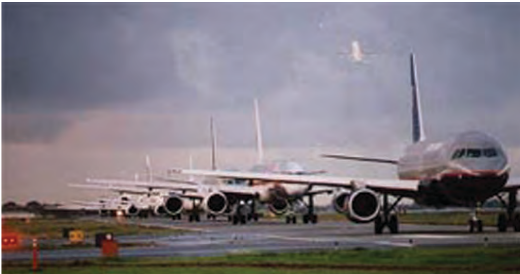
Wake-vortex separation requirements under instrument flight rules conditions aggravate airport capacity problem.
