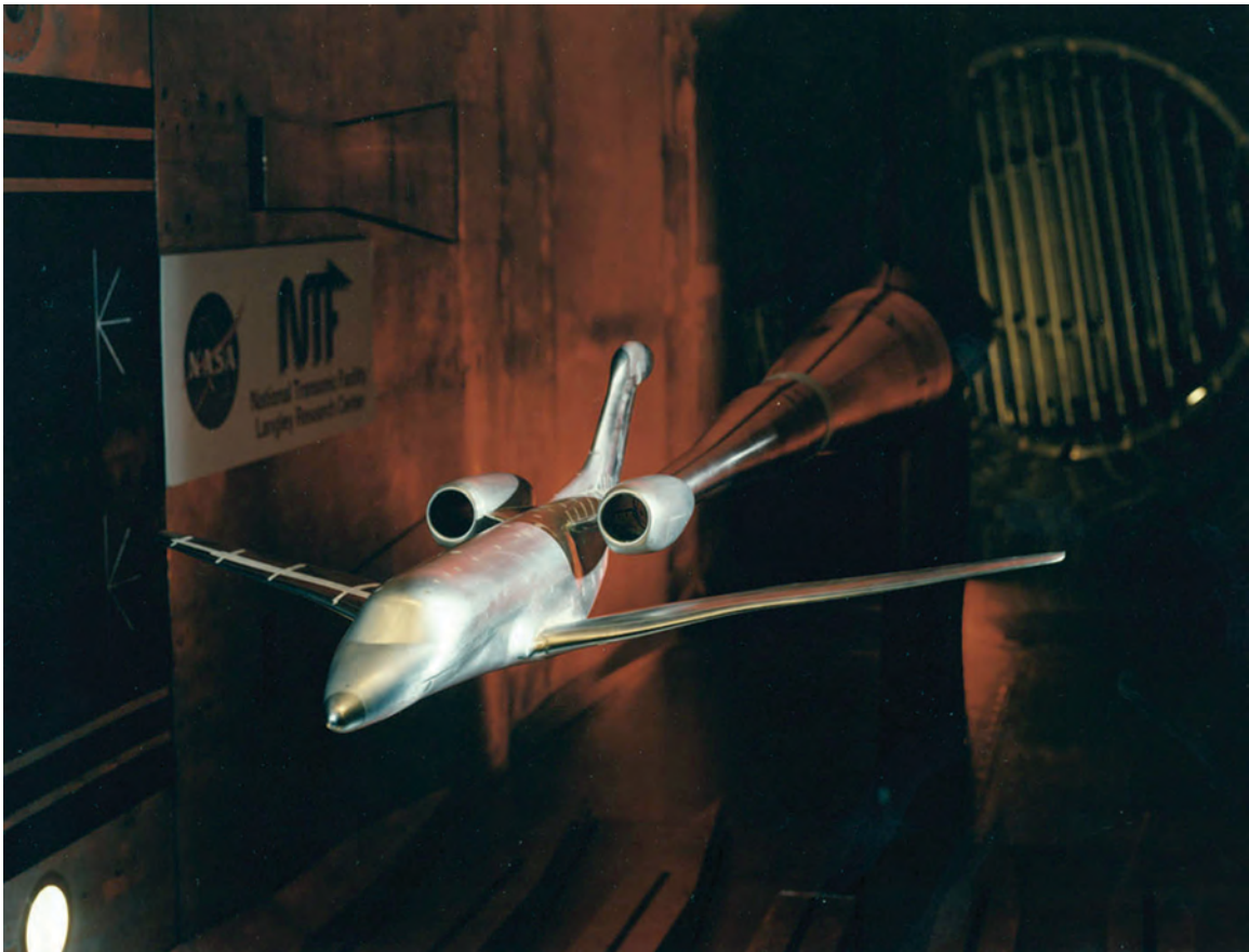
Cooperative Langley and Cessna tests of multipoint wing design for Citation X in National Transonic Facility.
