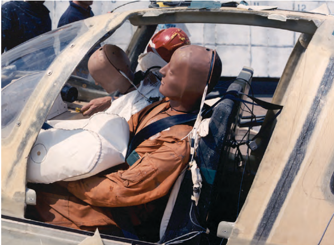
Postcrash photograph of dummies used in IDRF testing.
