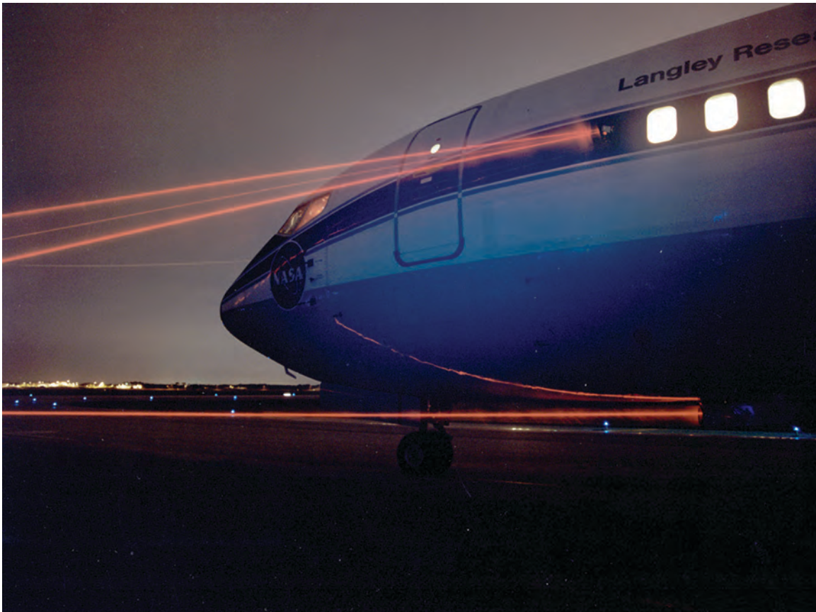
Laser beams used to align lidar and infrared detection systems on TSRV.
