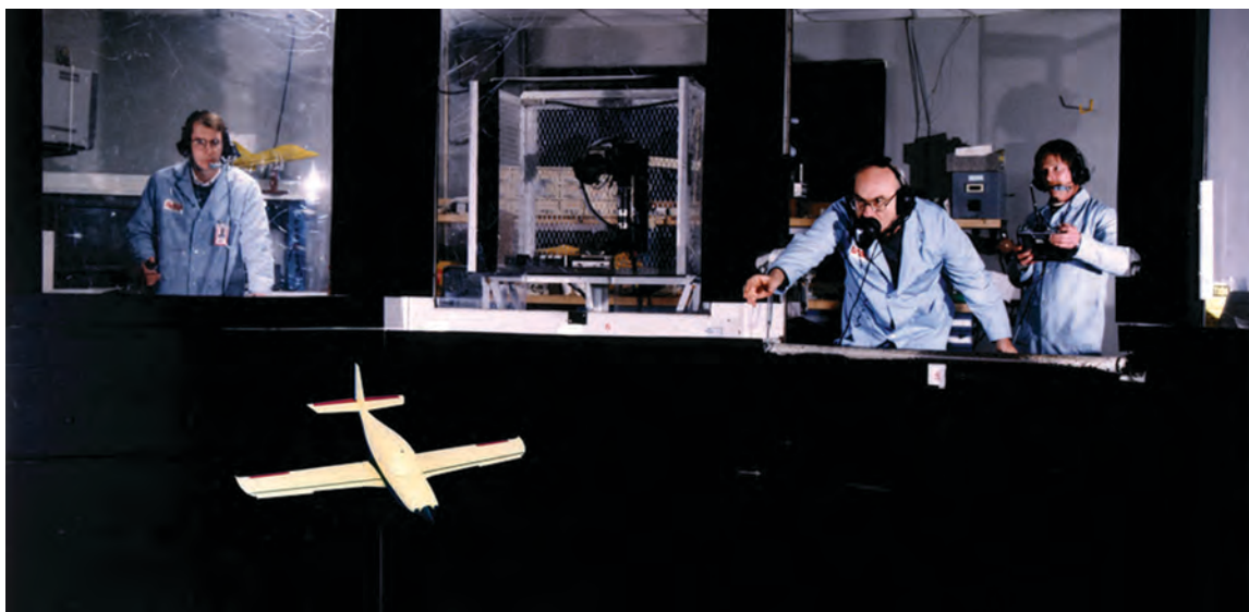
Researcher Charles Fremaux (left) and technicians Ronald Hermansderfer and James Hassell conduct tests of Columbia 300 model. Note auxiliary leading-edge flaps on wings for correction of Reynolds number effects.
