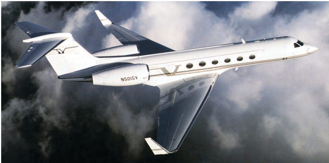
Record-setting Gulfstream V with supercritical airfoil sections for its winglet design.
