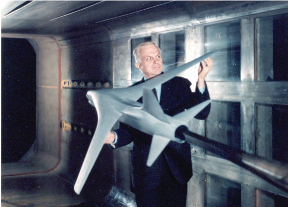
Richard T. Whitcomb with model of F-8 supercritical wing configuration in Langley 8-Foot Transonic Pressure Tunnel.
