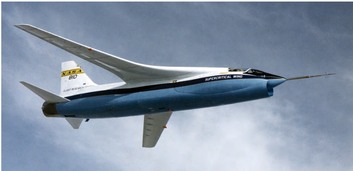
F-8 supercritical wing test-bed aircraft in flight with an area-ruled fuselage and underwing leading-edge vortex generators.
