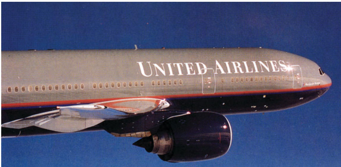
In-flight photograph of Boeing 777 shows lower wing trailing-edge curvature associated with supercritical airfoils.
