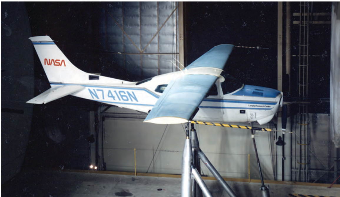
Following highly successful flight test program, Centurion was tested in Langley 30- by 60-Foot Tunnel in 1985.
