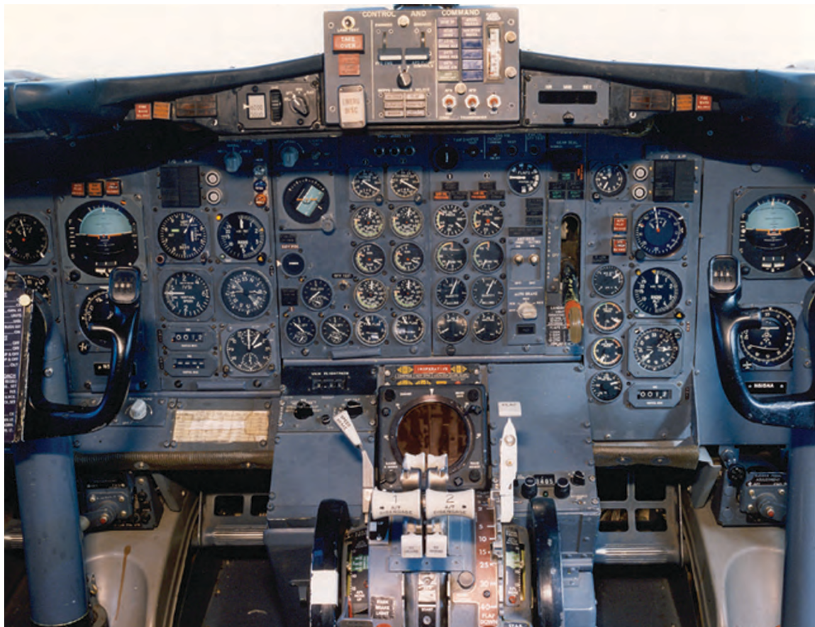
TSRV forward cockpit display in original layout. Note electromechanical gauges and dials; control and command panel added on glare shield to engage and transfer control to and from aft research flight deck.
