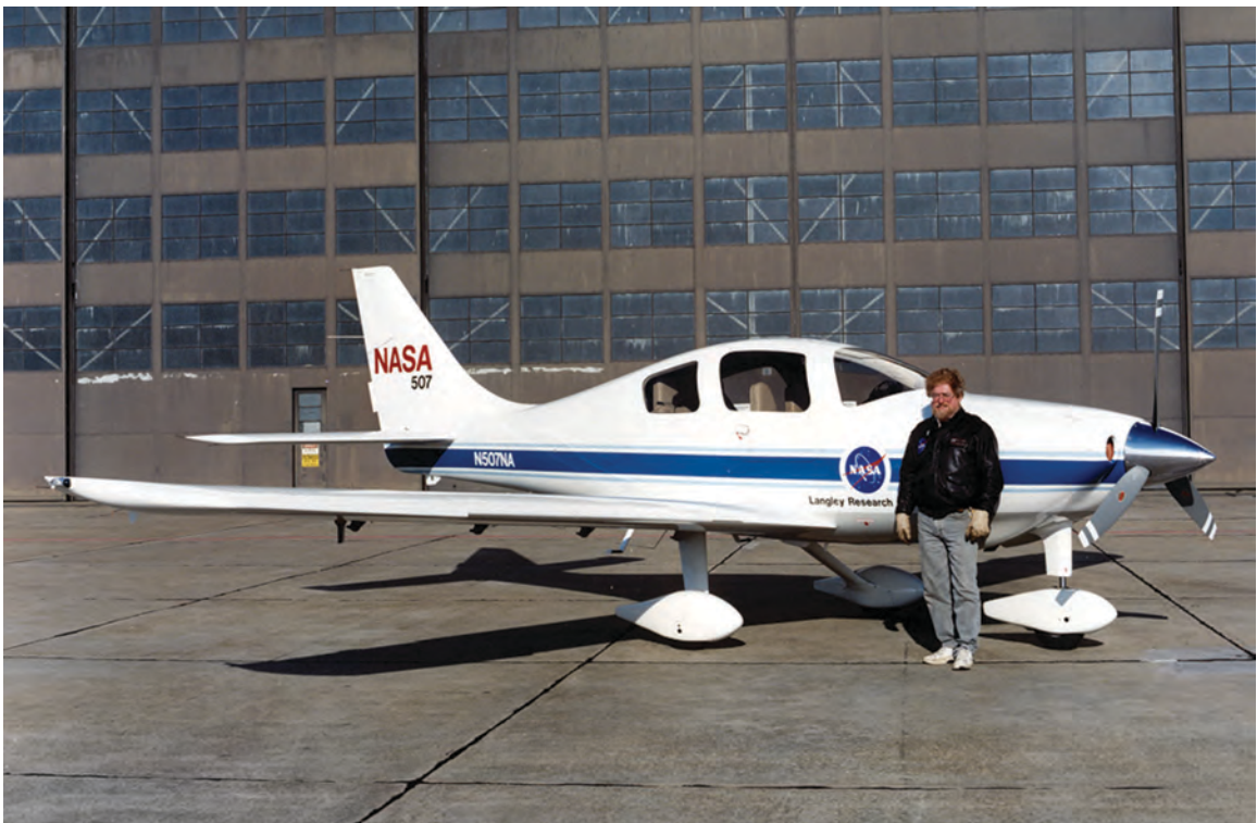
NASA Lancair 300 research aircraft with outboard leading-edge droop.
