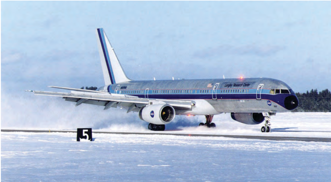
Langley's Boeing 757 aircraft during test run at joint runway friction testing at Kenneth Ingle Sawyer Air Base at Gwinn, Michigan, February 1999.
