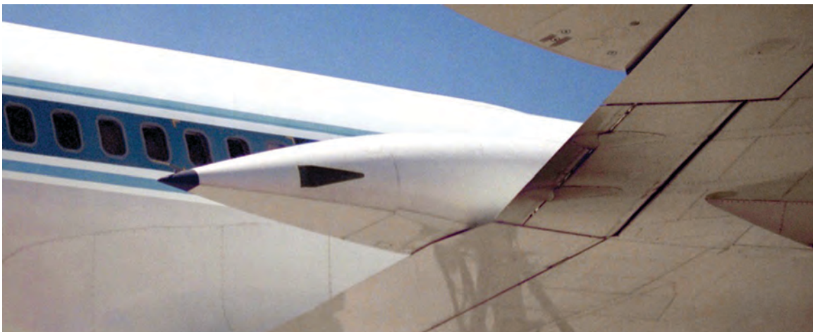
View from beneath Convair 990 showing flattened lower surface of semiconical antishock bodies.
