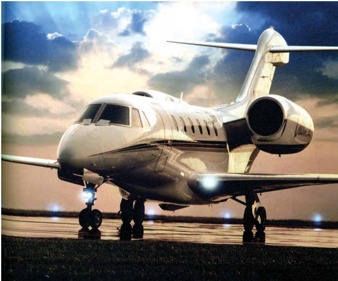
Cessna Citation X with local area-ruled features incorporated in its lower and aft-fuselage shapes.
