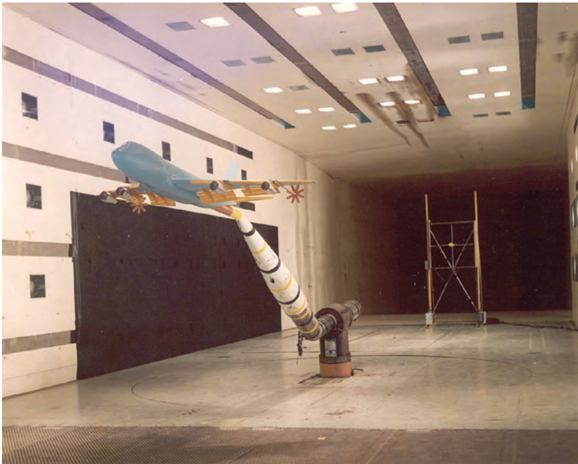
Model of Boeing 747 during wake-vortex testing in Langley 14- by 22-Foot Tunnel with traversing rig mounted downstream to permit measurements of trailing wake.
