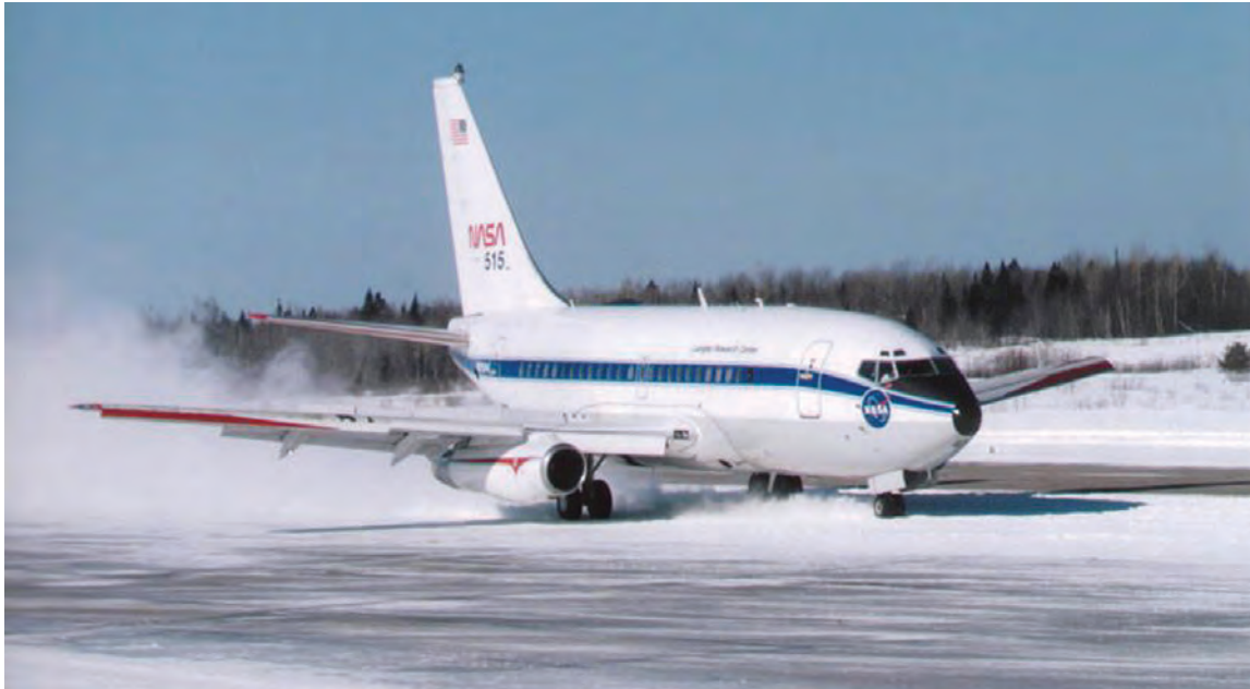
Langley's Boeing 737 research aircraft during winter runway friction studies.
