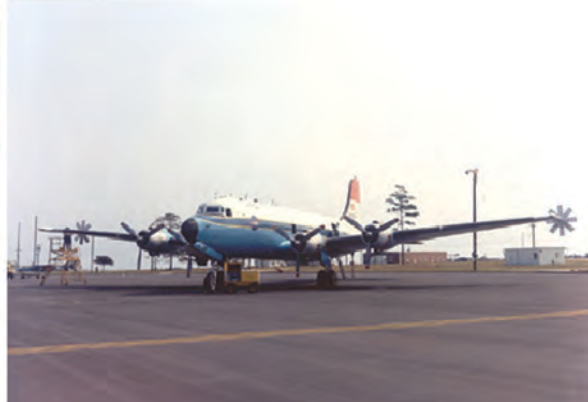
Langley's evaluation of spline device on C-54. Top photographs show VRF results for basic (left) and modified model, showing diffuse wake with spline. Lower photographs show installation of splines on full-scale aircraft.
