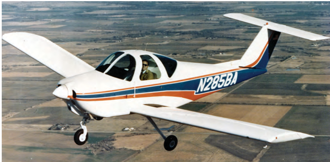
Beechcraft Model 77 Skipper, one of first industry applications of radio-controlled model test technique for spin studies.
