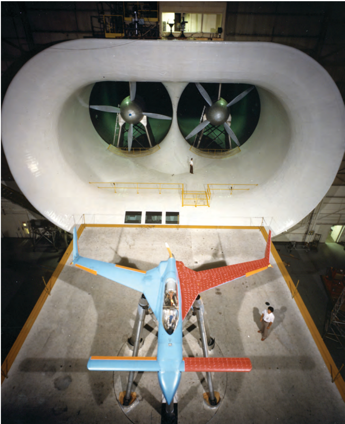
Long Yip with full-scale model of Rutan VariEze aircraft in Langley 30- by 60-Foot Tunnel. Note outer wing extended leading-edge-droop modifications on aft main wing.
