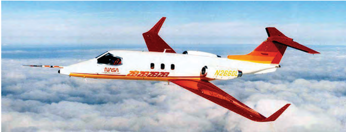
Learjet Model 28/29, first production jet aircraft to utilize winglets.
