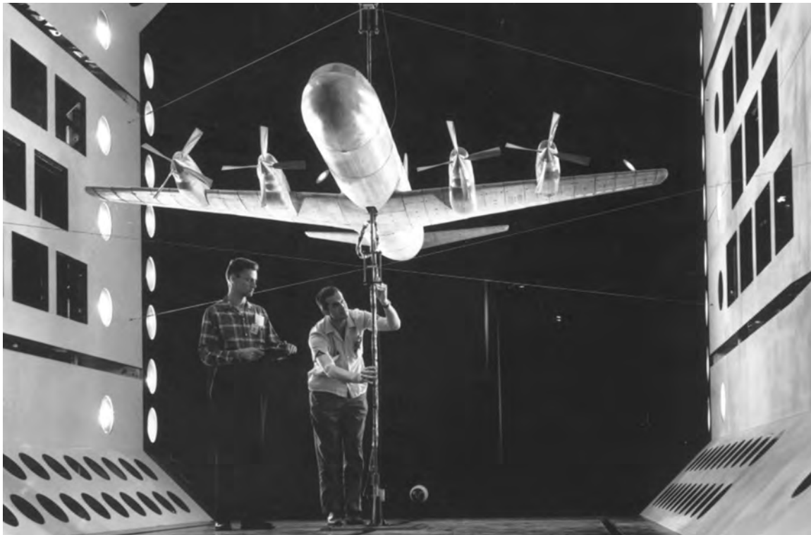
Powered model of Lockheed Electra mounted in Langley Transonic Dynamics Tunnel for flutter tests.
