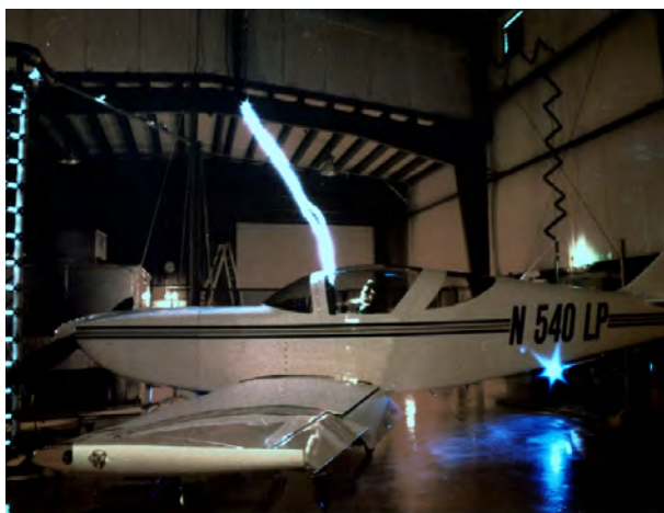
Prototype of Glasair III LP manufactured by Stoddard-Hamilton Aircraft, Inc., undergoing direct-effect testing at LTI's laboratory.
