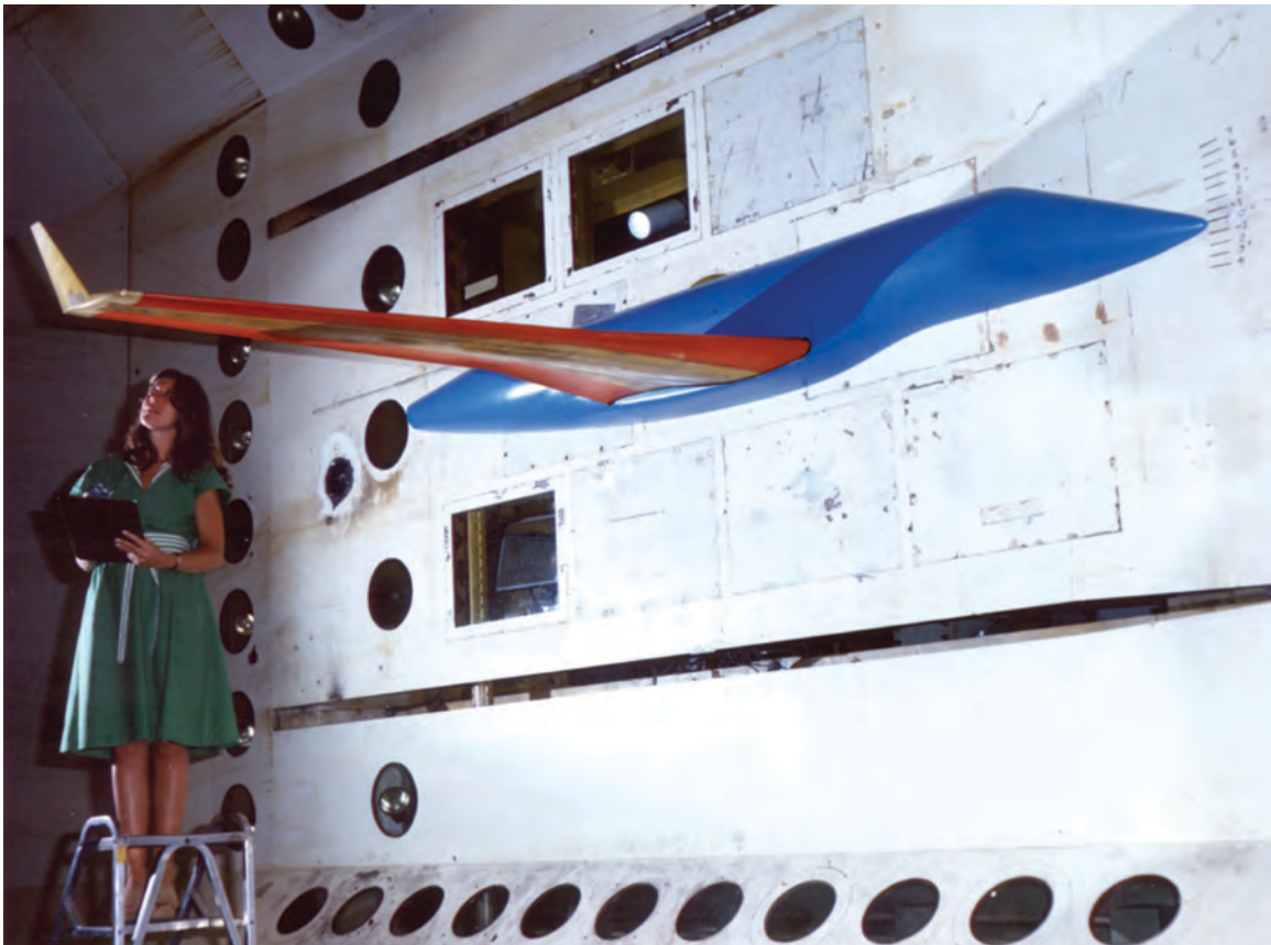
Patricia Cole inspects semispan model of Gulfstream III in TDT.
