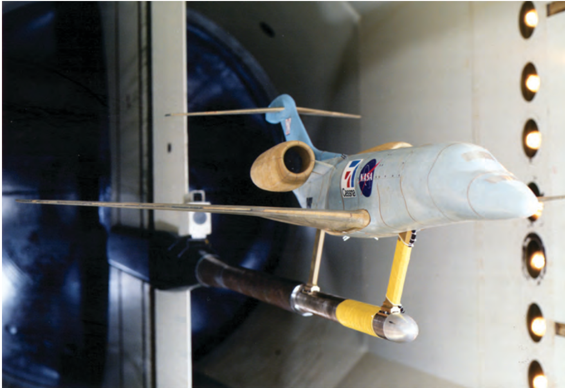
Full-span flutter model of Citation X.
