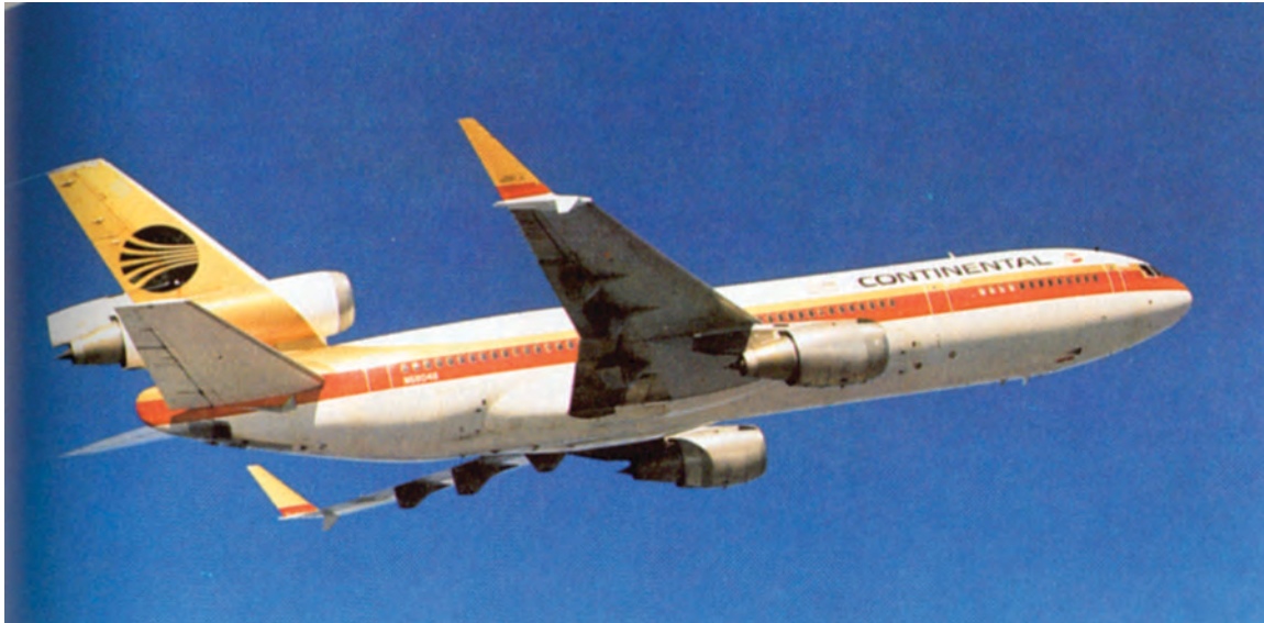
Modified DC-10 during Douglas winglet flight tests in 1981.
