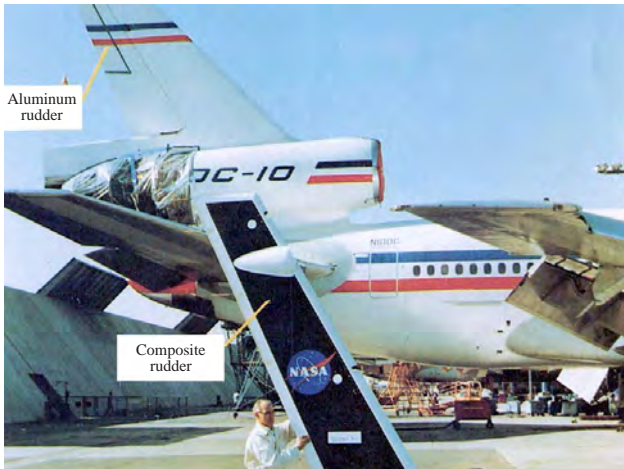
Composite upper aft rudder flown on McDonnell Douglas DC-10 in ACEE Program.
