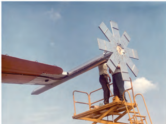
Langley's evaluation of spline device on C-54. Top photographs show VRF results for basic (left) and modified model, showing diffuse wake with spline. Lower photographs show installation of splines on full-scale aircraft.
