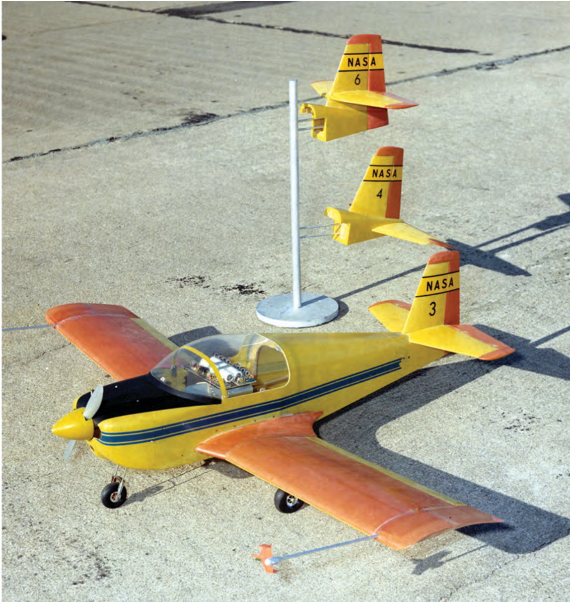
Some tail configurations tested on radio-controlled model of modified AA-1 aircraft.
