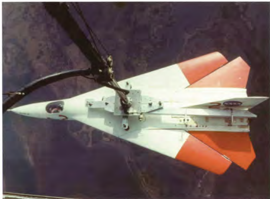
The F-111A drop model prior to launch from a helicopter for a spin-entry test.
