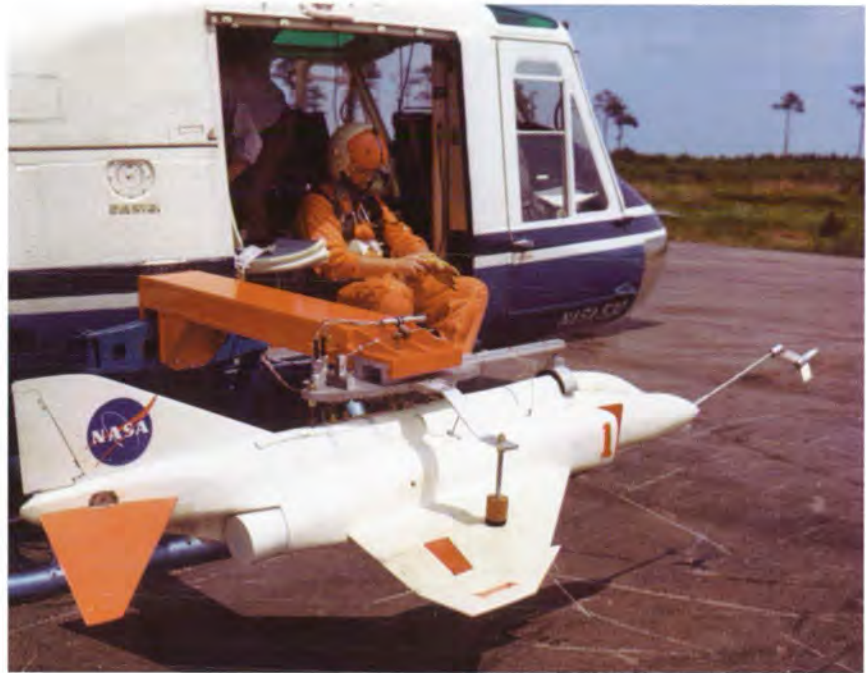
F-4 drop model mounted on the Langley helicopter drop rig for a spin entry test.
