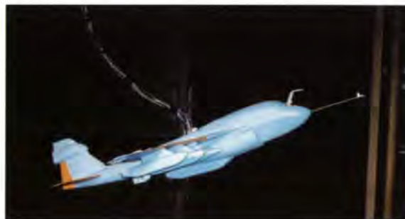
The modified EA-6B model in flight in the Full-Scale Tunnel.
