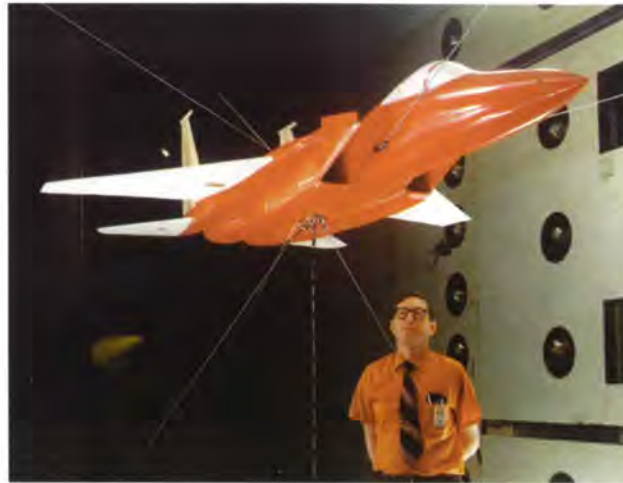
Langley researcher Moses Farmer with F-15 model in preparation for flutter tests in the 16-Foot Transonic Dynamics Tunnel.
