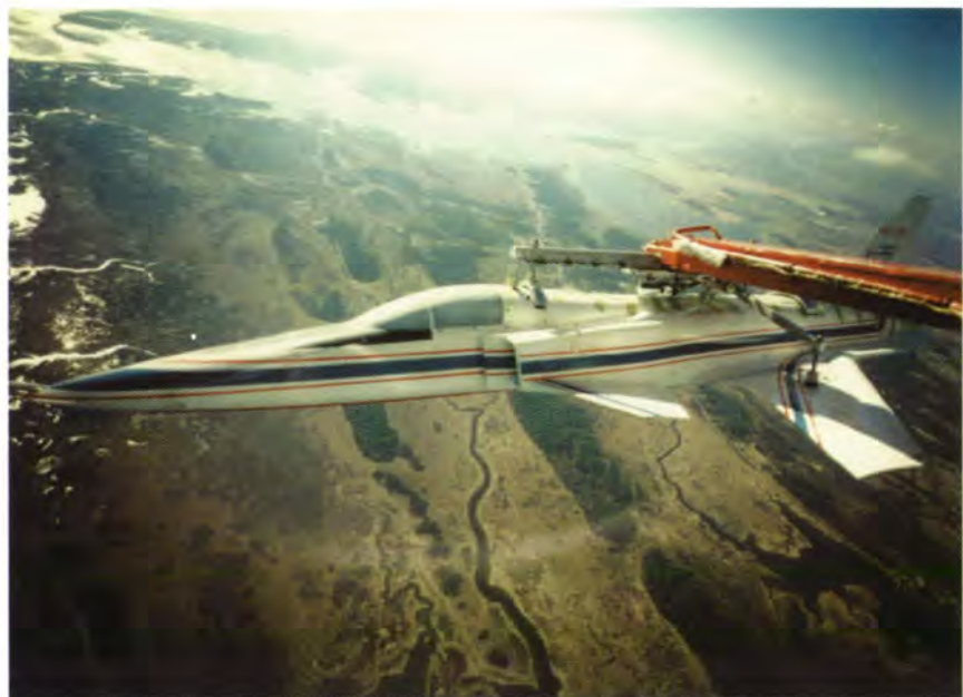
X-29 drop model mounted on launch apparatus on side of helicopter prior to release for post-stall tests.
