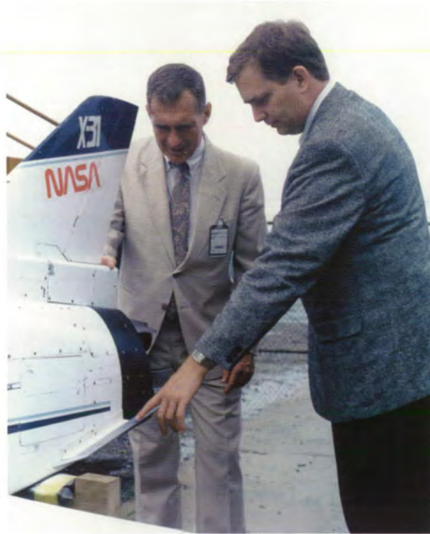
Mark Croom points to the aft-fuselage strakes defined by Langley tests and subsequently incorporated on the X-31 aircraft.
