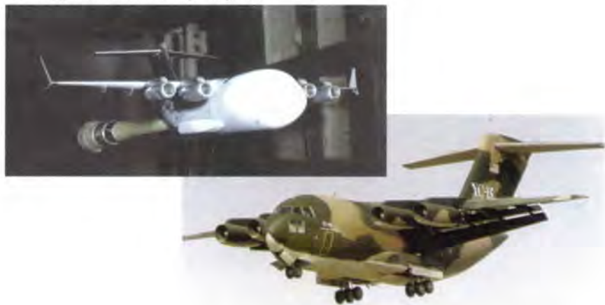
YC-15 model in the Langley 8-Foot Transonic Pressure Tunnel for an evaluation of winglets.
