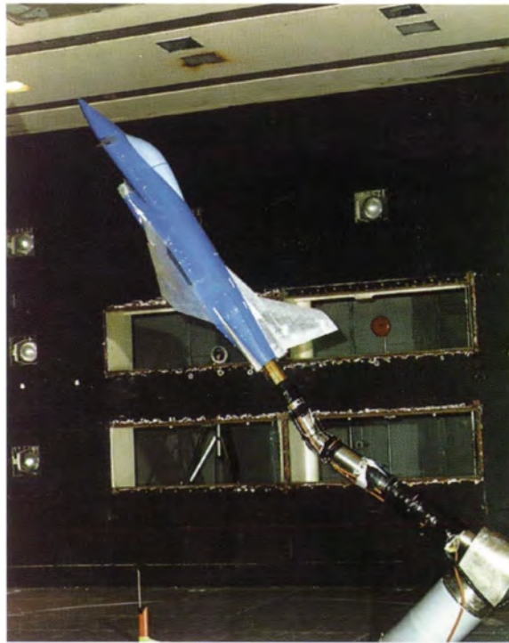
X-31 with F-16 canopy during tests in the Langley 14- by 22-Foot Low-Speed Tunnel.
