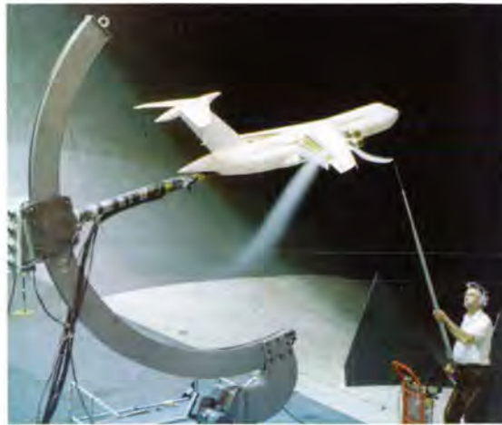
Langley engineer Charles C. Smith, Jr. conducts flow visualization studies on the modified C-5 model.
