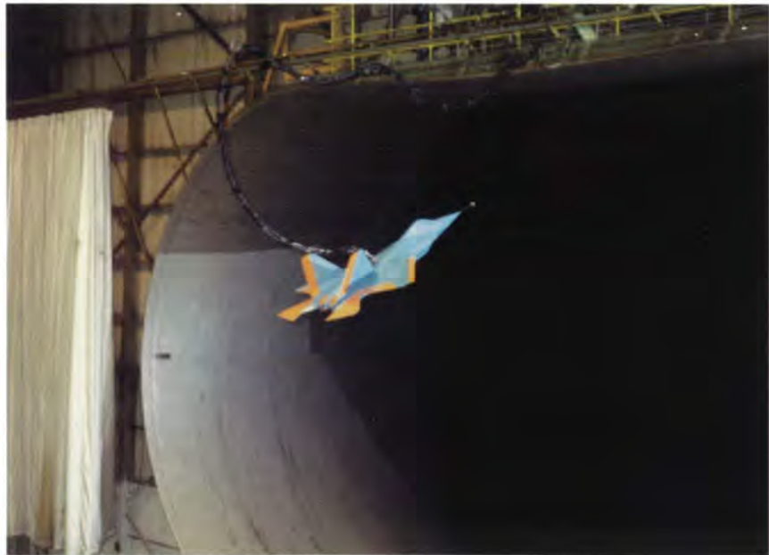
Free-flight tests of the YF-22 model in the Langley Full-Scale Tunnel in 1990.
