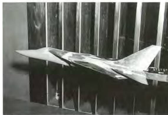
Supersonic tests of the early F-111 design in the Langley Unitary Plan Wind Tunnel in 1963.
