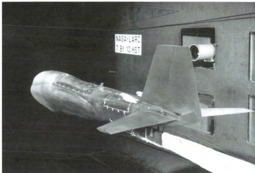
EA-6B fuselage and empennage model in the Langley 7-by 10-Foot High-Speed Tunnel for air scoop studies.
