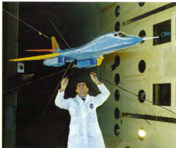
B-1A flutter model mounted in the Langley 16-Foot Transonic Dynamics Tunnel.
