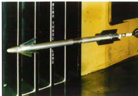
Sidewinder missile research model in the Langley Unitary Plan Tunnel.
