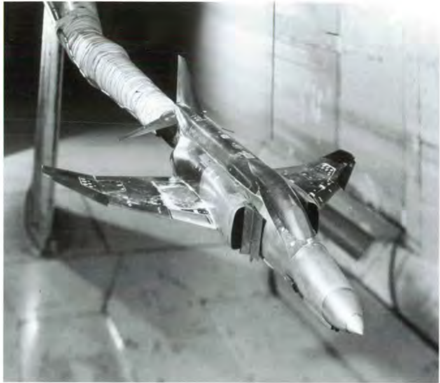
F-4E model in the Langley 7- by 10-Foot High-Speed Tunnel for evaluation of wing leading-edge modifications for enhanced maneuverability.
