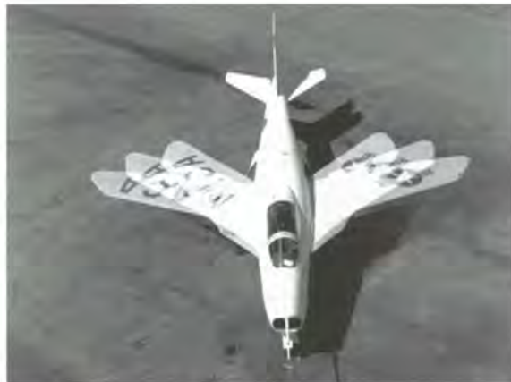
Time-lapse photograph of the Bell X-5 shows the wing at various sweep angles.
