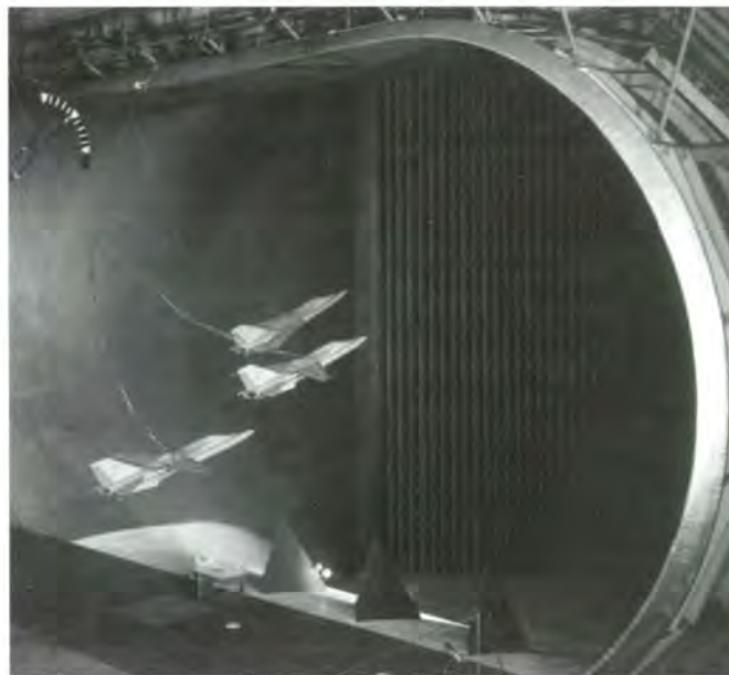
Time-lapse photograph of the F-111A free-flight model at several wings sweep angles during tests in the Langley Full-Scale Tunnel.
