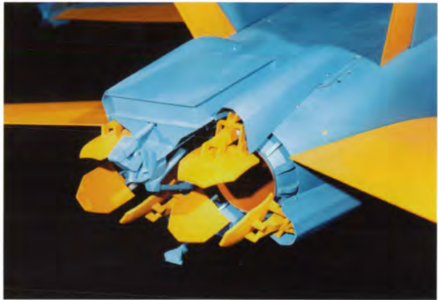
Thrust-vectoring vane installation on the F-18 HARV free-flight model with rectangular box above the vanes representing the container for the spin parachute.
