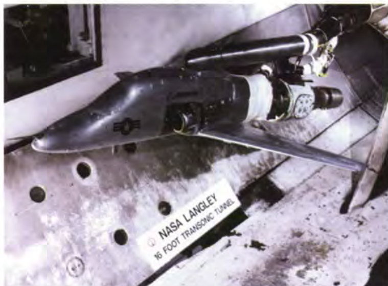
T-45 inlet performance model in the Langley 16-Foot Transonic Tunnel.
