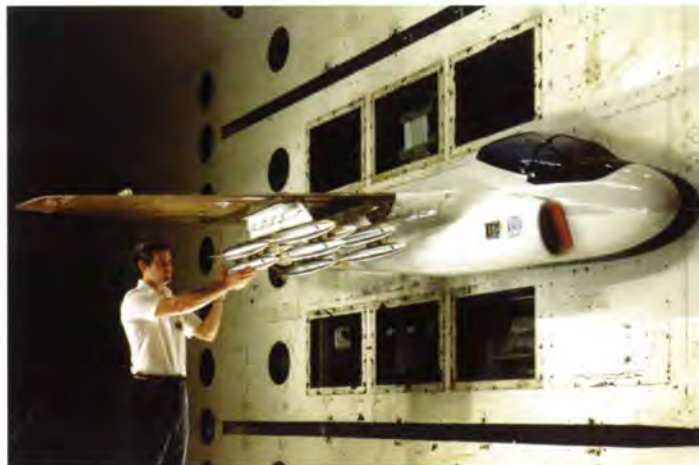
Flutter tests of the new A-6 composite wing in the Langley 16-Foot Transonic Dynamics Tunnel included numerous external store loadings.
