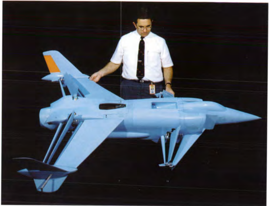
Langley researcher William Newsom with the XFV-12A free-flight model with augmentor doors on wing and canard open.
