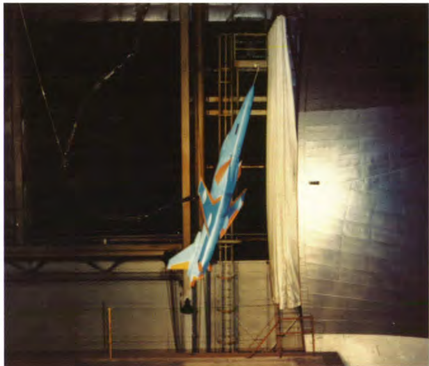
X-29 ADEN model flying at an angle of attack of 80 deg in the Langley Full-Scale Tunnel.
