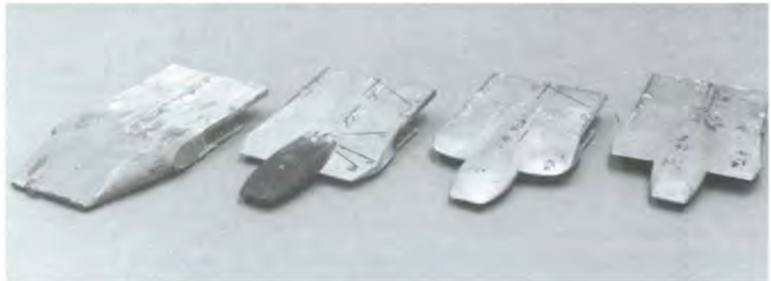
Pancake configurations evaluated in cruise-drag studies in the Langley 16-Foot Transonic Tunnel. Original shape is at left.
