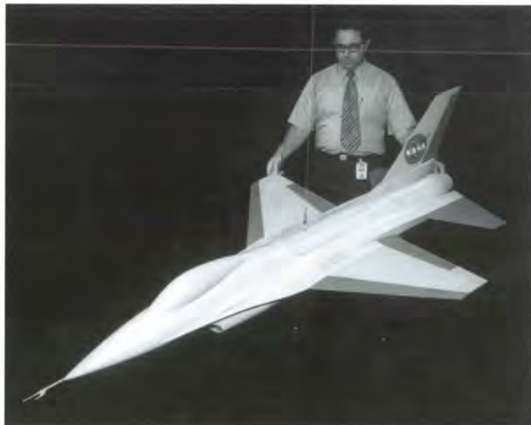
Researcher William A. Newsom, Jr. with the free-flight model of the YF-16 used in tests in the Full-Scale Tunnel.
