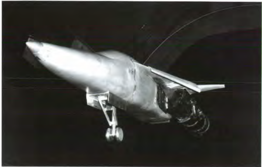
Inlet tests of an F-111 model in the Langley 16-Foot Transonic Tunnel.
