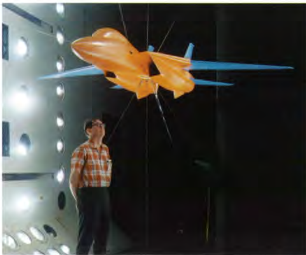
F-14 model mounted in preparation for flutter tests in the 16-Foot Transonic Dynamics Tunnel.
