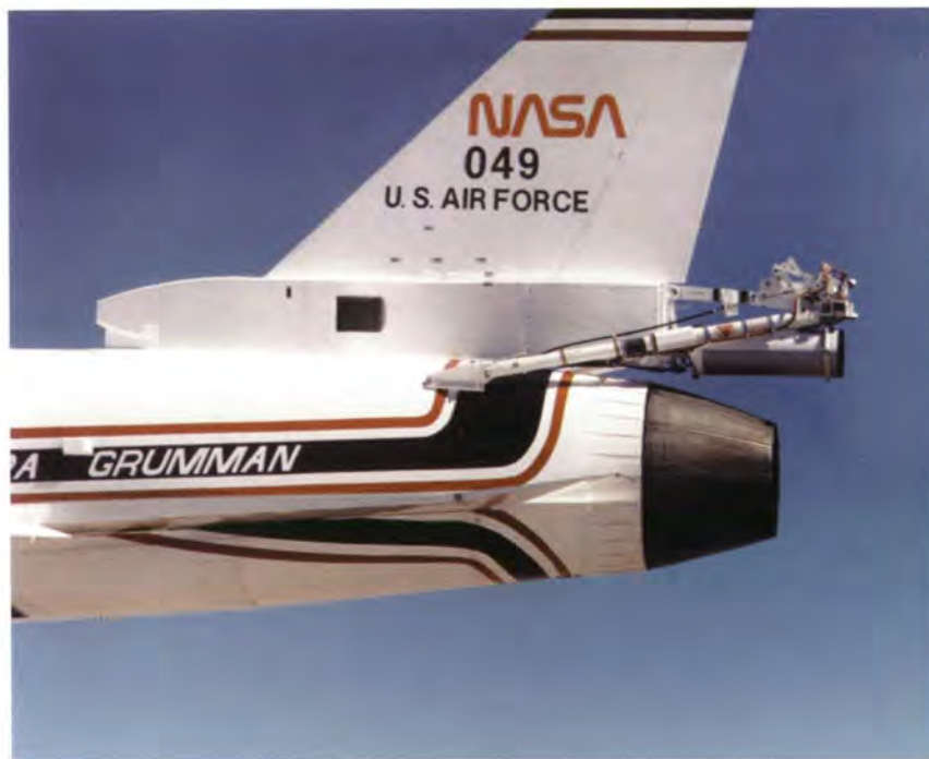
The spin parachute and truss assembly on the X-29 during high-angle-of-attack tests at Dryden.
