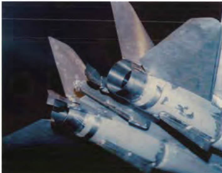
F-14 model equipped with deflectable yaw vanes in the Langley 16-Foot Transonic Tunnel.
