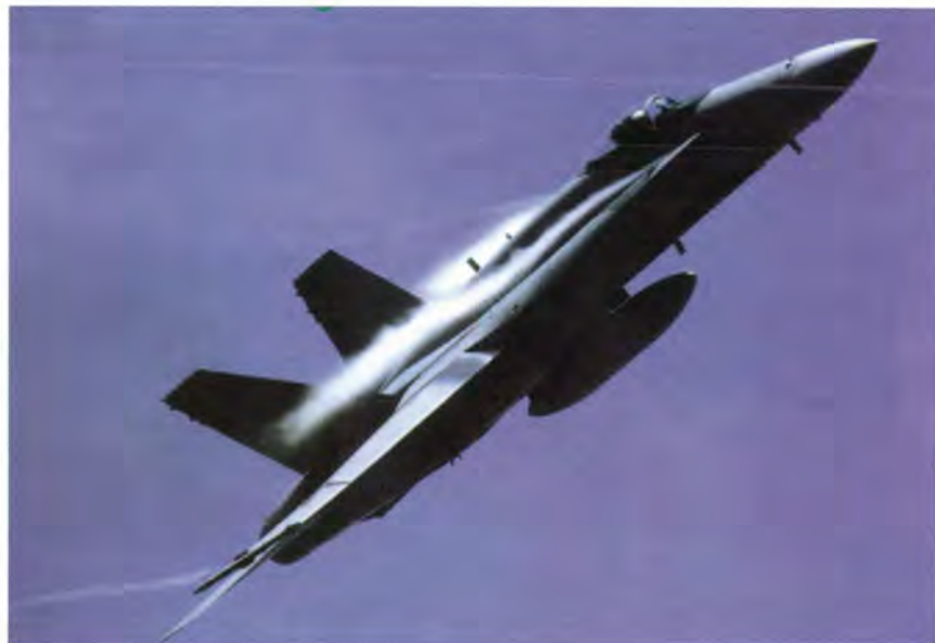
F/A-18 with wing leading-edge flaps deflected and LEX vortices made visible by condensation.
