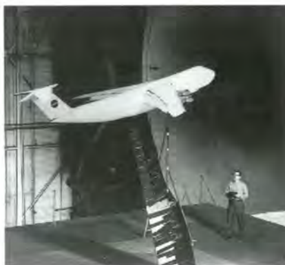
Powered C-5 model mounted in the Langley Full-Scale Tunnel for externally blown flap assessments with the double-slotted flap configuration.
