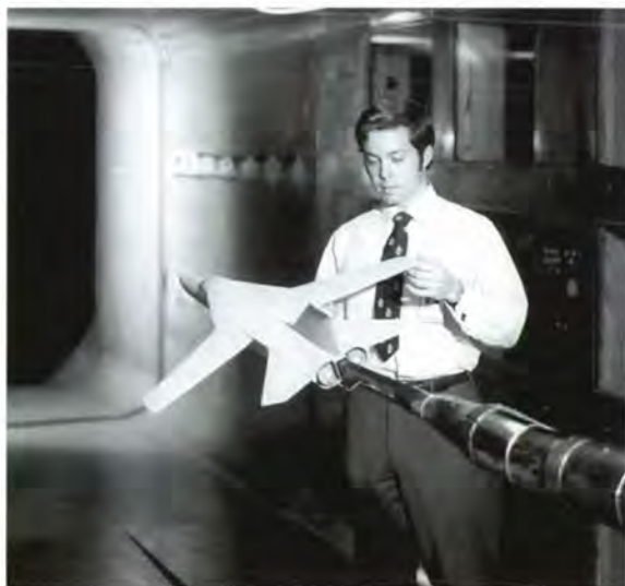
James B. Hallissy inspects the F-111 TACT model in the Langley 8-Foot Transonic Pressure Tunnel.
