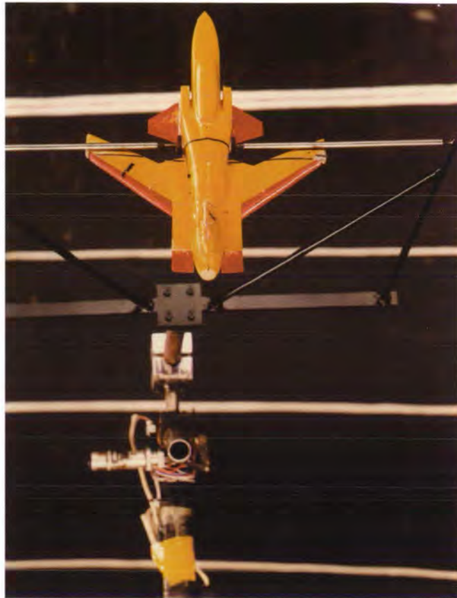
X-29 model mounted on single-degree-of-freedom pitch-tumble test apparatus in the Langley Spin Tunnel.
