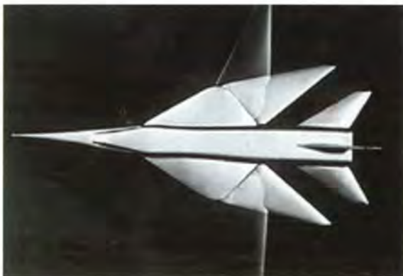
Configuration IV, which was the breakthrough model for variable-sweep technology.
