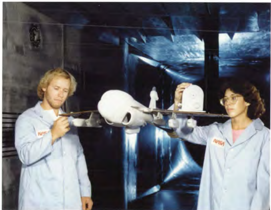
EA-6B model being prepared for tests in the National Transonic Facility at Langley.
