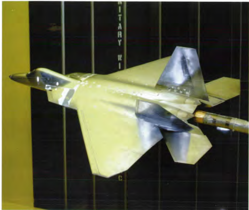
F-22 model mounted for supersonic test in the Langley Unitary Tunnel.
