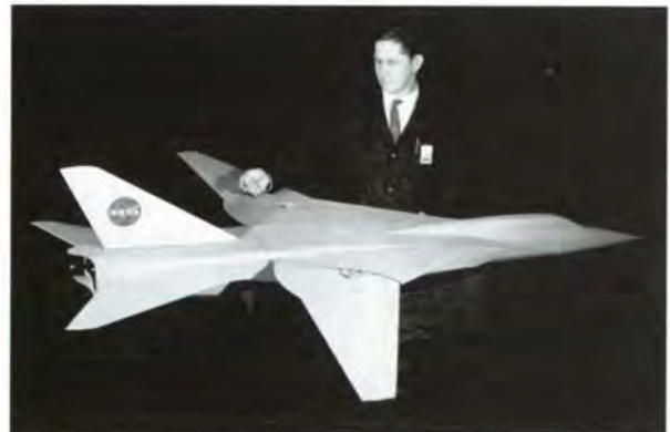
James L. Hassell, Jr. with a free-flight CAP model that was flown in the Langley Full-Scale Tunnel.
