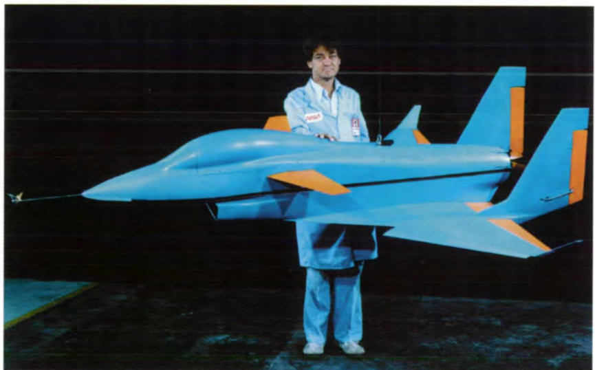
The modified SNAKE configuration after the Langley tests with upturned wingtips, wing leading-edge flaps, enlarged vertical tails, enlarged wing-fuselage strake, and nose strakes.
