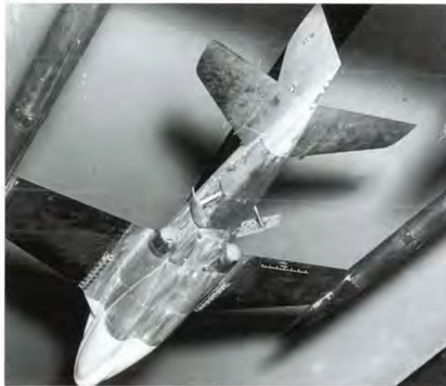
Powered-model tests in the Langley 16-Foot Transonic Tunnel evaluated several speed brake configurations.
