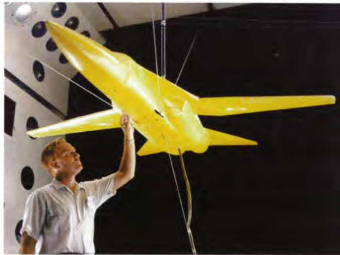
F-111 model in the Langley 16-Foot Transonic Dynamics Tunnel in 1963. (Tail surfaces were later changed to avoid flutter.)
