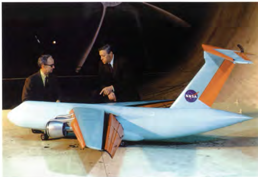
Langley researcher John P. Campbell (l) and Gerald G. Kayten (r) of NASA Headquarters inspect a free-flight model of an EBF configuration in the Langley Full-Scale Tunnel.
