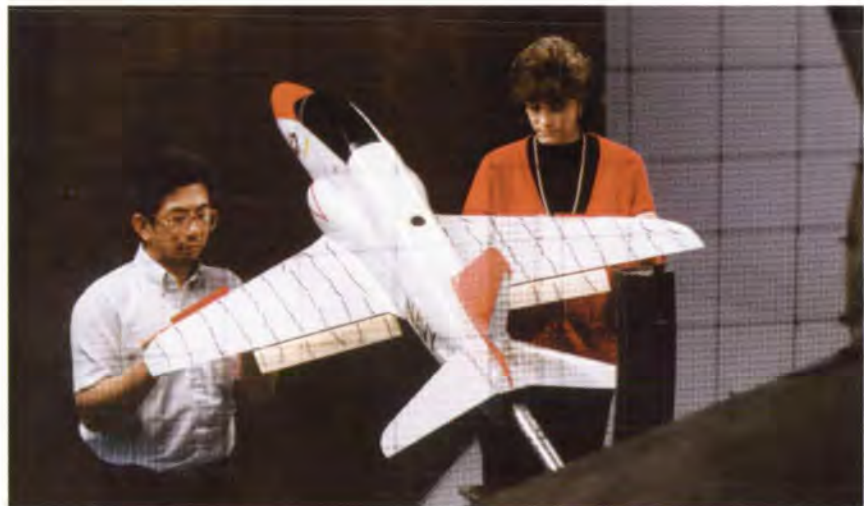
Langley researchers Long P. Yip and Holly M. Ross examine a T-45 model with a discontinuous leading-edge modification in the Langley 12-Foot Low-Speed Tunnel in 1989.
