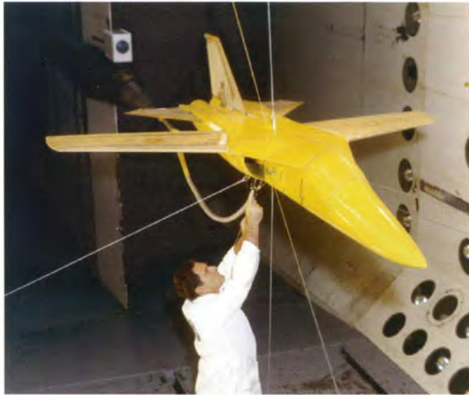
F-111 TACT model mounted for flutter tests in the Langley 16-Foot Transonic Dynamics Tunnel in 1971.
