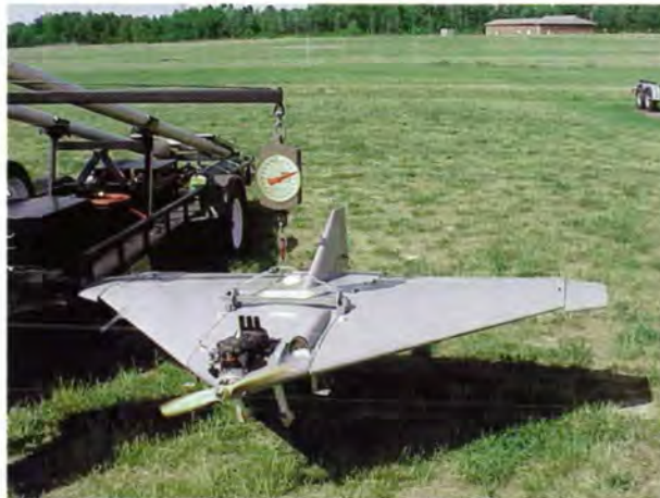
An Exdrone undergoes weight and balance tests.
