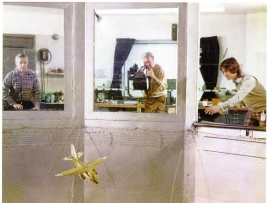
S-3 model launched into the vertically rising airstream in the Langley Spin Tunnel.
