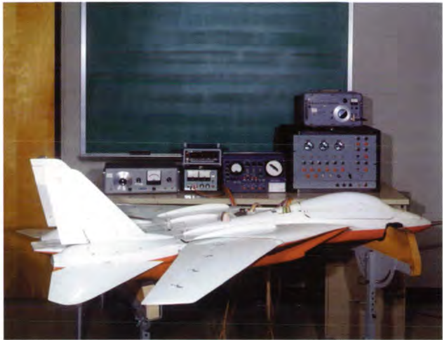
F-14 drop model being calibrated in flight electronics lab prior to flight tests.
