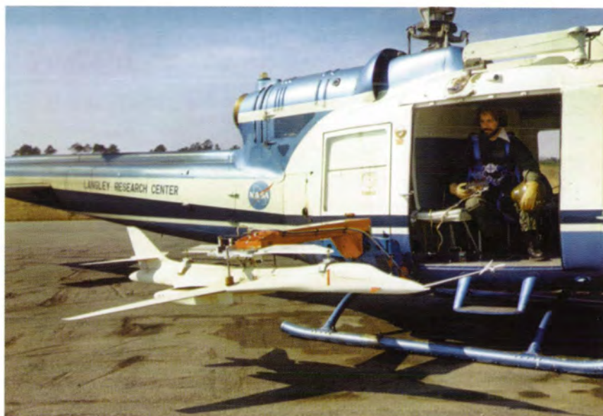
B-1A drop model being prepared for helicopter drop test in 1974.
