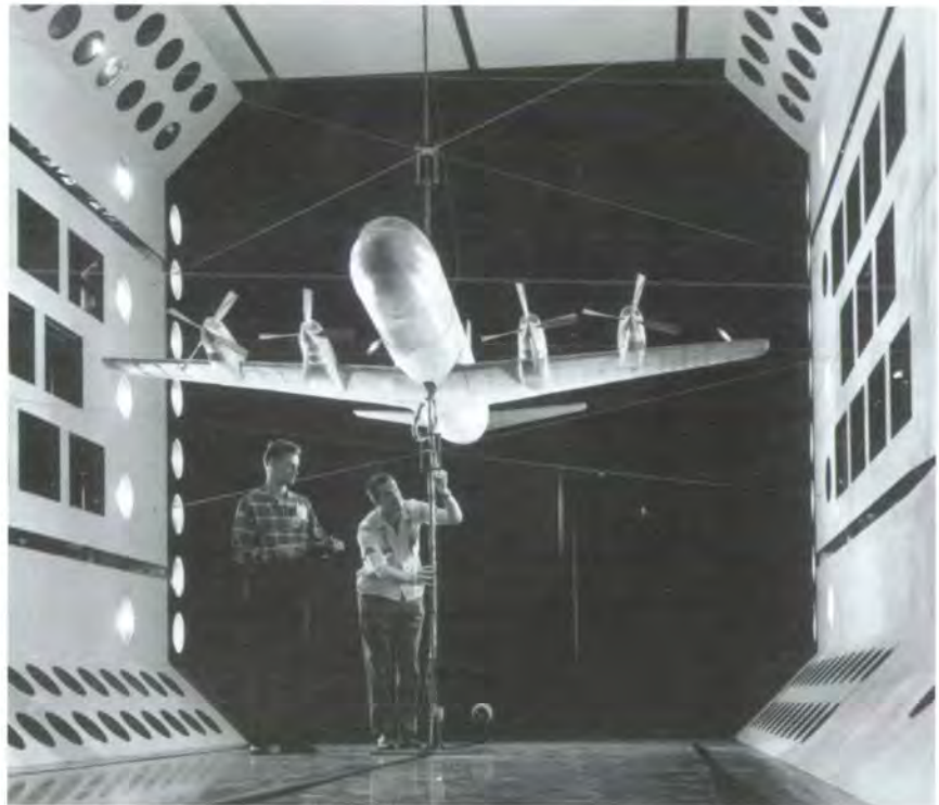
Powered model of the Lockheed Electra mounted in the Langley 16-Foot Transonic Dynamics Tunnel for flutter tests.
