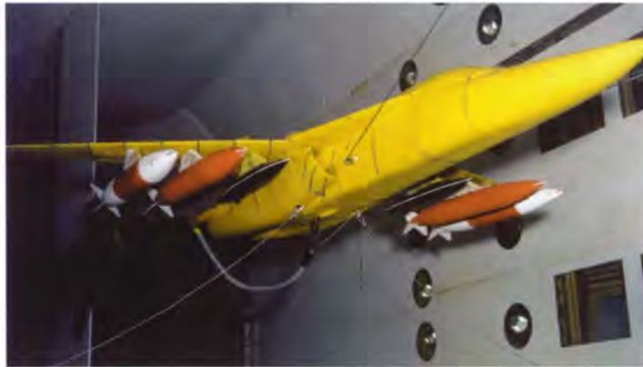
FB-111 flutter model illustrating the wide scope of external stores that were tested in the program.
