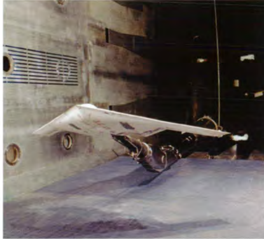
B-2 model during tests in the National Transonic Facility (NTF) at Langley.
