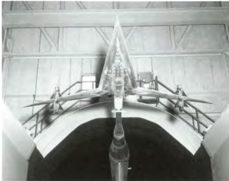
The radical British Swallow configuration in the Langley 16-Foot Transonic Tunnel with variable sweep arrow wing and over and under wing-mounted engines.
