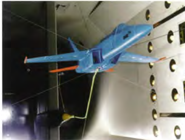
F/A-18E/F model mounted for flutter tests in the Langley 16-Foot Transonic Dynamics Tunnel.
