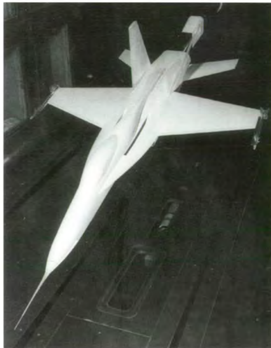
YF-17 model in the Langley 8-Foot Transonic Pressure Tunnel for drag assessment studies.
