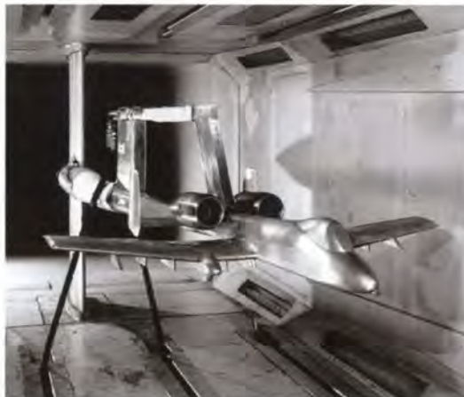
Powered-model tests of the Fairchild A-10 with engines supported by an auxiliary upper sting in the Langley 7- by 10-Foot High-Speed Tunnel.
