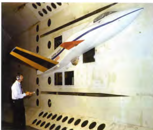
Rodney Ricketts with the Grumman FSW model during aeroelastic divergence tests in the Langley 16-Foot Transonic Dynamics Tunnel.
