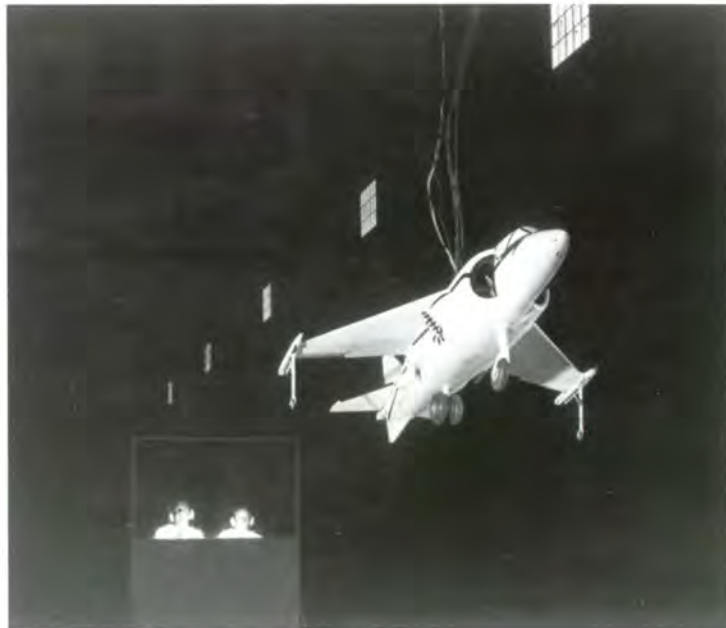
Shielded by a protective panel, Langley researchers Robert O. Schade and Louis P. Tosti hover the 1/6-scale free-flight model in the airflow return passage of the Full-Scale Tunnel.
