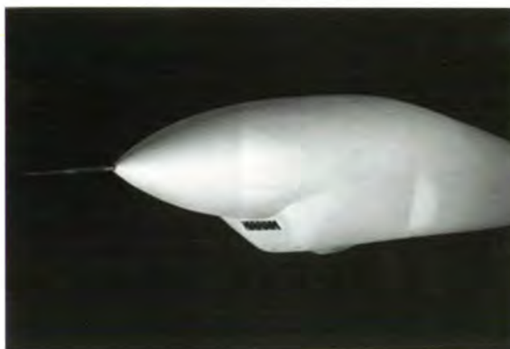
Simplified model of RF-4 nose tested in the Langley 16-Foot Transonic Dynamics Tunnel.
