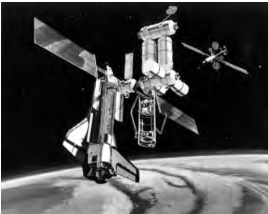
This 1982 artist's conception depicts a mature space station configuration, which includes two solar panels to provide power; several modules for command, habitation, and experimental activity; a Shuttle-sized unpressurized rack for the storage of payloads; advanced remote manipulator systems for the assembly of large structures and the servicing/storage of satellites and instruments; and a docking/utility hub that might serve in addition as a "safe haven" in case of emergency. Attached to the station in this picture is a
