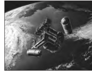
Lunar Transfer Vehicle would have provided transportation between Space Station Freedom and lunar orbit (Source: 90-Day Study)
