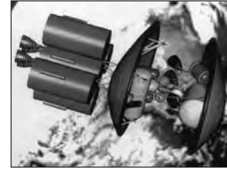
Mars Transfer Vehicle would have propelled crew and Mars excursion vehicle to Mars orbit (Source: 90-Day Study)
