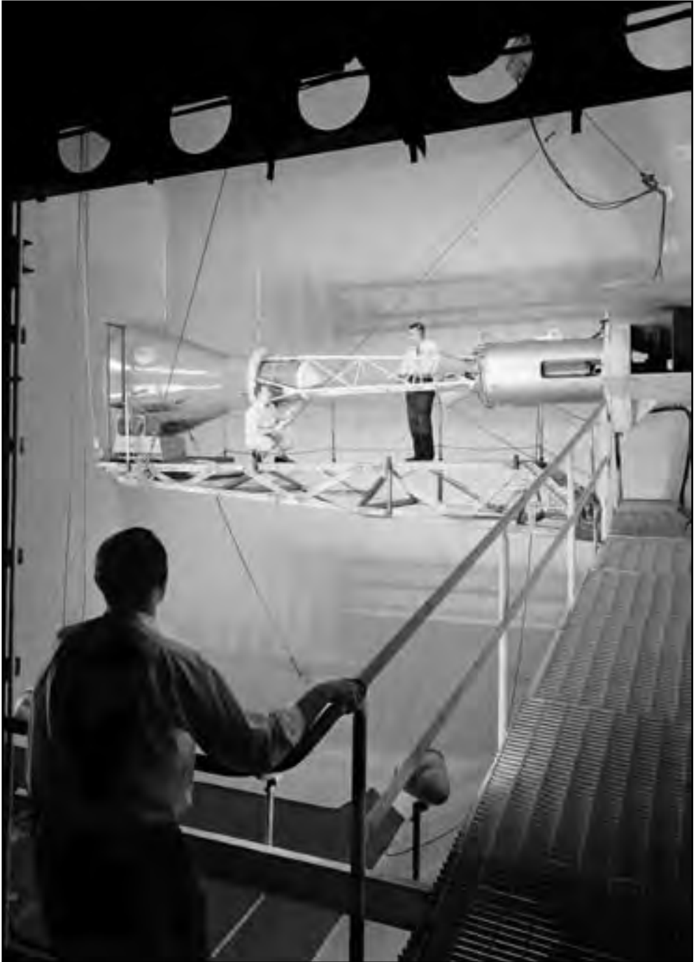
Image 149: A Mercury capsule is mounted in the Altitude Wind Tunnel for a test of its escape tower rockets. The AWT was quickly modified and became the center of NASA Lewis's work on Project Mercury. (NASA C-1960-53287)
