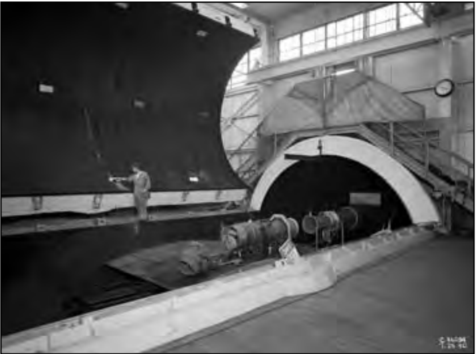
Image 36: The test section lid, seen raised in this photograph, was 40 feet long, 20 feet wide, and 10 feet high. A motor-driven system using large counterweights, pulleys, and cables could open and close the lid in approximately 10 minutes. The lid contained a number of viewing windows and a portal for a periscope camera. Handwheels were used to seal the lid once it was lowered in place. (NASA C-1950-26294)
