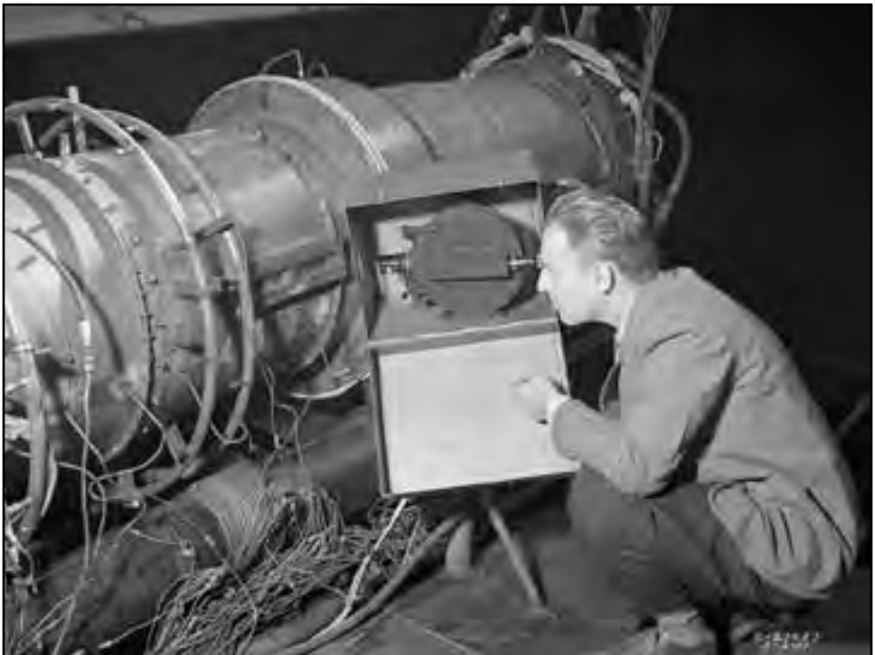
Image 112: A camera is set up in the AWT to film the combustion process in the afterburner of the Westinghouse 24C-WE-22 engine. Bob Walker recalled that, as a colleague was leaning onto the test section lid to monitor one of the Westinghouse runs through a portal, the engine seized—causing the turbine wheel to fly off. “We tended to doze up there on the midnight shift. He said, ‘man, I thought I was going to jump right off the lid, that wheel came right past the window.’ He was truly excited about that. It really wrecked that engine.” 244 (NASA C-1951-27657)
