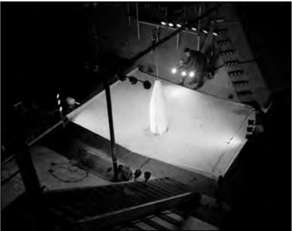
Image 250: A one-sixth-scale model of the failed AC-21 shroud is set up inside SPC No. 2. Investigators found that the spring actuators failed to jettison the shroud because of some restraint in the shroud. When the restraint was freed, it took over 8 minutes for the springs to release the shroud. The flight data on hinge strain and the accelerometer indicated that the latch system was the most probable cause. 540 (NASA C-1971-01491)
