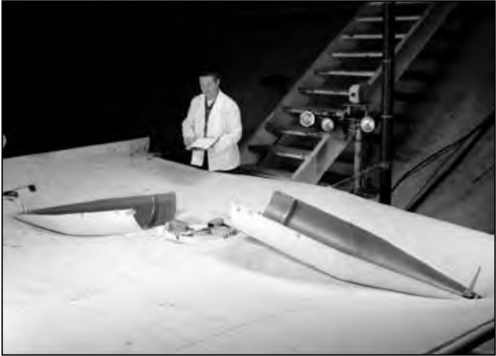
Image 251: The AC-21 shroud is investigated in SPC No. 2. The fairing was joined by 16 latches with no backup systems or redundancy. The board recommended adding mechanical redundancy to each nut, the self-containment of the separation nut and interface, additional inspections to ensure hardware conformity, and identification and removal of all nonflight hardware. Other recommendations were verification of cleaning fluids and the resolution of discrepancies of on-site fixes. 541 (NASA C-1971-01488)
