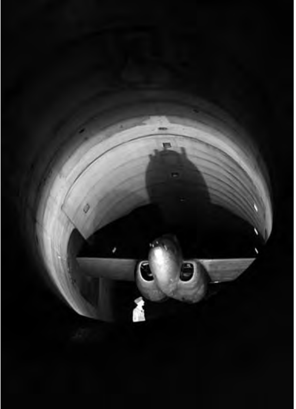
Image 40: The secret test of the Bell YP-59A Airacomet was the first investigation in the new Altitude Wind Tunnel. The Airacomet was the first aircraft in the United States powered by a jet engine, the General Electric I-16. (February 1944). (NASA C-1944-04830)
