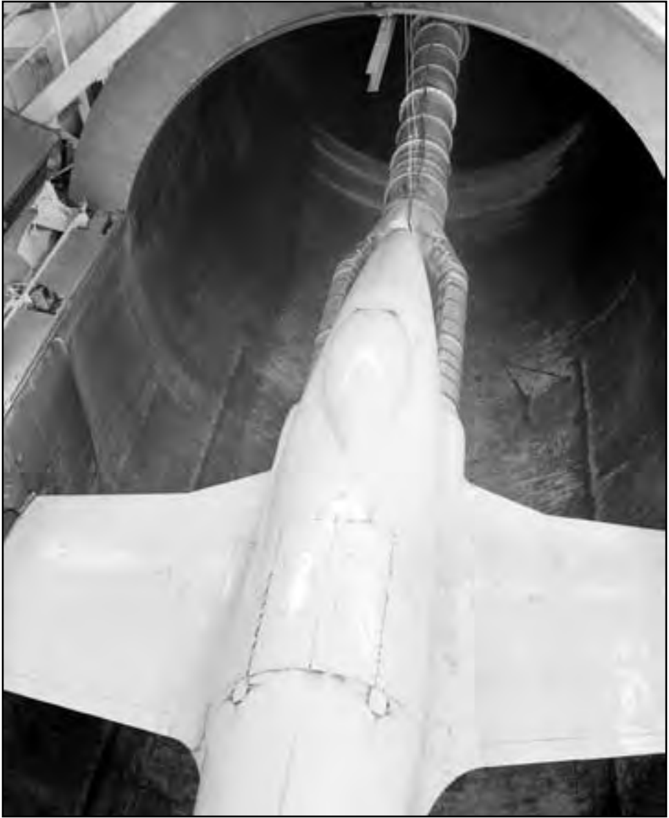
Image 53: Lockheed YP-80A with its GE I-40 engines being tested in the AWT. One of the modifications required to test jet engines in the AWT was the ducting of conditioned airflow directly to the engine inlets. This method effectively reduced the tunnel size but allowed greater speeds and altitude conditions for the engine. The direct-connect method was used for all future turbojet and ramjet tests in the AWT. (NASA C-1945-09446)
