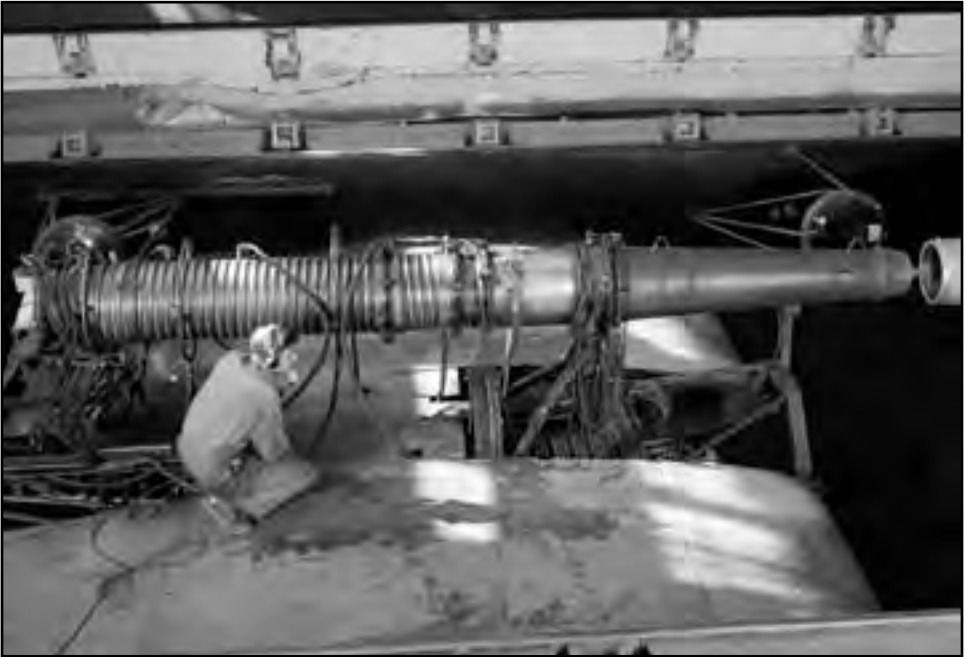
Image 83: A 16-inch ramjet is installed in the AWT to study inlet shocks for the Project Bumblebee missile. The free jet air allowed the supersonic ramjet to be studied in the subsonic wind tunnel. The 18-foot-long ramjet was tested in the AWT from January through May 1949. Initially there was some concern with the number of contractors to be given clearance and allowed to witness the tests. A request from United Aircraft Corporation to have a representative present was declined. 225 (NASA C-1949-23409)
