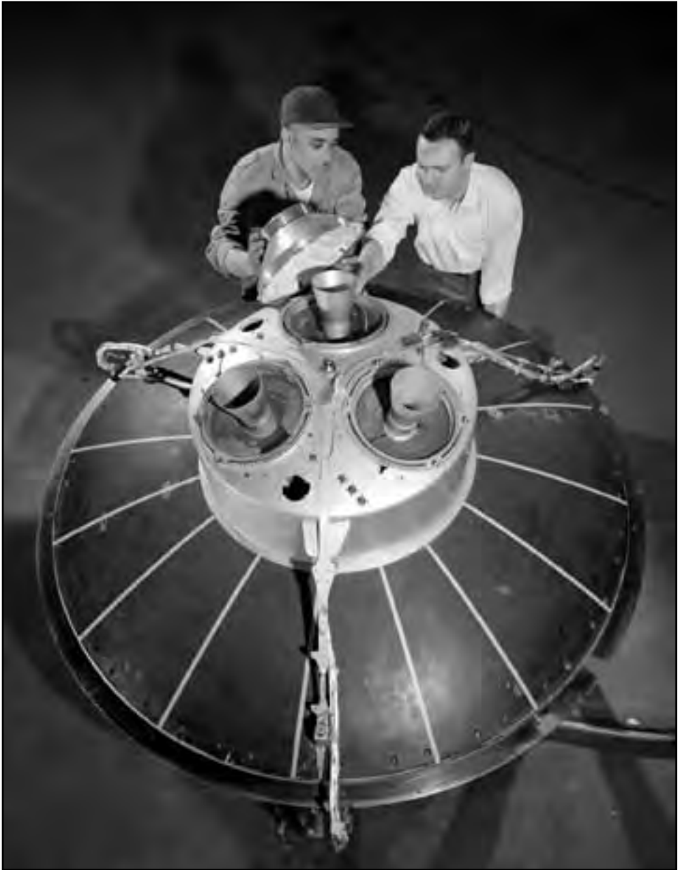
Image 169: Left: Gale Butler examines the Mercury capsule's retrograde rockets prior to a test run inside the AWT. These studies showed that a previous problem concerning delays igniting the propellant had been resolved. Follow-up runs verified the reliability of the coated igniter's attachment to the propellant grain. In addition, the capsule's retrorockets were calibrated so that they would not alter the capsule's position when fired. (NASA C-1960-53146)
