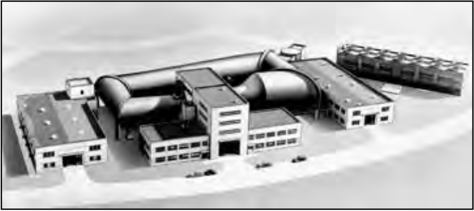
Image 11: Early drawing of the new AWT, which was originally referred to as the “Engine Research Tunnel.” It was the nation’s first wind tunnel built to study engines under simulated flight conditions. (NASA C-1944-05308).
