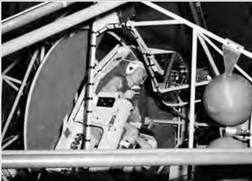
Image 162: John Glenn begins his tests on the MASTIF. (NASA C-1960-52741)
