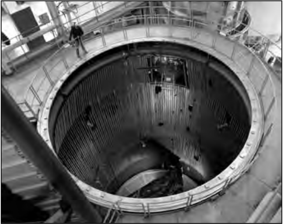
Image 253: Space Propulsion Facility at Plum Brook Station. The facility, with its lid propped open to the left, combined some of SPC No. 1's space simulation methods and added the ability to fire large rocket engines in a vacuum. Its first tests in 1970 verified that Centaur could be flown without its boost pumps. In 1985 the Space Propulsion Facility was named a National Historic Landmark. (NASA C-1987-02664)
