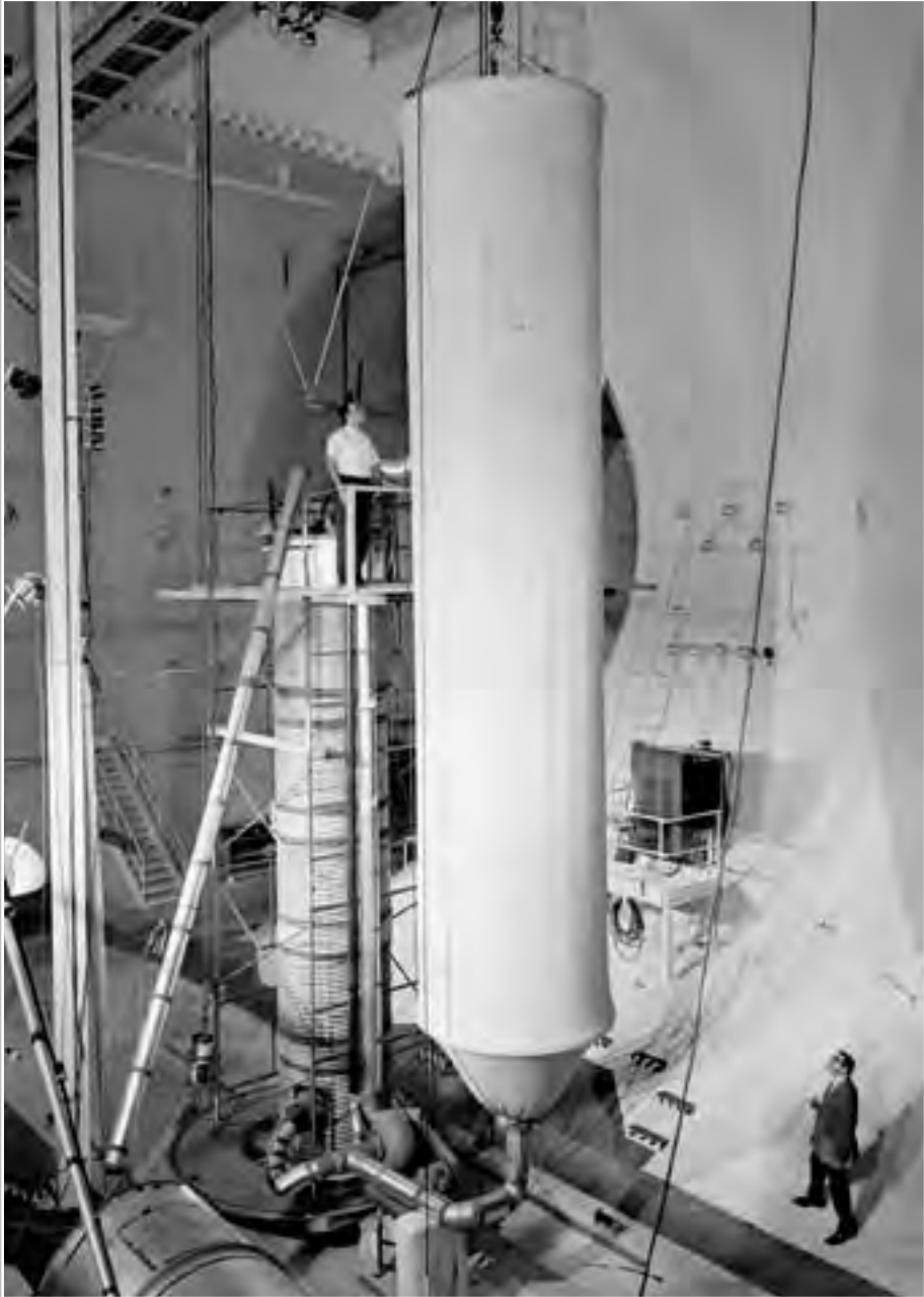
Image 243: In late 1965, tests of deceleration pellets for the new Zero Gravity Facility, which was about to come online, were conducted in SPC No. 2. A 5-foot-diameter, 20-plus-foot-tall deceleration stand was mounted vertically in the chamber floor and filled with polystyrene pellets. Objects were dropped through a penetration in the roof into the decelerant to determine which types of pellets worked best. (NASA C-1966-01954)
