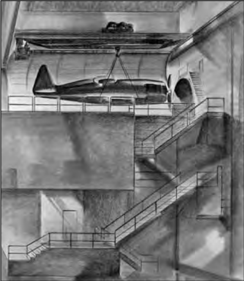
Image 10: A full-scale aircraft is lifted into the AWT's test section. Although testing full-size versions reduced the cost, time, and effort of developing engines, it also required a substantial investment in large facilities. Many of the NACA's achievements resulted from its willingness to make those investments. (NASA C-1944-06305)
