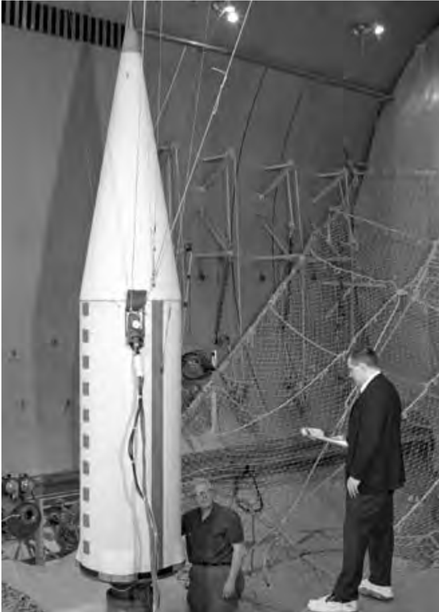
Image 241: The Weightlessness Analysis Sounding Probe sounding rocket is tested in SPC No. 1 in April 1966. During the 7 June 1966 sounding rocket launch off of Wallops Island, the propellant was purposely sloshed by a thruster on the side of the tank. The tank contained a baffle ring that quickly settled the sloshing fuel. 515 The 862-pound rocket reached an altitude of 250,000 feet before freefalling back to Earth. The almost 7 minutes of microgravity during freefall provided researchers with enough data to launch the first orbital Saturn IB one month later. 516 (NASA C-1966-01838)
