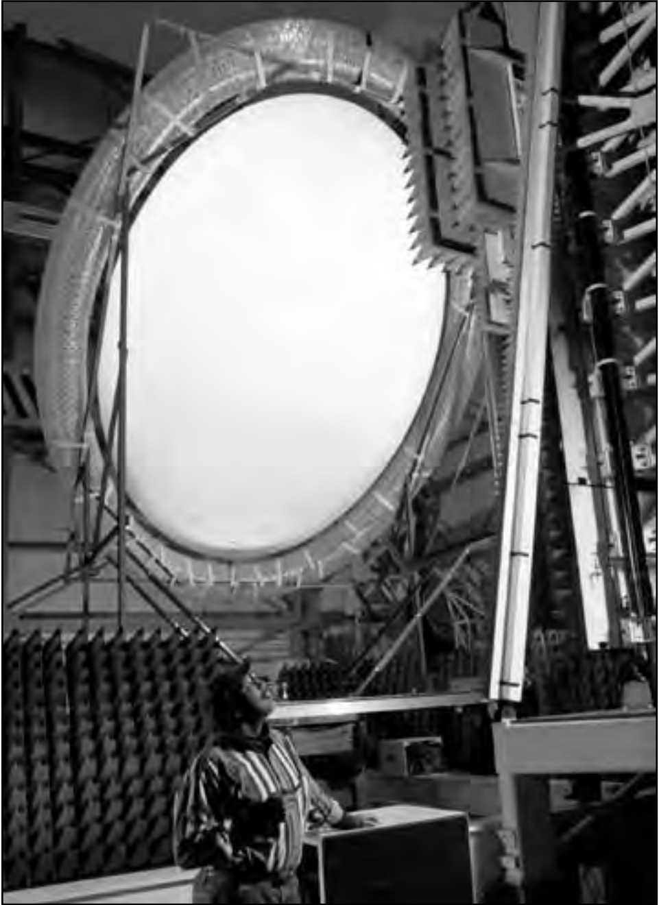
Image 267: Bill Darby, a mechanical engineering technician, stands beneath an inflatable membrane antenna inside the Near-Field Antenna Test Facility in the high bay. The 4- by 6-meter offset-parabolic inflatable membrane reflector and software were developed to demonstrate that a novel ground station composed of an array of relatively small apertures could economically replace a single, expensive tracking ground station. (NASA C-2004-01883)
