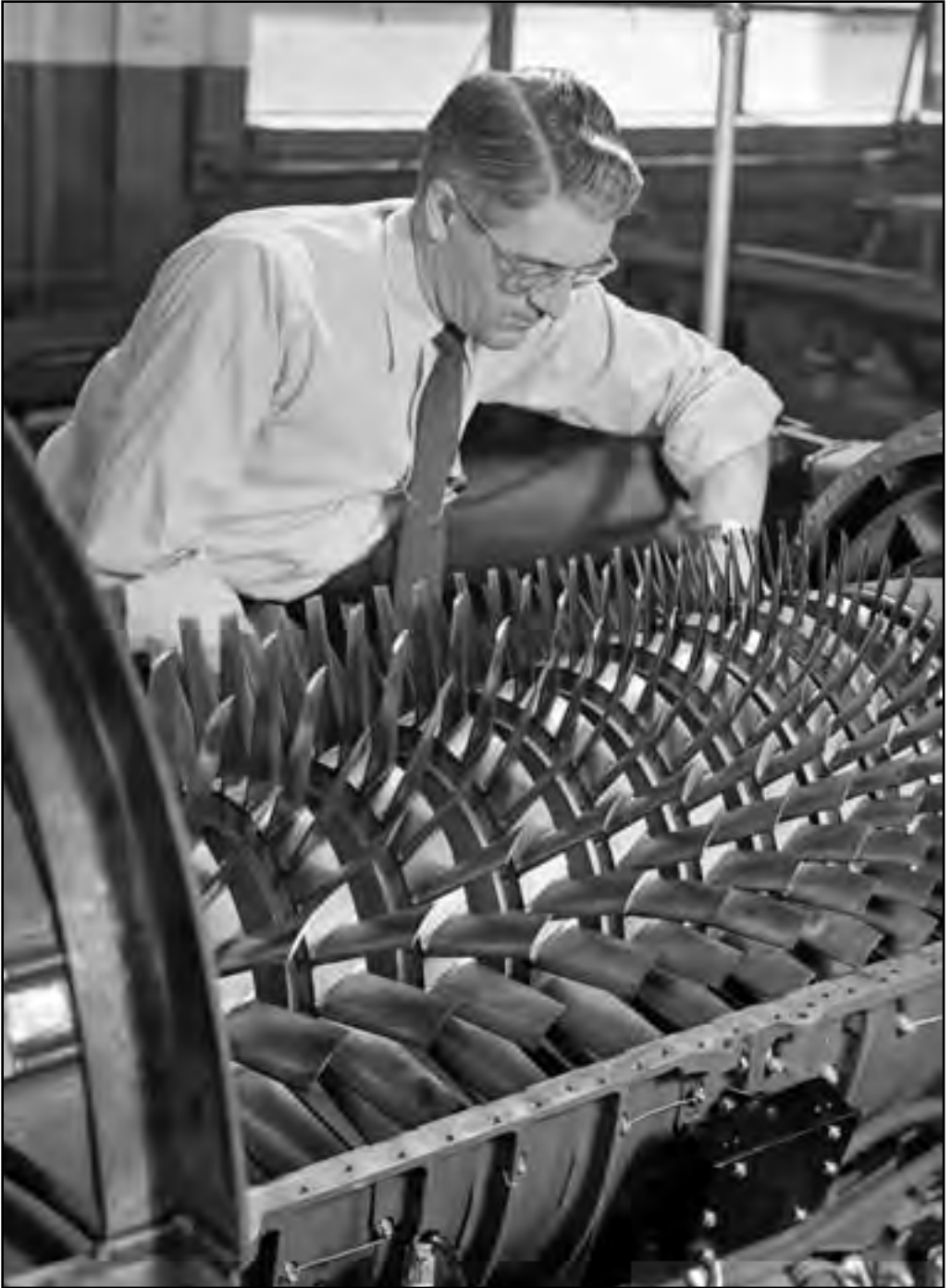
Image 59: A researcher examines the stator blades on a Westinghouse 24C axial-flow turbojet engine in the shop area. Axial-flow engines, with multiple stages or rows of compressor blades as shown here, were studied extensively in the Altitude Wind Tunnel. (NASA C-1950-26086)
