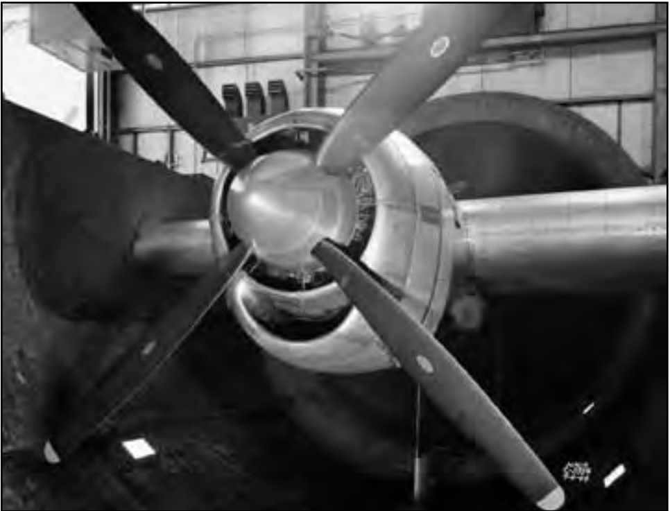
Image 54: The AWT was used to study the engine cooling problems for the Boeing B-29 Superfortress for the Pacific phase of World War II. The B-29's right inboard nacelle and wing section were installed in the AWT test section from May to September 1944. As part of this series of tests, several different flap designs were studied on the Wright R-3350 engine's 43-inch-diameter cowl inlet. The logbook notes that the day shift “washed model for pictures” prior to this midday 4 July photograph. 147 (NASA C-1944-05554)
