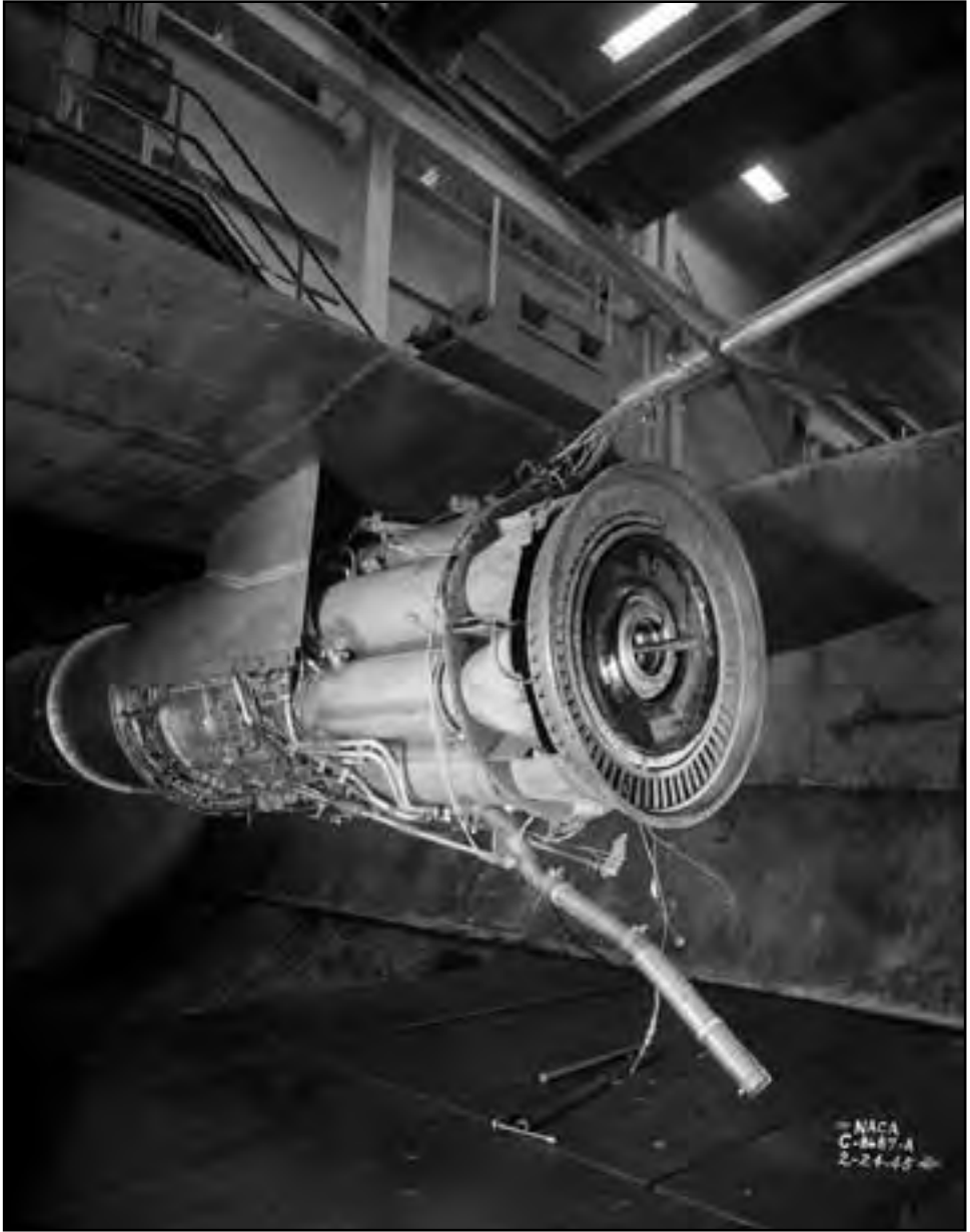
Image 66: Eleven-stage axial-flow GE TG-180 installed in the AWT test section. The initial tests focused on the benefits of tailpipe burners, or afterburners, to improve thrust. One area of research determined the performance of a 29-inch-diameter tailpipe burner over a range of altitude conditions using several different flameholders and fuel systems. AERL researchers determined that the optimal design was a three-stage flameholder with its largest stage upstream. 179 (NASA C-1945-08687)
