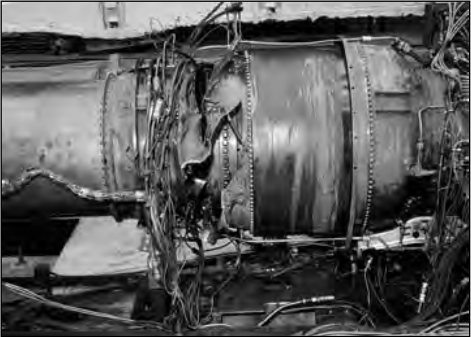
Image 138: The Pratt & Whitney J57 was tested extensively in the AWT from December 1953 to February 1954. General performance characteristics, inlet pressure distortions, and combustion efficiency were studied. Near the end of the investigations, one of the J57-P-1 engines suffered a major failure, seen in this photograph. (NASA C-1954-37208)
