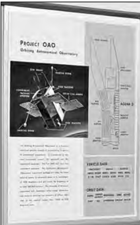
Image 235: The text on this 1965 poster states: "The OAO is a precisely stabilized satellite capable of accommodating a variety of astronomical experiments. It is comprised of two main component systems: the spacecraft and the experiment packages. The first OAO will carry two experiment packages. The Smithsonian Astrophysical Observatory experiment package will map the entire celestial sphere in ultraviolet down to a wavelength of 1100 Angstroms and will record the brightness of at least 200,000 hot stars. The University of Wisconsin experiment will determine stellar energy distribution and measure emission line intensities of diffuse nebulae in the spectral region from 3000 to 800 Angstrom units." (NASA C-1965-74461)
