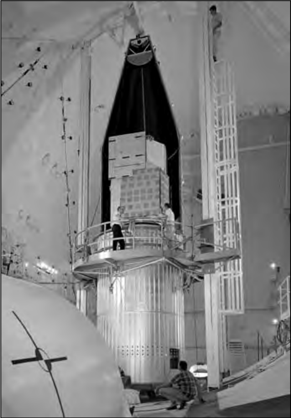
Image 236: Lewis engineers work on the OAO-1 test setup in SPC No. 2. One-half of the large clamshell nose fairing is removed in this photograph, revealing the 10-foot-long, 4-foot-diameter OAO-1 payload. The solar panels are folded flat against the satellite as they would be during a launch. A platform elevator with an 11-foot inside diameter was built around the setup to allow access to all areas of the shroud. (NASA G-1965-01461)
