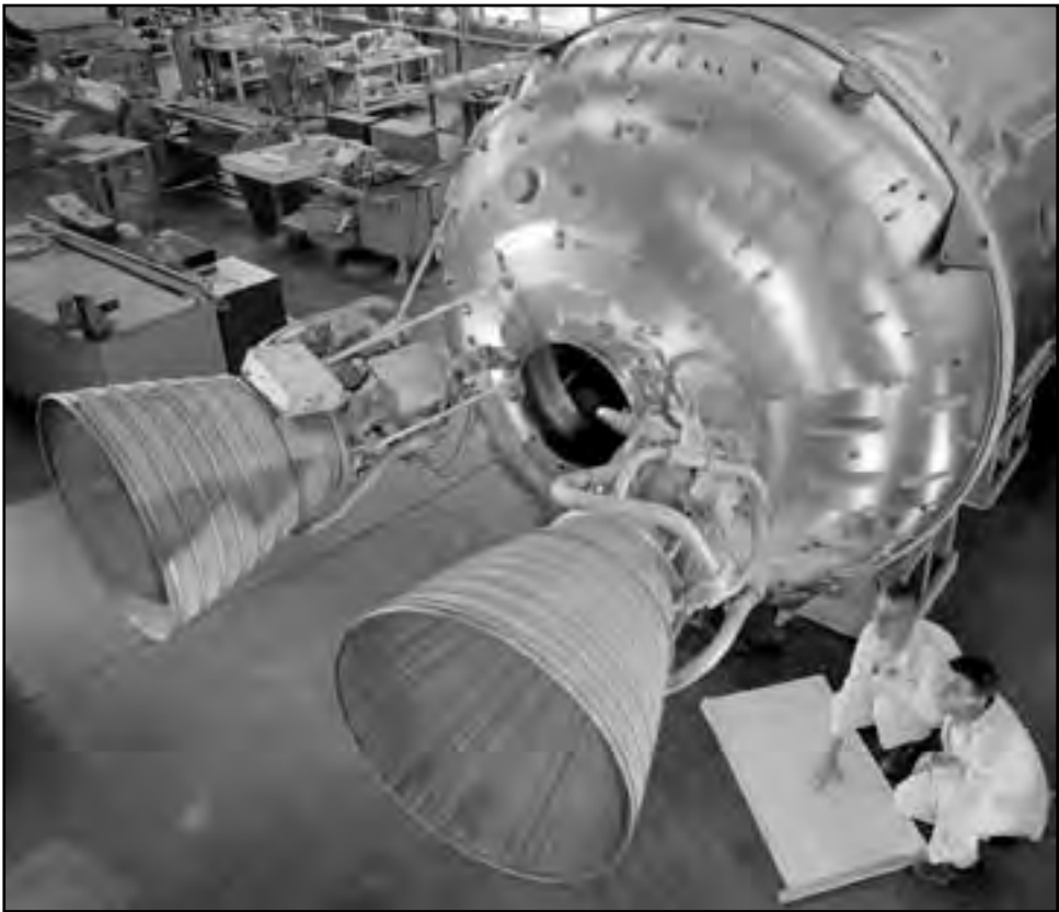
Image 205: Lewis technicians study the Centaur's RL-10 engines in the SPC shop. Centaur was the center's highest profile program, and the SPC was an important part of the program. Abe Silverstein felt, "If the space program did nothing else than to show that if you want to develop a good product for a given use, whether it be on the ground or in space, the thing you do is to design it and develop it for the environment in which it is going to live." 436 (NASA C-1964-71100)
