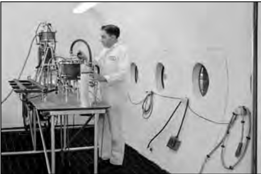
Image 177: Mercury was released into the horizontal pressurized condensing tube. Its behavior was monitored by an oscillograph and a high-speed camera on a rail that could film at any point along the tube. 376 Although the SNAP-8 program was eventually terminated, these power-conversion studies contributed to the Brayton cycle and the mercury Rankine systems of the late 1960s and early 1970s. 377 (C-1961-58584)
