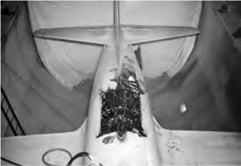
Image 106: Occasionally engines failed during tests, like the GE I-40 in this photograph. A failure could significantly damage not only the engine but also the wind tunnel. (NASA C-1945-11214)
