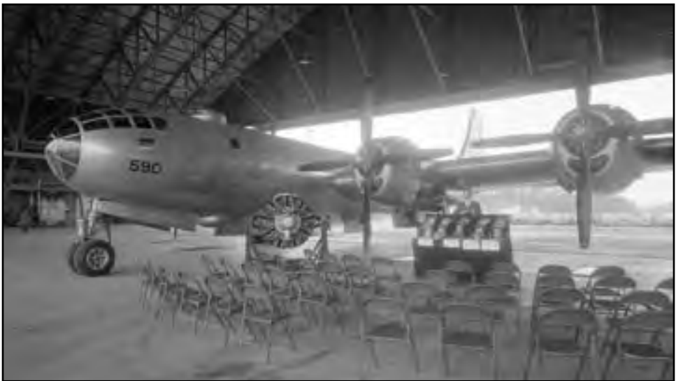
Image 56: B-29 Superfortress in the AERL hangar for a postwar open house event with its Wright R-3350 engine on display. The AERL had remedied the engine's cooling problems, but many of the modifications would not be implemented until after the war. (NASA C-1945-10587)
