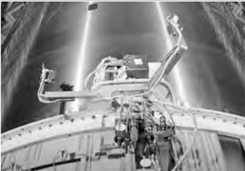
Image 214: A radiant heater system was designed specifically for the tests. Six sectors of 500-watt tungsten-iodine lamps were arranged around the rocket to simulate the effect of the Sun's heat on the electronic systems. Four of these arrays were on the upper end of the Centaur, and two arrays were located near the RL-10 engines. Certain lamps could be turned on at different times to simulate the changing direction to the Sun. 458 (NASA C-1967-00180)
