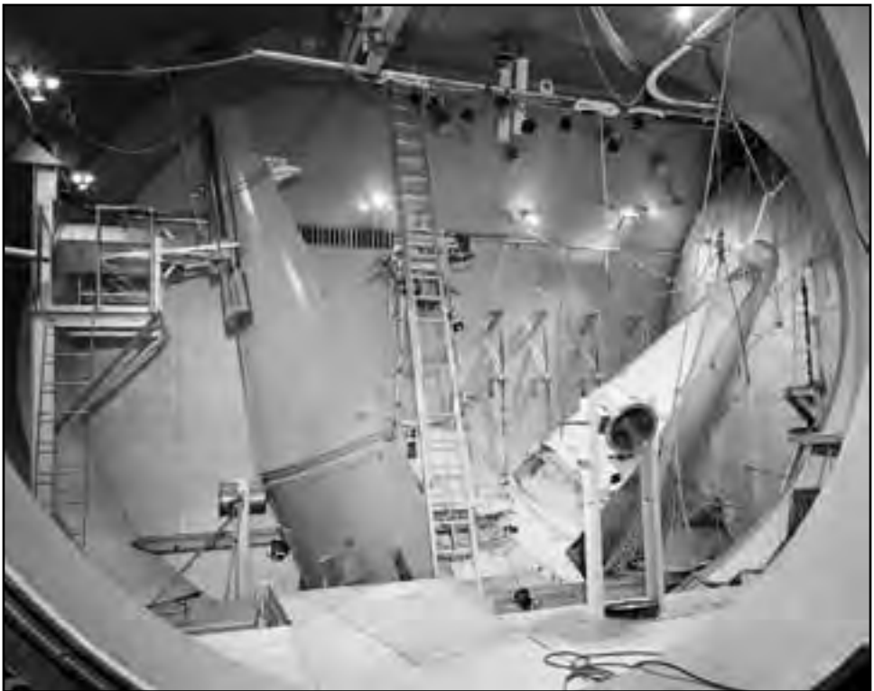
Image 225: Nose-cone separation test in SPC No. 1 for the upcoming AC-6 mission, which would place the first Surveyor model into orbit. The 2,000-pound model was used as an instrumented dynamic payload simulation. (NASA C-1965-00725)
