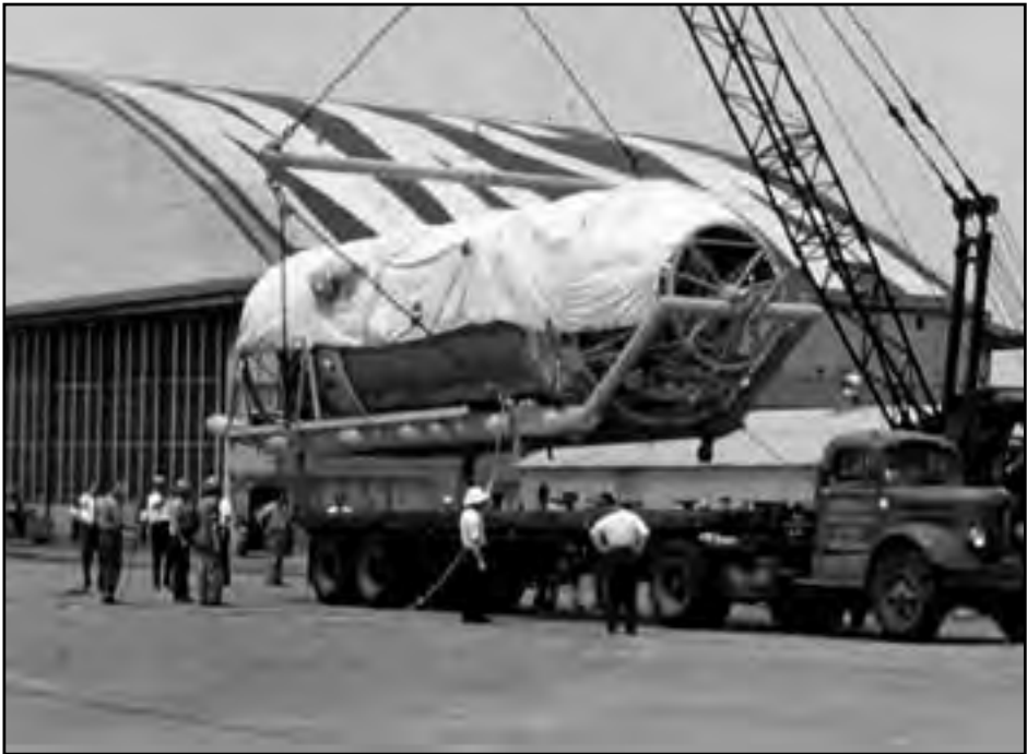
Image 203: The Centaur 6A rocket is delivered to NASA Lewis for testing in SPC No. 1. Because of its fragile structure, the Centaur had to be transported on a stretcher to make sure that it did not collapse on itself. It was flown from Cape Canaveral on a C-130 transport aircraft. ("Centaur engine arriving at Lewis aboard C-130," 27 September 1963, NASA MPD-498) (NASA Glenn film collection)
