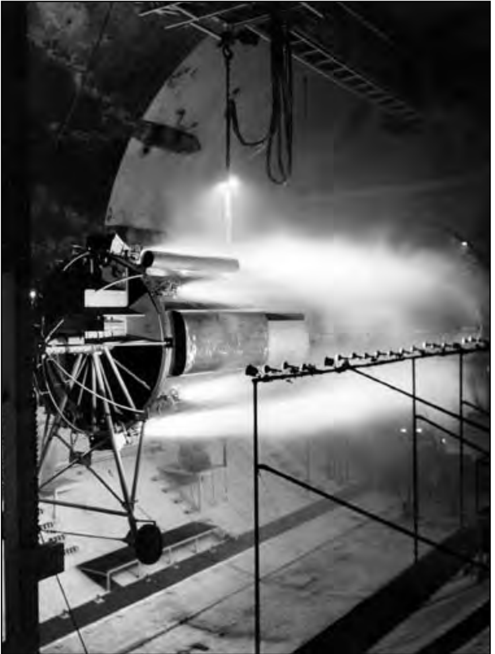
Image 194: The first study in the new Space Power Chambers used a unique model that simulated the Atlas/Centaur's size and weight to test retrorockets. During this time a full-scale Centaur rocket was being readied for testing in the facility's vacuum chamber. (NASA C-1964-69428)
