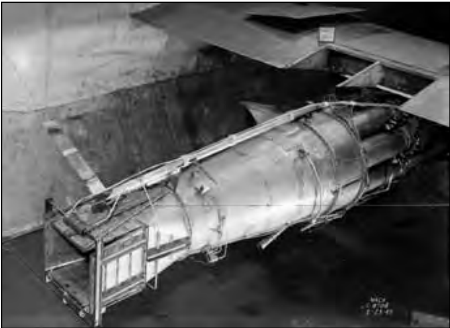
Image 71: A variable-area nozzle is installed on a GE TG-180 engine with an afterburner in the AWT. AERL created a clam-shell design because it was easier for the mechanics to build. The AERL studies led engine manufacturers to later develop an iris-type nozzle that was lighter and more efficient. 194 (NASA C-1945-8708)
