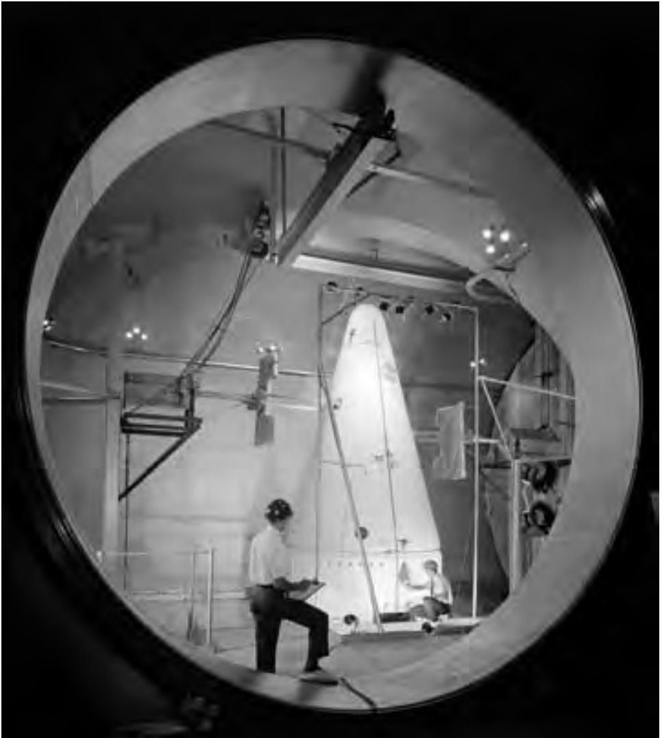
Image 220: Researchers in SPC No. 1 examine the nose cone for the Centaur/Surveyor spacecraft. (NASA G-1964-71093)
