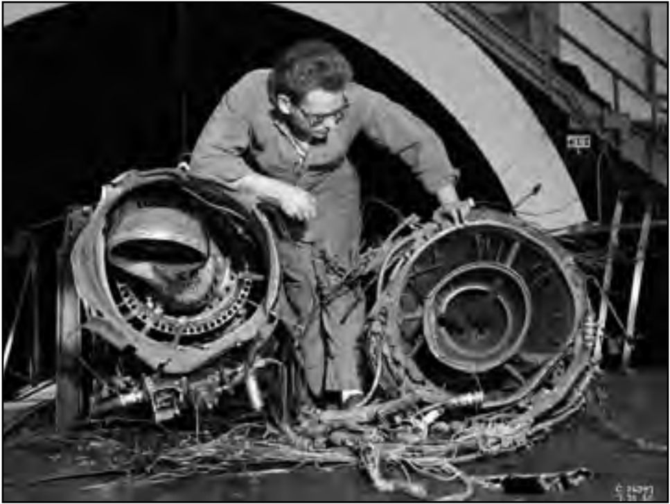
Image 123: Apprentice Dominic Giomini examines a Westinghouse 24C-7 that failed during a run in the AWT on 19 July 1950. That same day NACA Director Hugh Dryden had issued a letter proposing the acceleration of research at the lab in response to the outbreak of the Korean War three weeks before. (NASA C-1950-26297)
