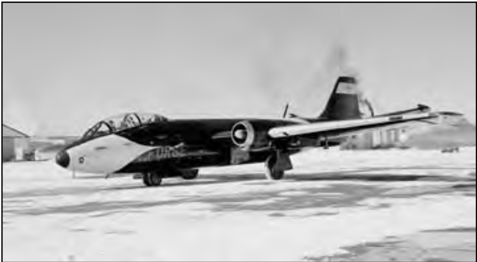
Image 142: The B-57B aircraft flew several flights in the winter of 1957 using liquid hydrogen as a propellant at cruising altitudes. The flights would be one of the first times all of the lab's research elements were incorporated into a single operating system. This photograph of the aircraft was taken one year later with the wing tanks removed. (NASA C-1958-47236)
