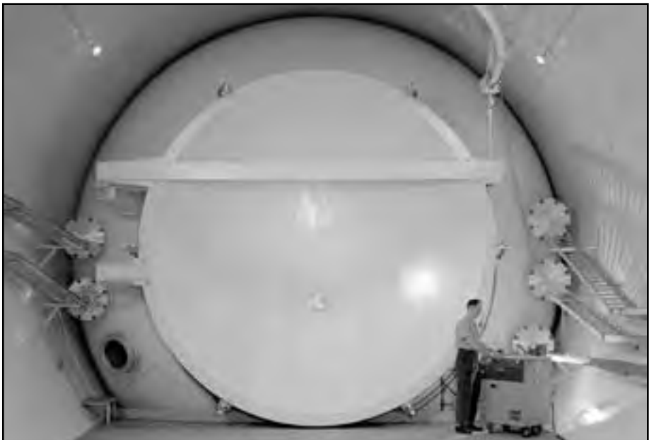
Image 189: Publicity photograph of a bulkhead in the new SPC taken two days after the Centaur F-1 explosion. Work would soon begin readying the unused facility for Centaur testing. (NASA C-1962-60341)
