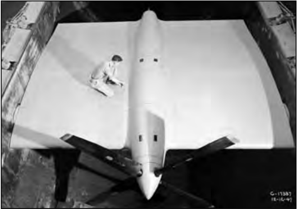
Image 117: GE's 14-stage axial-flow TG-100, the nation's first turboprop aircraft engine, underwent two months of testing in the AWT starting in late 1946. A 12-foot, 7-inch Hamilton Standard propeller was fitted to the engine. The TG-100 was run at 8,000 to 13,000 revolutions per minute (rpm) and at altitudes from 5,000 to 35,000 feet. 258 (NASA C-1946-17387)
