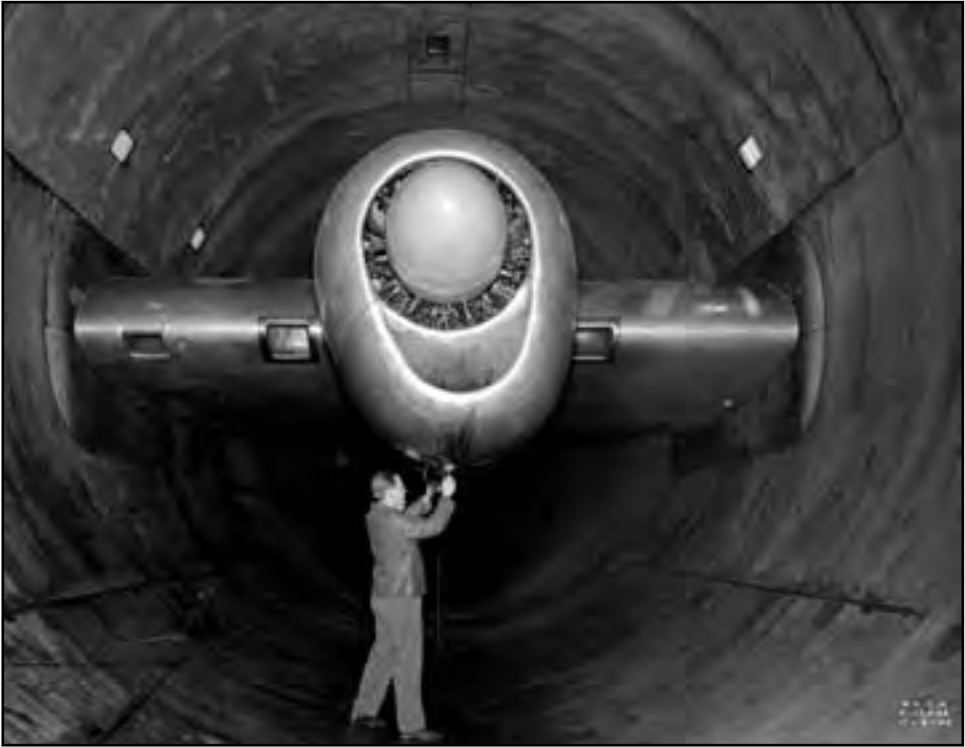
Image 73: A mechanic installs instrumentation on the Lockheed XR-60's R-4360-18 engine inside the closed AWT test section during a test for the navy. The October 1945 studies found that engine temperature did not exceed 450°F at takeoff or at cruising altitudes of 5,000, 10,000, or 15,000 feet. In this photograph, the four-bladed Curtiss propeller has been removed. (NASA C-1945-13598)
