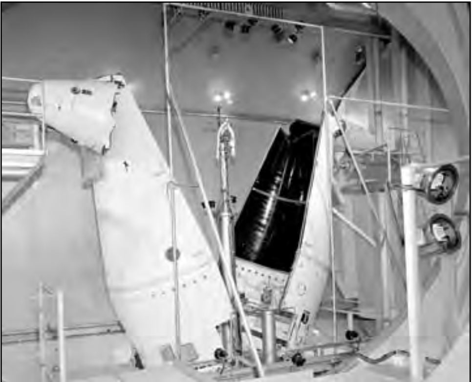
Image 219: On 5 August 1964, the first actual jettison test was run in SPC No. 1 at a pressure altitude of 70 miles. The deflector bulkheads below the payload were ripped from their bindings, and the tips of the shroud were broken off as the fairing halves slammed into the catcher pads. 465 (NASA G-1964-71125)
