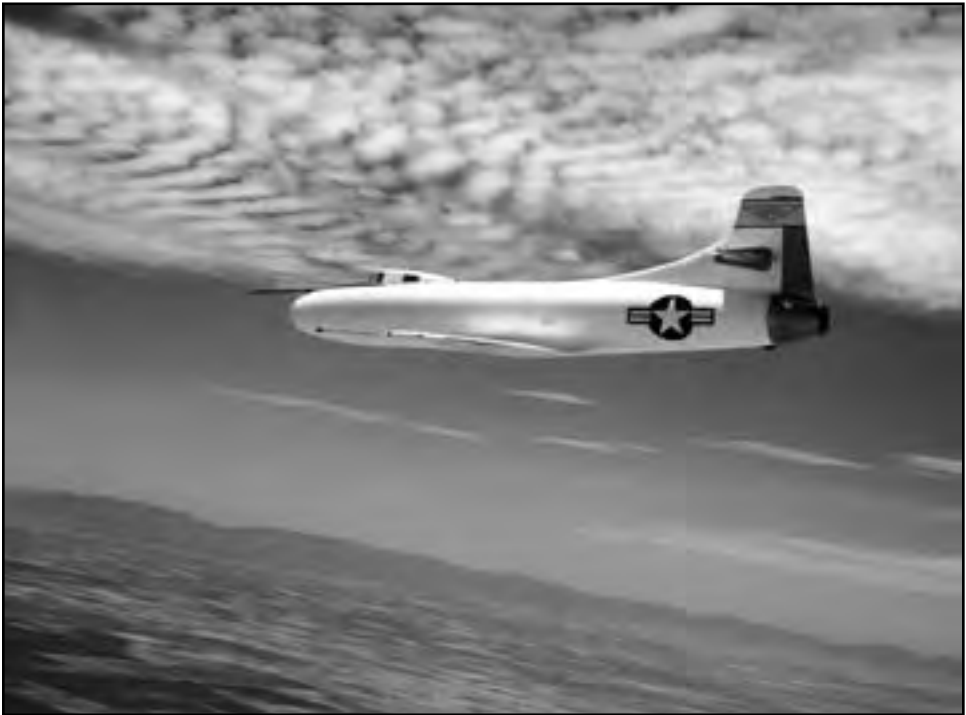
Image 65: Douglas D-558-I Skystreak powered by the TG-180 engine. On 20 August 1947 U.S. Navy Commander T. Caldwell flew the Skystreak to a new world's speed record of 640.7 mph. A second D-558-I flown by U.S. Marine Pilot Major Marion Carl soon bettered the record by 10 mph. Unlike the X-planes, the Skystreaks took off from the ground under their own power and had straight wings and tails. 178 (NASA E-713)
