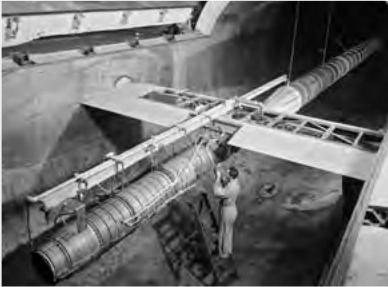
Image 91: The engine was mounted to a wing span that was fixed to trunnions on the tunnel walls. The wing was connected to the measurement devices in the balance chamber. The tunnel mechanics connected the instrumentation to data output lines, installed the fuel and oil supply lines, and hooked up the engine's operating controls. (NASA C-1946-14244)
