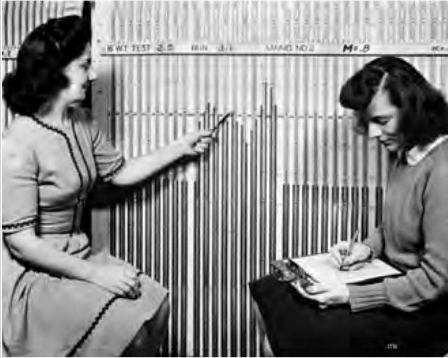
Image 107: Female computers obtained test data from the manometers and other instruments and made the computations. Analysts then converted the data into meaningful figures. The “computers” and analysts were located in the Shop and Office Building office wing until being relocated to the 8- by 6-Foot Supersonic Wind Tunnel in 1948. Al Young’s wife, Mercedes, served as the computers’ supervisor for years. (NASA C-1944-04238)
