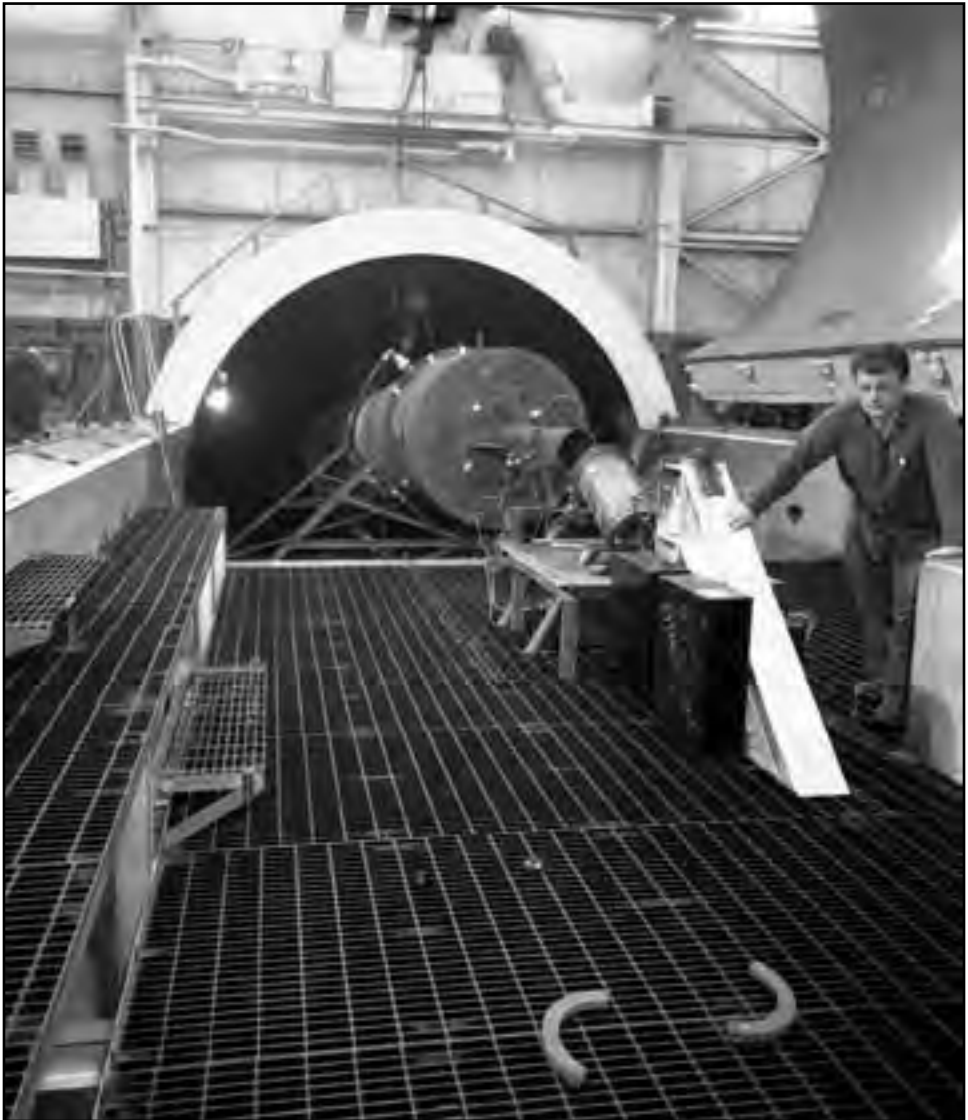
Image 148: Solid-rocket assembly damage in the AWT. Unlike the solid propellants used for typical missiles or other engines, the behavior of propellants in high-performance vehicles cannot be predicted on the basis of sea-level tests. In May 1958, Lewis researchers commenced a series of low-pressure tests in the AWT to study the behavior of the solid propellant, high-performance rocket engines with high expansion ratios. The pressure's influence on the entire chamber, the exhaust nozzle, and the rocket's specific impulse was measured. 316 (NASA C-1958-48161)
