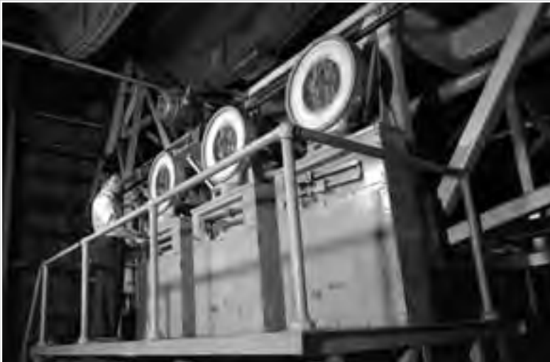
Image 92: Harold Friedman inspects the Toledo scales in the balance chamber. The balances were located in the balance chamber below the test section. Toledo scales recorded the movements of the balances caused by the engine being tested. The maximum thrust capacity was 12,000 pounds, and the maximum lift was 20,000 pounds. 233 (NASA C-1945-09635)
