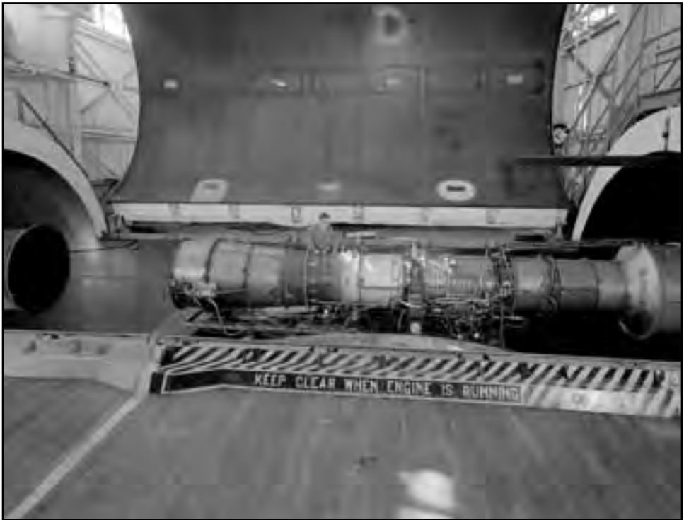
Image 131: A technician works on the 9,700-pound-thrust Allison J71-A-11 engine in the AWT test section. The 16-stage axial-flow engine was 16 feet long, 4 feet in diameter, and weighed 4,450 pounds. The J71 replaced Westinghouse's J40 on several navy fighters. (NASA C-1955-39623)
