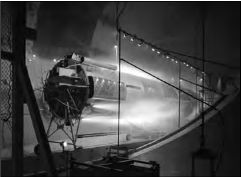
Image 198: The Atlas portion of the model separates from the simulated Centaur. Following the initial findings in late 1963, Rocket Power, Inc., developed its own improved igniter. The system was again tested during the spring of 1964 in SPC No. 2. The extended-burn igniters used an initiator and fired electronically. Propellant granules used in the sustainer charge improved the heat input by providing hot gases to the grain. The researchers found that the newly designed igniter fired properly using any closure thickness. 426 (NASA C-1964-68534)
