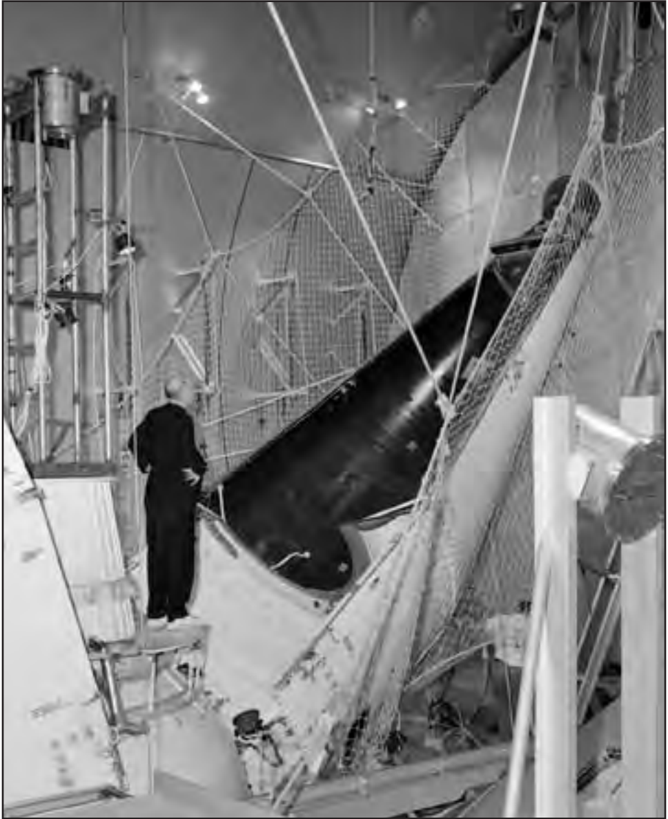
Image 222: Jack Humphrey, project manager for the Surveyor nose-cone tests, inspects half of the jettisoned shroud inside SPC No. 1 in 1964. Humphrey had been at the center since 1943. He and his team had determined that the new design had enough clearance between the deflector bulkhead and the packages. (NASA C-1964-73201)
