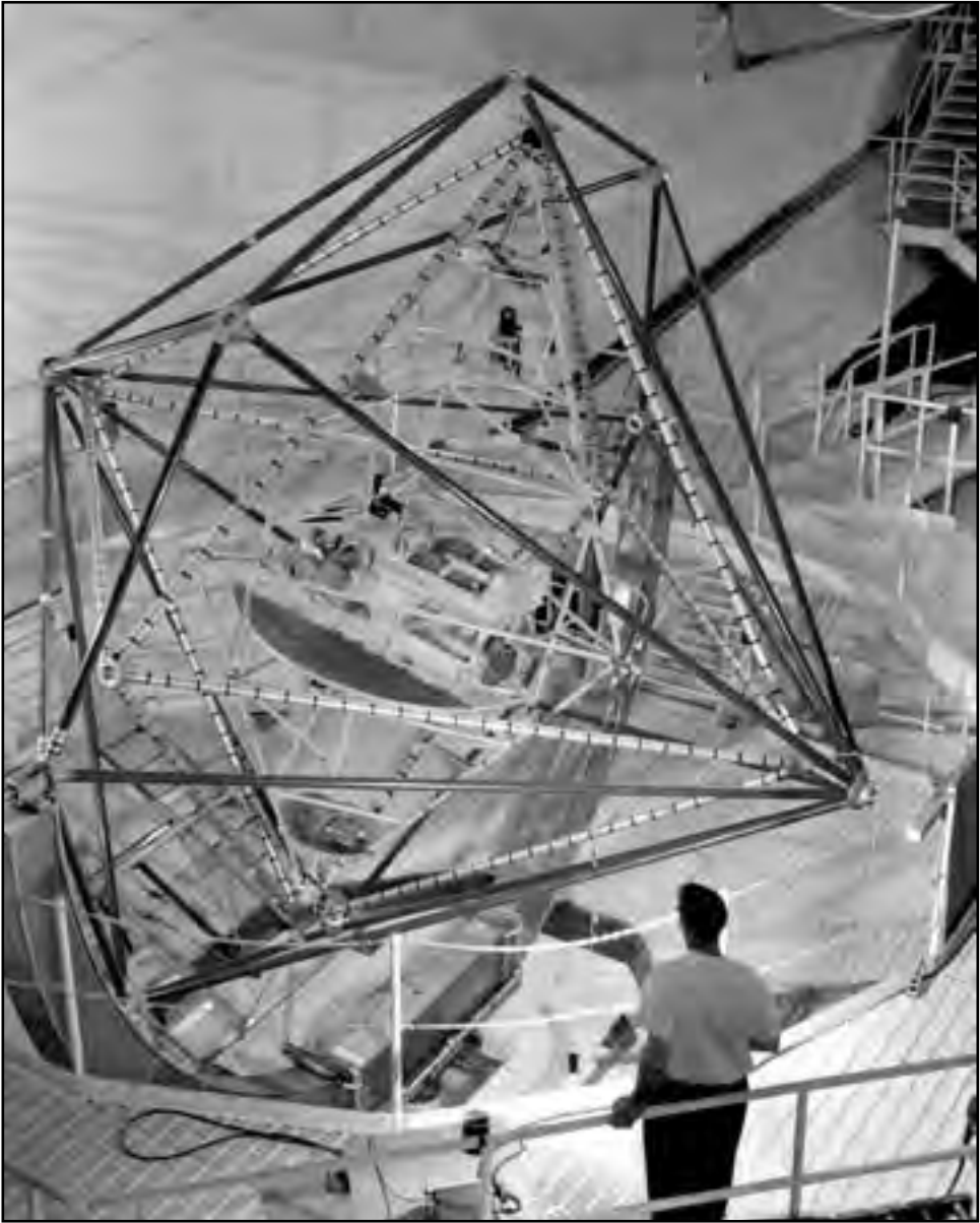
Image 159: The MASTIF, a three-axis rig with a pilot's chair mounted in the center, was installed in the AWT to train Project Mercury pilots to bring a spinning spacecraft under control. After being secured in a foam couch in the center of the rig, an astronaut would use small nitrogen gas thrusters to bring the MASTIF under control. There was an incident during which one of the valves was opened and the empty rig spun wildly until it fell apart. The MASTIF was reassembled using the spare set of parts, although a different style of mounting had to be designed. 345 (NASA C-1959-51723)
