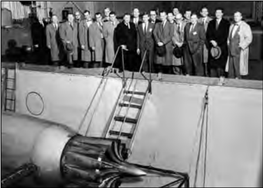
Image 143: The NACA Special Subcommittee on Aircraft Noise, chaired by William Littlewood, views a Pratt & Whitney J57 engine with a Greatex No. 2 exhaust nozzle in the AWT test section. The engine was tested with various nozzles as part of a noise-reduction study in the tunnel from January to May 1957. (NASA C-1957-44377)
