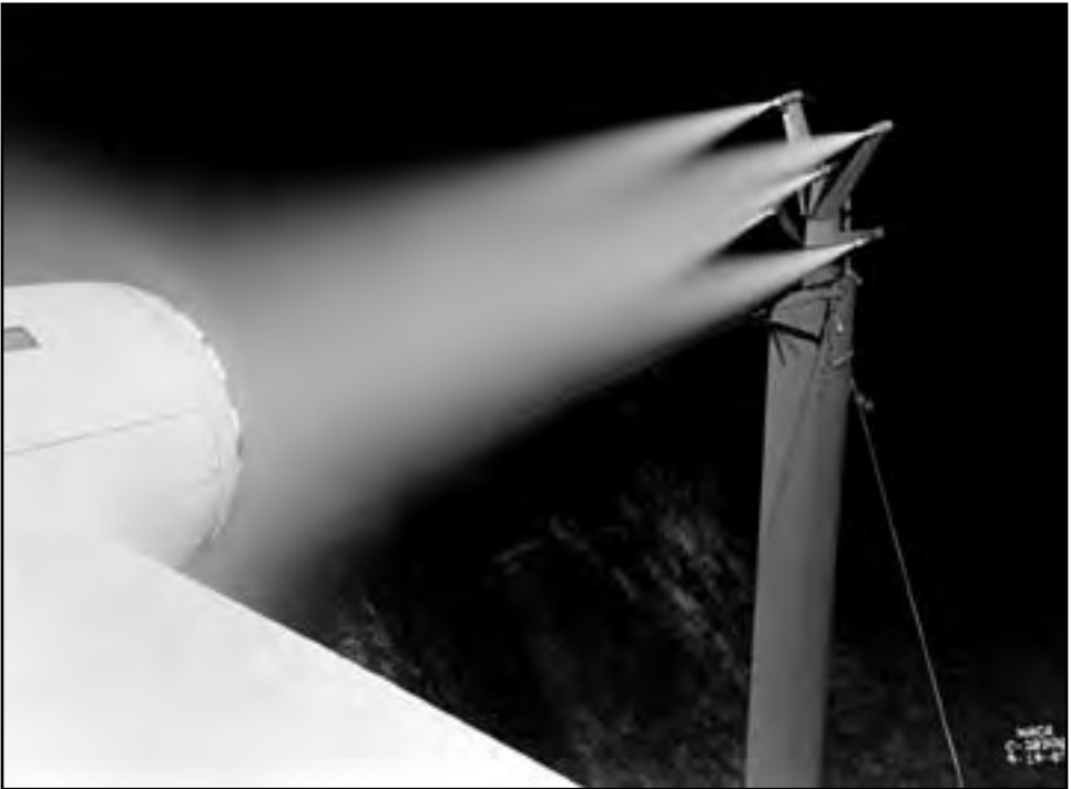
Image 113: A jet engine ice-protection system for the Westinghouse 24C-4B was studied at altitudes from 5,000 to 20,000 feet over a range of speeds in the AWT. Since icing tests were not usually conducted in the tunnel, this five-nozzle spray tower was installed just upstream from the inlet. The spray system turned out to be inadequate, so future hot-gas bleed tests were conducted in the Icing Research Tunnel. (NASA C-1947-18308)
