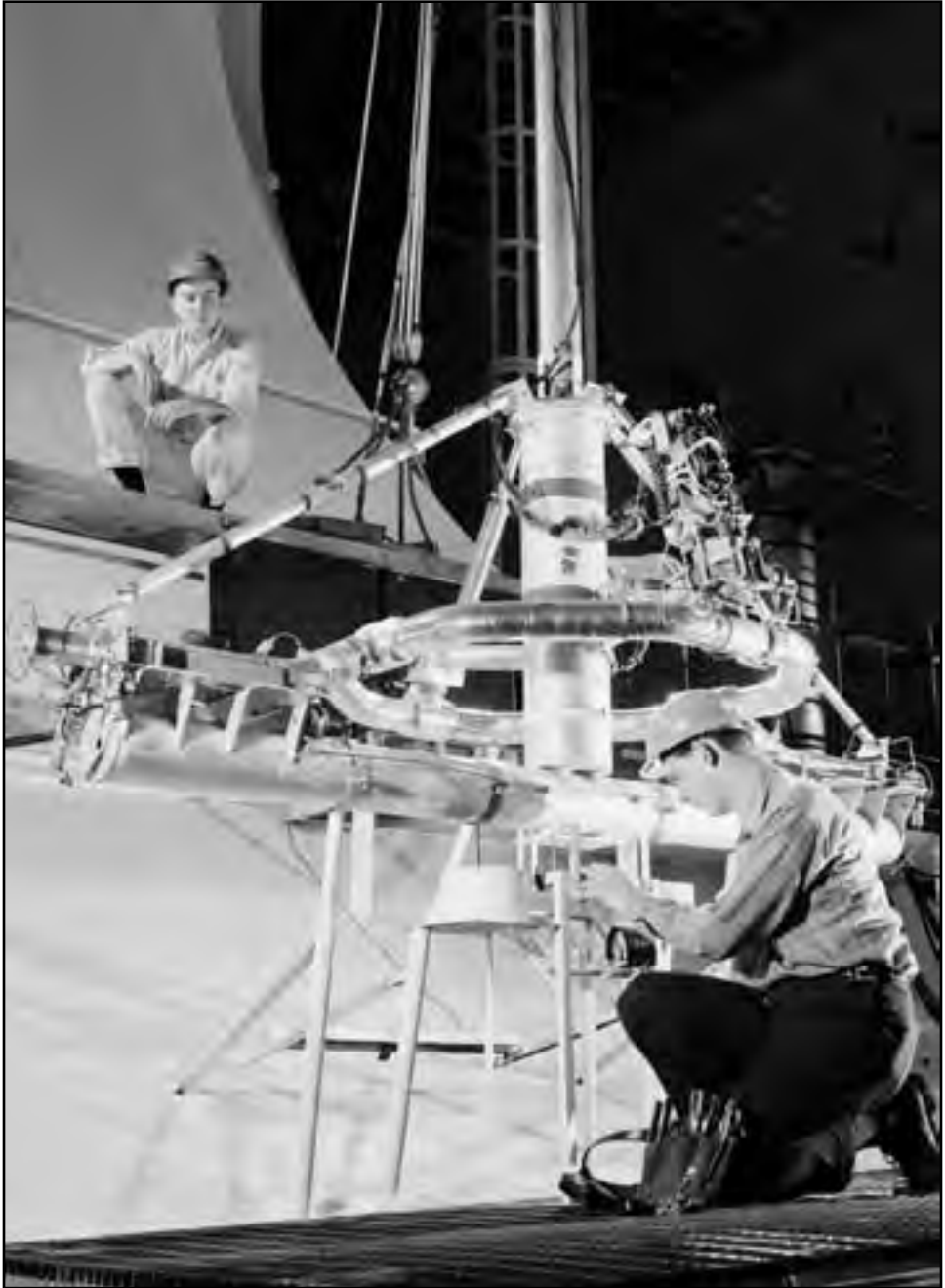
Image 230: Setup for qualification tests of the new hydrogen venting system in SPC No. 2 prior to the AC-8 mission. The hydrogen gases were drawn up into a small chamber, which then discharged through symmetrical vents. The nozzles were installed away from the spacecraft to dampen their flow effects. Shields were placed below the inlet to keep the vent lines free of liquid hydrogen. 492 (NASA C-1965-03932)
