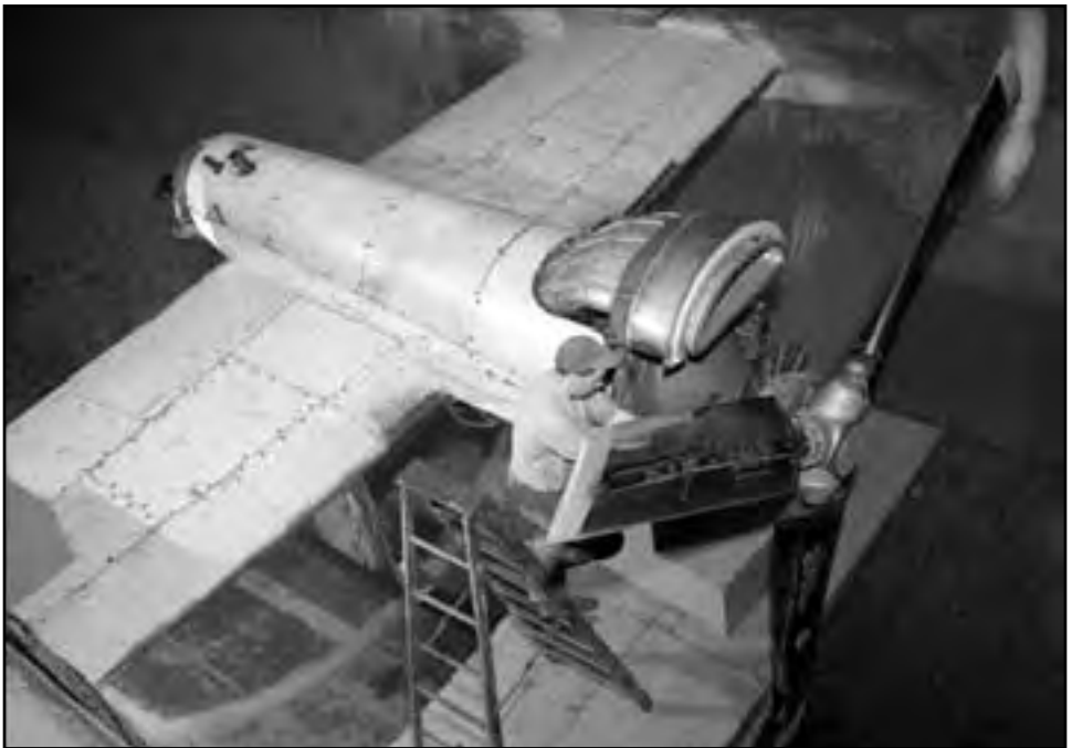
Image 134: The Allison T-38 turboprop was tested in the AWT from March to November 1953. (NASA C-1953-33216)
