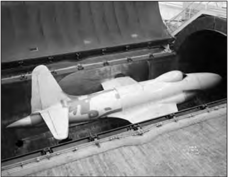
Image 58: GE I-40 engines for Lockheed's YP-80A Shooting Star were tested in the AWT from March to May 1945. The tunnel's 20-foot-diameter test section allowed the entire fuselage to be installed. (NASA C-1945-09576)
