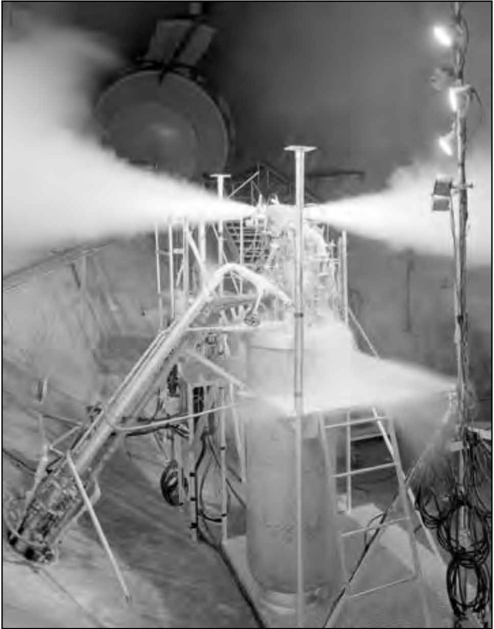
Image 229: Centaur's cryogenic liquid-hydrogen system is tested in SPC No. 2 prior to the AC-4 mission. The cryogenic liquid hydrogen used by Centaur had a boiling point of -423^{\circ}\text{F} . During the Centaur's coast period, some of the fuel would vaporize and would have to be expelled via vents. The AC-4 system contained a venturi pump that measured the gaseous hydrogen flow from the tank through the standpipe. The pressure level was controlled by a vent valve. After the nose cone was ejected, the gas could be vented through pressure-filled exits. (NASA C-1964-72930)
