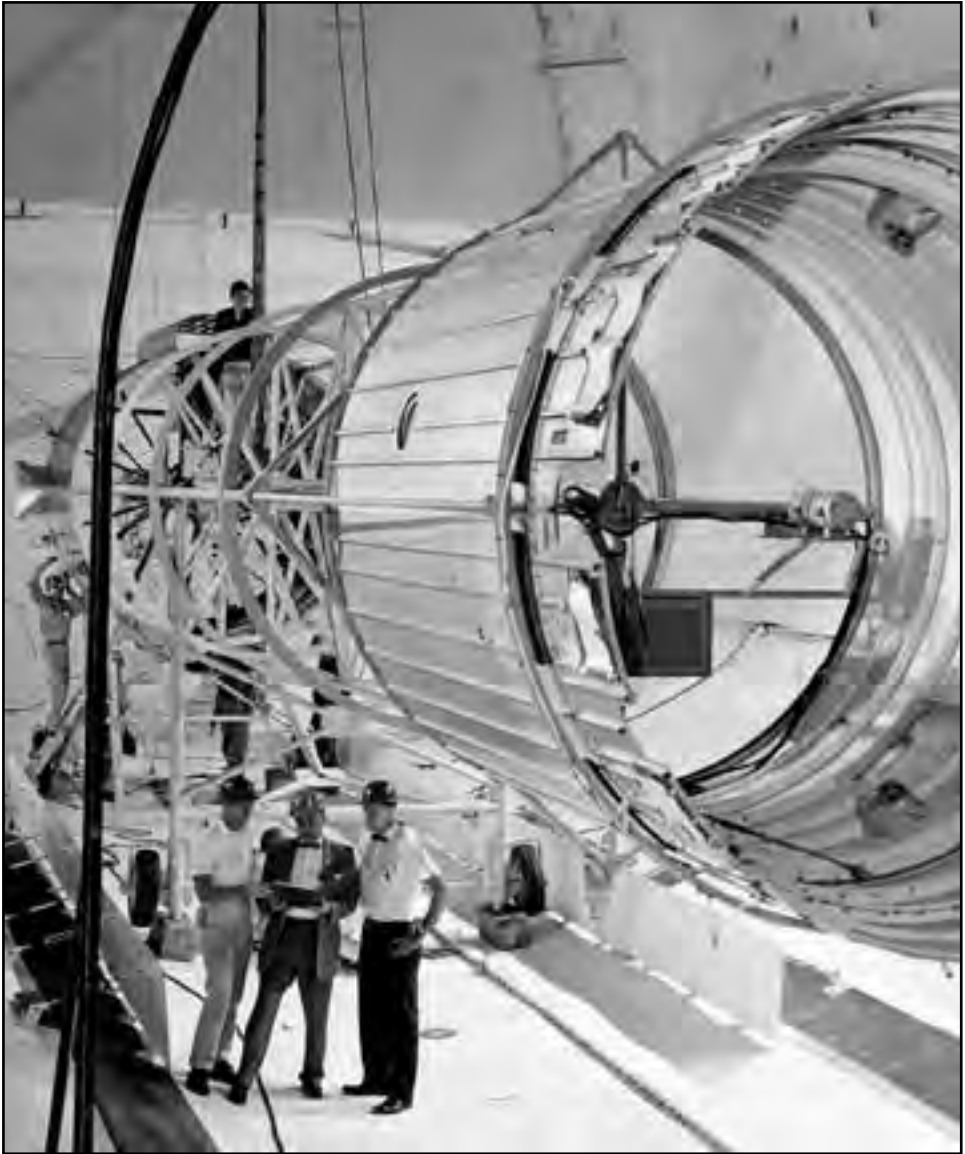
Image 201: Center; Lewis researcher Henry Synor goes over the Atlas/Centaur test setup with General Dynamics technicians inside SPC No. 2. (NASA C-1963-65906)
