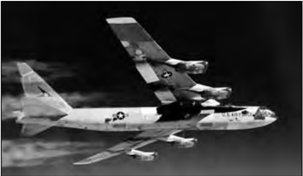
Image 137: NASA's NB-52A with an X-15 underneath its wing. The B-52 was designed by Boeing in the late 1940s as a successor to the B-47 bomber and remains an important U.S. strategic bomber. Despite the design similarities, the B-52, powered by four pairs of Pratt & Whitney J57 engines, was a much heavier and faster aircraft. In early 1951, the Air Materiel Command requested the production of 13 B-52As, but in June 1952, 10 of the orders were changed to an updated version, the B-52B. One of the three B-52As, renamed the "NB-52A," became the mothership for the NACA's X-15 program. (1960) (NASA E-88-0180-4)
