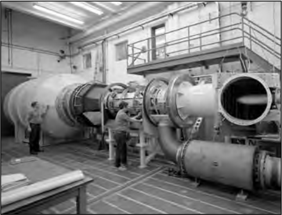
Image 263: AWT model assembly in cell CW-22 of the Engine Research Building. The model included the high-speed test section near the middle and a corner with a turning vane at the right. (NASA C-1985-02361)
