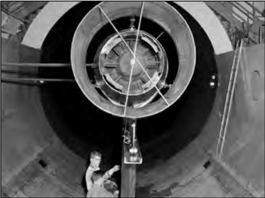
Image 145: A J57 engine is tested with a Coanda nozzle and ejector for a noise-reduction study conducted in the AWT. As the engine exhaust roared through the ejector it pulled low-speed air from the ejector pump with it. This reduced the shock and resulting noise as the exhaust hit the atmosphere. (NASA C-1957-44771)
