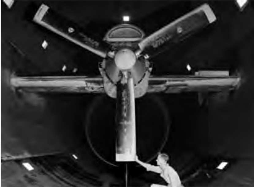
Image 103: The engine was operated and tested inside the 20-foot-diameter test section. There were numerous viewing windows in both the lid and the bottom of the tunnel. (NASA C-1953-33230)
