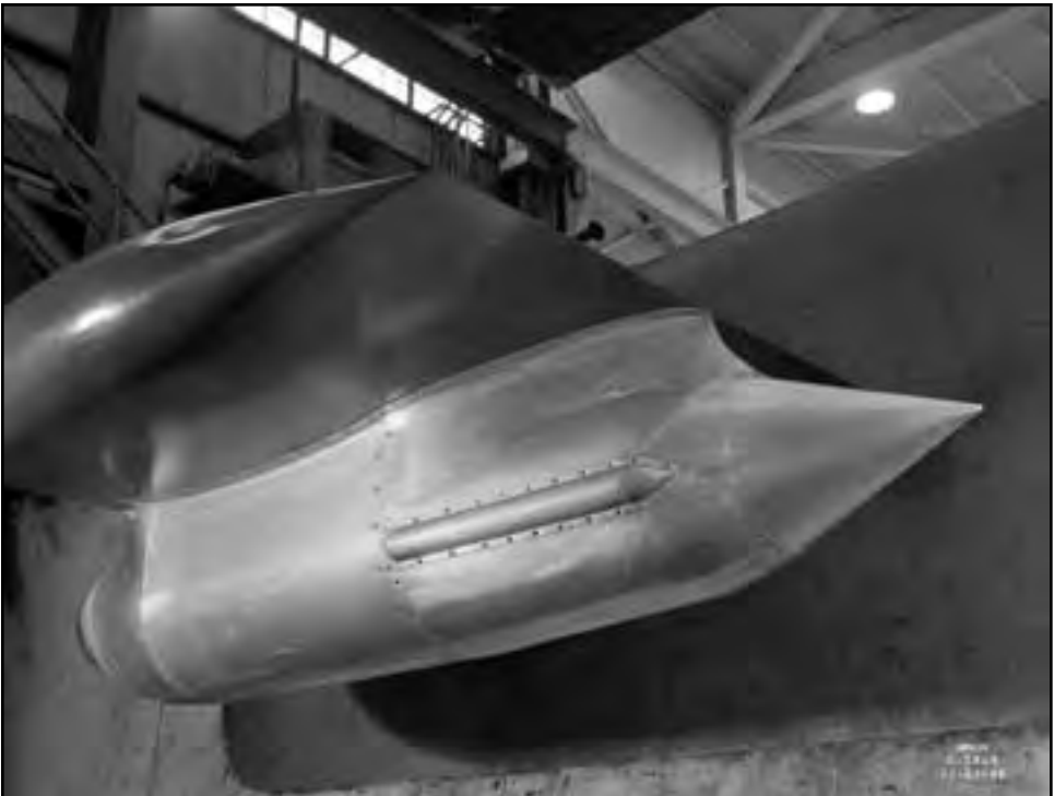
Image 63: The Westinghouse 19XB seen from the side in the AWT. Two 19XBs arrived on 6 November 1944 and were promptly installed in the tunnel. The 19XB-1 and 19XB-2B produced 1,400 and 1,600 pounds of thrust, respectively. The AWT tests revealed the superiority of the 19XB over the 19B and led to its success. (NASA C-1944-07564)
