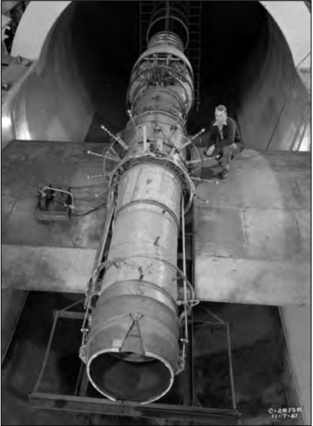
Image 121: Westinghouse's 25-foot-long, 11-stage axial-flow-compressor J40 turbojet underwent an 11-month period of study in the AWT. The AWT was upgraded in 1952 to handle these newer, more powerful jet engines. (NASA C-1951-28738)
