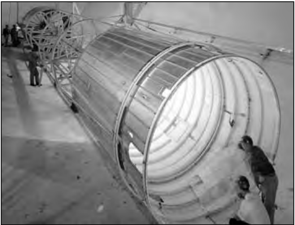
Image 196: Lewis personnel check out the Atlas/Centaur mass model inside SPC No. 2 on August 1963. The model, delivered the previous day on a small convoy of trailers, was promptly inserted into the chamber to begin setup for the separation system tests. Workers were continuing to assemble the dome on SPC No. 1 at the other end of the facility. (NASA C-1963-65614)
