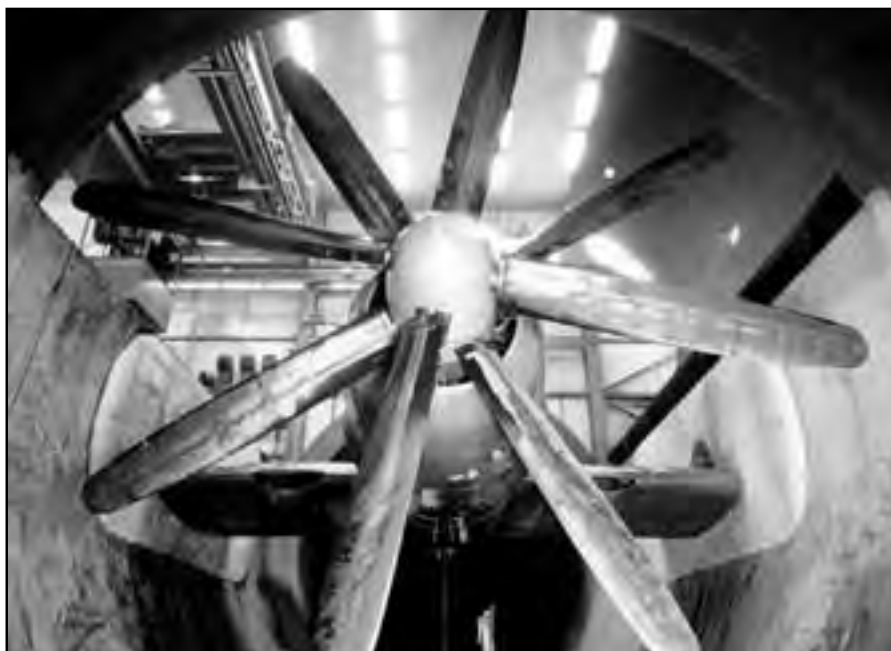
Image 72: The Douglas XTB2D-1 Skypirate, an experimental torpedo bomber powered by the Pratt & Whitney R-4360 Wasp Major engine. The XTB2D-1 was too large to be used on pre-Midway carriers, and multiseat torpedo bombers were falling from favor by the time that the Midway carriers were put into action in late 1945. Carburetor air scoops and the effect of the R-4360's long propellers were investigated in the AWT in November and December 1944. 197 The propeller caused low-pressure recoveries in the engine inlet, particularly at high angles of attack. 198 (NASA C-1944-08060)
