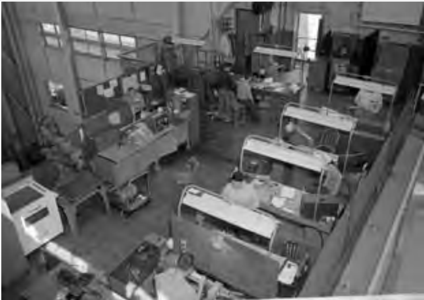
Image 239: The viewing platform alongside the former tunnel test section was converted into a shop area. The high bay is to the left of the platform, and the test section is to the right. (NASA C-1965-00378)
