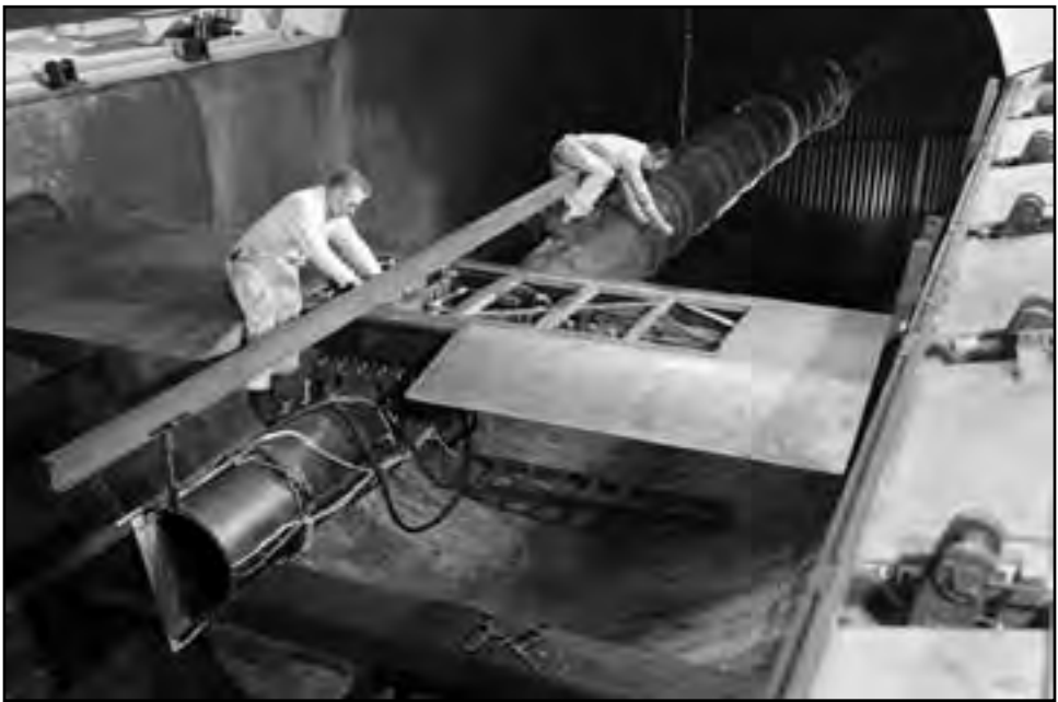
Image 82: Mechanics working on the 20-inch NACA ramjet in the AWT test section. Referring to the ramjet tests in the AWT, Bill Harrison said, "Back in those days, about the only tool you needed was an inch and a quarter wrench to take the copper tubing apart. All this was, was a pipe with angle irons and fuel injectors." 223 The tunnel's refrigerated airflow was ducted directly into the ramjet's inlet (as seen in this photograph) to create the desired speed, static pressure, and temperature to simulate high-speed flight. The tunnel was used to analyze the ramjet's overall performance up to altitudes of 47,000 feet and speeds to Mach 1.84. 224 (NASA C-1946-14733)
