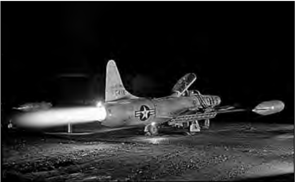
Image 69: Republic F-94 interceptor tests its afterburner prior to takeoff during the Korean War. The AWT was used to systematically study afterburner configurations on several early jet engines. Desired elements included maximum thrust, maximum operable range, high combustion efficiency, minimum weight, minimum size, low internal pressure losses, adequate cooling, and good control. 187 (27 July 1953) (National Archives)
