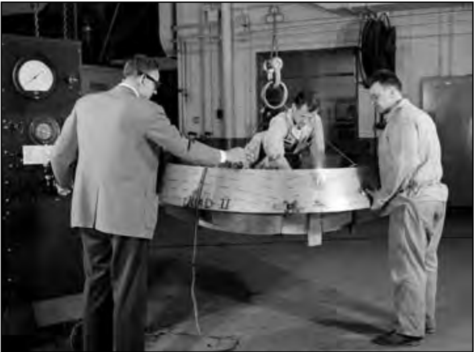
Image 154: Installation of the attitude control system for the Big Joe capsule in the AWT shop area. Robert Miller (on the left), Lou Corpas, Frank Stenger, and Phil Ross created the MASTIF test rig, which was based on a design by Harold Gold and Edward Otto. The upper portion of this piece contained the control system; gyros, thrusters, nitrogen tanks, and electronics were located in the lower section. (NASA C-1959-50457)
