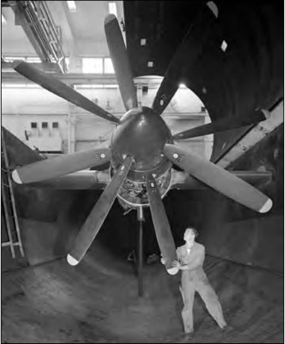
Image 119: In response to a request from the NACA, Britain supplied an Armstrong-Siddeley contrarotating turboprop engine to study in the AWT. The tests ran from July 1949 through January 1950; it was the first time that the tunnel had been used to study an engine with the sole purpose of learning about, not improving, the engine. (NASA C-1949-23957)
