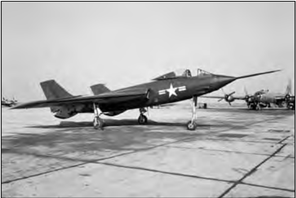
Image 114: The Vought Cutlass was powered by two Westinghouse J34-WE-32 (24C) engines. In 1945 the navy had requested that a new fighter jet be designed around the 24C engines. The Cutlass was the first tailless military fighter, the navy's first swept-wing aircraft, and the first production aircraft to use afterburners. The first Cutlass is seen here at the NACA Langley Aeronautical Laboratory in December 1948. In just over a year, these engines would undergo a thorough investigation in the AWT. (NASA EL-2000-00267)
