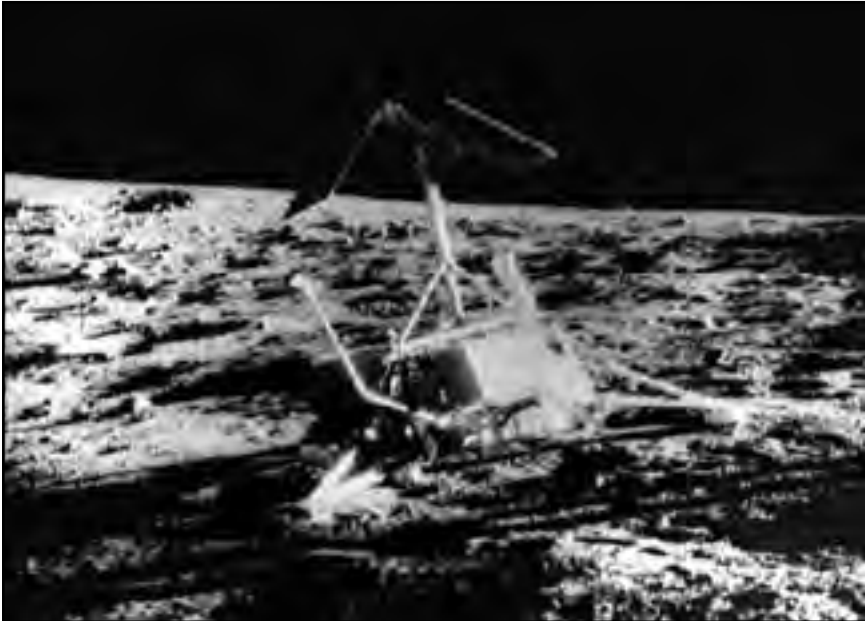
Image 209: The Surveyor landing vehicle was basically a large tripod with 4.3-meter legs. Different equipment packages were used for the various missions. The early missions contained only cameras, whereas the later spacecraft also included excavating equipment. The Surveyor III spacecraft shown here landed on the lunar surface on 20 April 1967. In this photograph, which was taken in November 1969 by the Apollo 12 crew, a 1-meter mast with a solar cell panel rises above the base. 453 (NASA AS12-48-7121)
