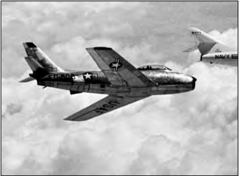
Image 122: The swept-wing F-86A Sabre became the preeminent fighter of the Korean War. It was powered by the General Electric J47-GE-13 (TG-190), which had undergone intensive studies in the AWT during the late 1940s. The Sabre could reach an altitude of 49,000 feet and speeds of 685 mph, and it had a 10-to-1 kill advantage over the Russian MiG-15. 278 (1955) (NASA E-3996)
