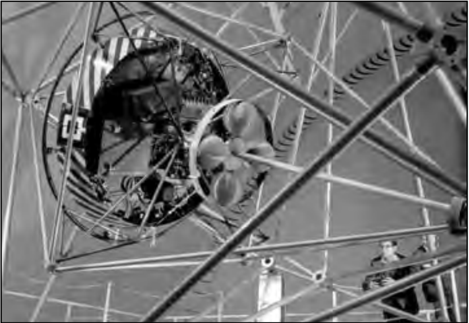
Image 155: NASA Lewis researcher William Masica operates the MASTIF. The Big Joe navigation system package is mounted in the center of three cages, which each spin in a different direction. Mounts for the tunnel's turning vanes, which had been removed prior to these tests, can be seen in the background along the ceiling. (NASA C-1959-51728)
