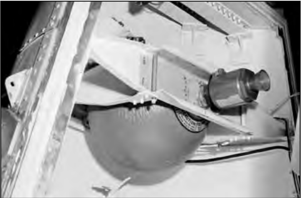
Image 221: Nitrogen bottle, thruster, and attachment plate in the tip of the Centaur/Surveyor nose cone. This thruster fired as the explosive bolts securing the fairing were released, thus pushing the 1,000-pound fairing halves away from one another and the Centaur. (NASA G-1965-00604)
