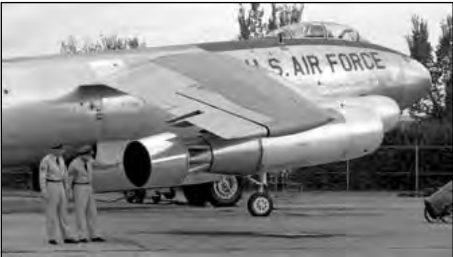
Image 146: A B-47 bomber on display at the NACA Lewis 1957 Inspection. One of its GE TG-190 (J47) engines has a noise-reducing ejector installed on its exhaust. The ejector was developed at Lewis and tested on a Pratt & Whitney J57 in the AWT. (NASA C-1957-46143)
