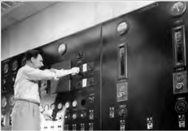
Image 94: To start a test, a tunnel operator would activate the tunnel's drive motor, refrigeration system, and exhausters from inside the AWT control room. The operator worked in coordination with colleagues in the Engine Research, Exhauster, and Refrigeration buildings. (NASA C-1945-10346)
