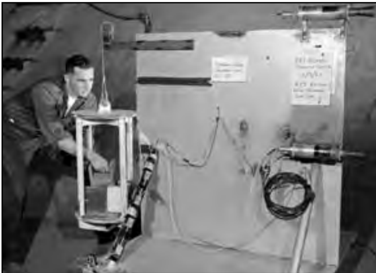
Image 200: The retrorockets were tested with their igniters packed with various forms of boron potassium nitrate. The igniters failed six times during their 67 firings. Researchers also used foam panels to record the flame patterns and found a wide range of disbursement among the various igniters. A new igniter, which directed its flame directly at the propellant and burned for a longer duration, was selected. 428 (NASA C-1964-70158)
