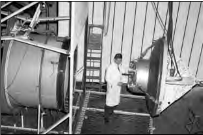
Image 168: Mercury capsule/Redstone separation test in the AWT. The postgrade rockets were fired, and the capsule jettisoned forward on a tether. High-speed film was used to analyze the separations. A plywood shield was hung guillotine-style above the ring. Once the bolts blew and the capsule shot out, the plywood dropped down to protect the booster model when the capsule swung back on its pendulum. 363 (NASA C-1960-52778)
