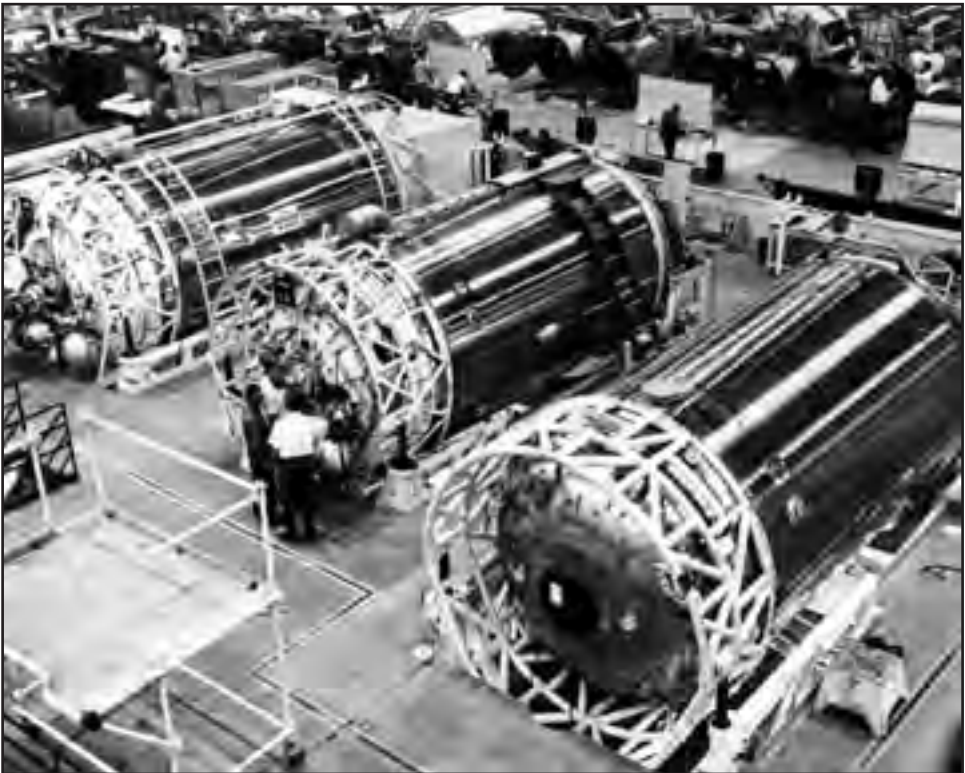
Image 190: Centaur rockets in the General Dynamics assembly plant. General Dynamics had devised a new type of spacecraft that initially possessed a number of difficulties. It was the first cryogenic stage ever attempted, it would restart its engines in space, its tanks were balloons that had to remain pressurized, and there was a bulkhead the thickness of only a couple layers of aluminum foil between the oxidizer and propellant. (NASA C-1962-62408)
