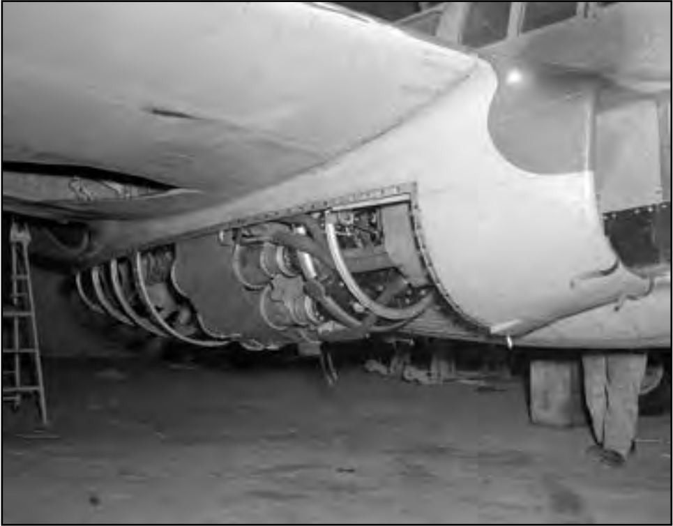
Image 49: The Bell YP-59A Airacomets with nacelle cover removed to reveal one of its two GE I-16 jet engines. GE's West Lynn plant had developed the turbocharger, which increased the capabilities of piston engines and allowed the first over-weather flight in July 1937. Because of the demand for the turbochargers, the West Lynn plant expanded its facilities and began working closely with the air corps. This relationship led to its selection to build the nation's first jet engine, the I-A. Turbocharger guru Sanford Moss was called out of retirement in 1943 to assist with the next generation of centrifugal jets—the I-14, I-16, and I-20. 139 (NASA C-1945-10686)
