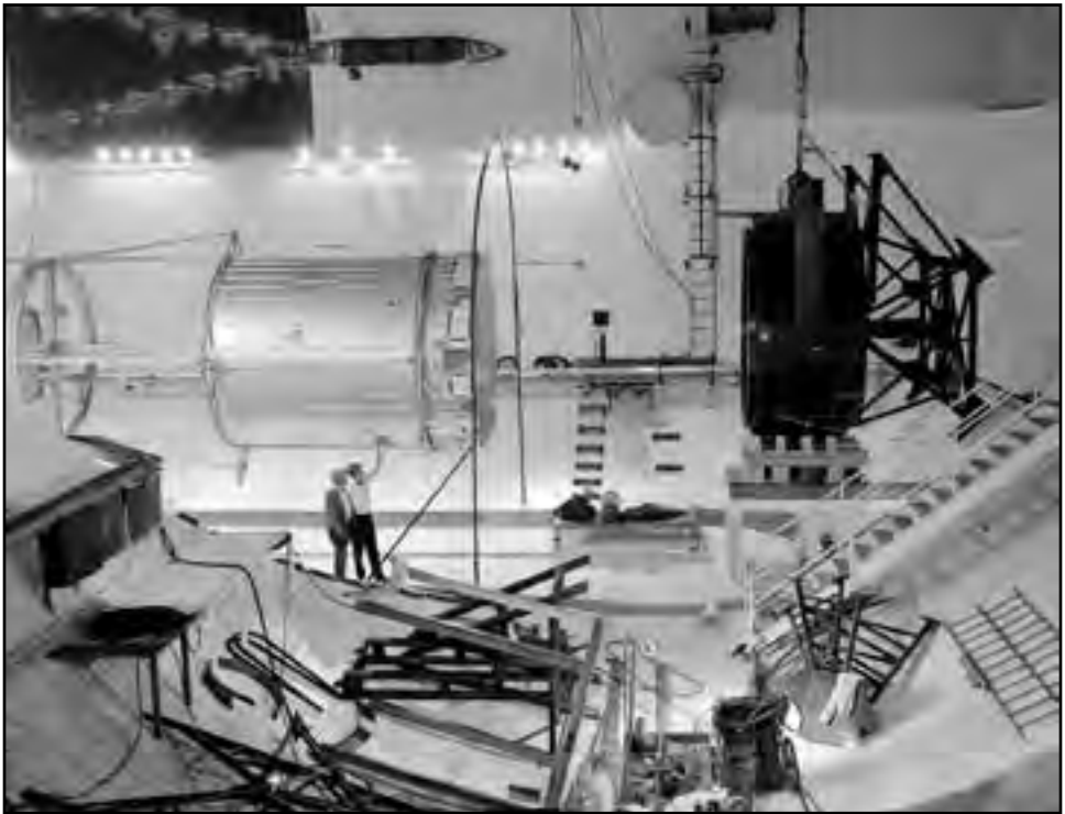
Image 197: Atlas/Centaur mass model suspended from the trolley system inside SPC No. 2. The dark section to the right is the fixed Centaur model. The corrugated section above the researchers is the interstage adapter that was jettisoned from the Centaur using linear-shaped charges. The long cagelike Atlas portion of the model begins just to the left of the adapter and continues out of view to the left. Eight retrorockets were used to push this section away from the Centaur. 424 (NASA C-1963-65907)
