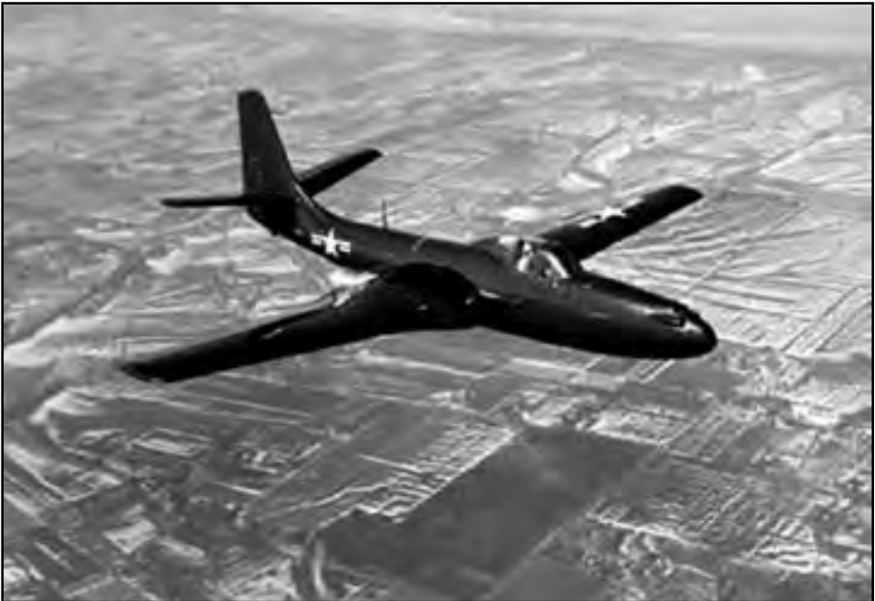
Image 64: The McDonnell Phantom XFD-1 became the U.S. Navy's first completely jet-propelled aircraft. Its development began in August 1943. The Phantom was originally designed to use two Westinghouse 19B jet engines. After successful tests in the AWT, these were replaced by 19XBs. The 19XBs were also used for the experimental Douglas XB-42A Mixmaster and the Northrop XP-79 "flying wing" aircraft. (U.S. Navy/Department of Defense)
