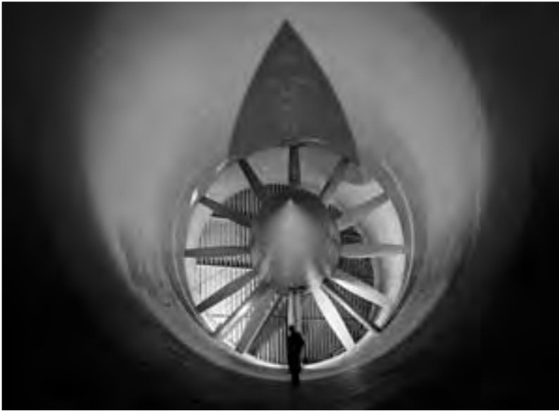
Image 97: The 31-foot-diameter, 12-bladed spruce fan in the southeast corner of the tunnel could generate wind speeds up to 500 mph depending on the pressure levels. The large tail fairing at the center of the fan helped to even the airflow. (NASA C-1944-03993)
