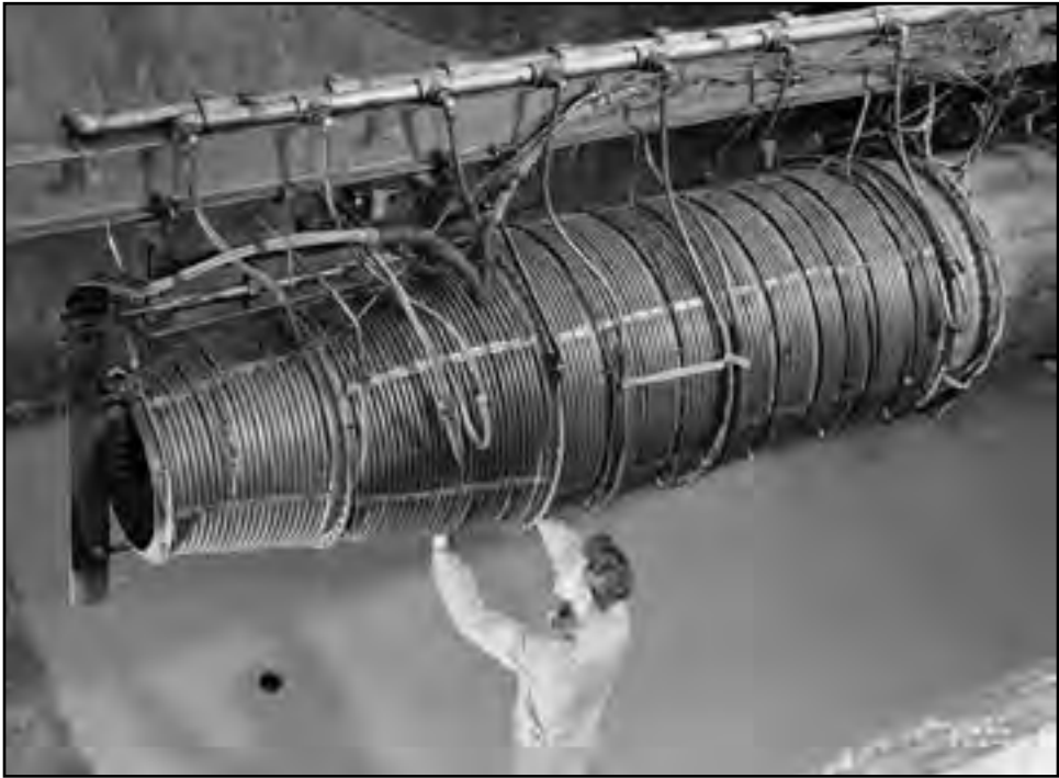
Image 70: A technician adjusts the large afterburner on a GE TG-180 engine in the AWT test section. The 29-inch diameter of the burner resulted in a low-velocity, but highly efficient, thrust. The three main sections of tailpipe burners are the diffuser section, the combustion chamber, and nozzle section. The engine underwent thrust augmentation tests in the tunnel using a variety of tailpipe burners. (NASA C-1946-14938)
