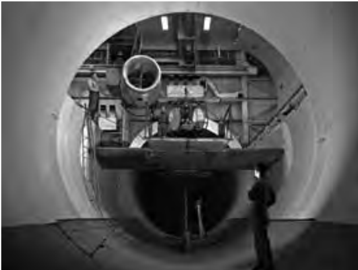
Image 90: Upon completion of the previous test, the engine was removed. The next engine was lifted by an overhead crane and transported from the shop, up into the second story test chamber room, and finally into the 20-foot-diameter test section. The crane ran along the high bay from the shop to the test chamber. (NASA C-1951-28463)
