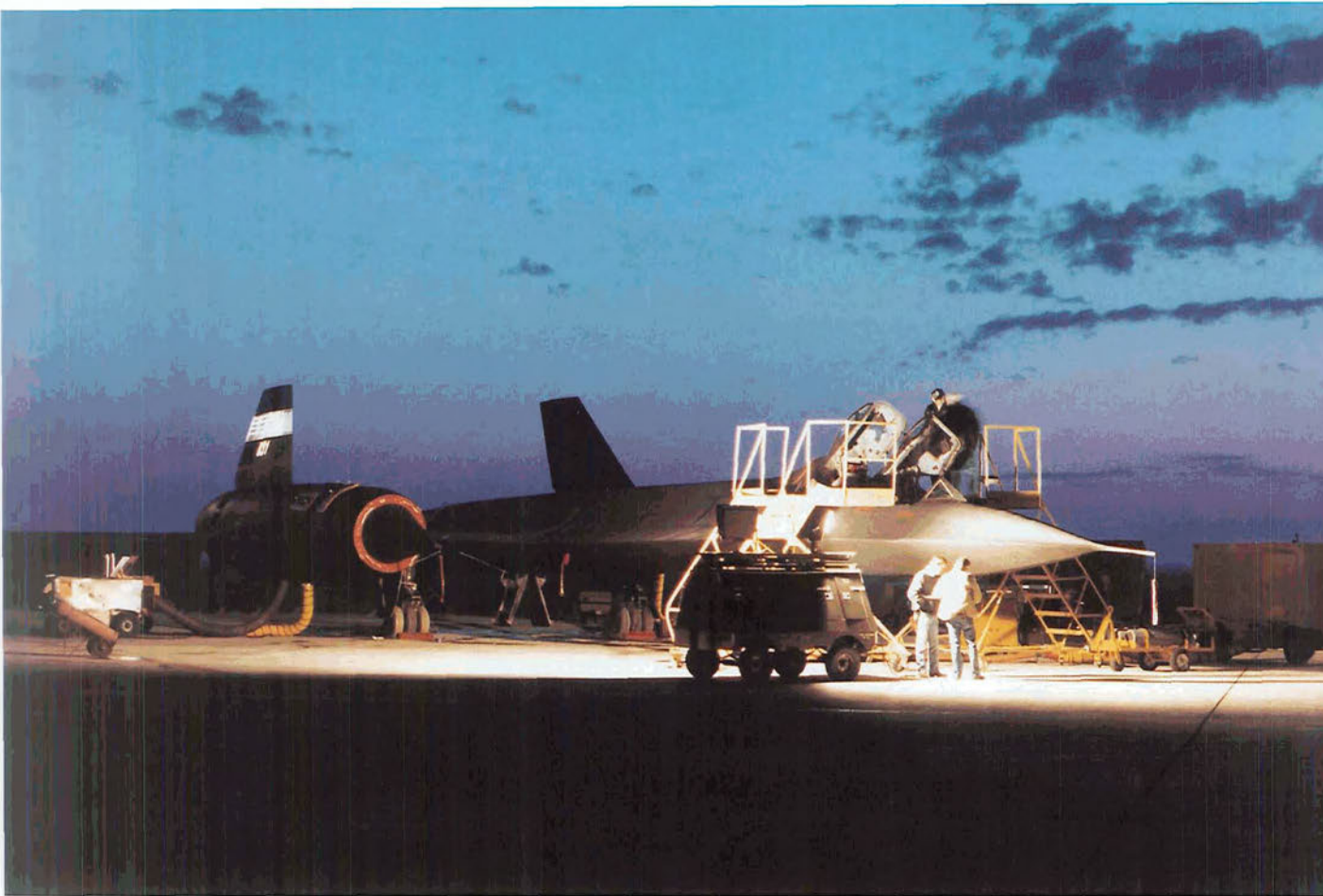
SR-71 being worked on at night on ramp. The aircraft was one of three SR-71s loaned to NASA by the Air Force for use as high-speed, high-altitude testbeds for research in such areas as aerodynamics, propulsion, structures, thermal protection materials, and instrumentation. Data from the SR-71 research program could aid designers of future supersonic/hypersonic aircraft and propulsion systems. (NASA Photo EC92 3103-8)
