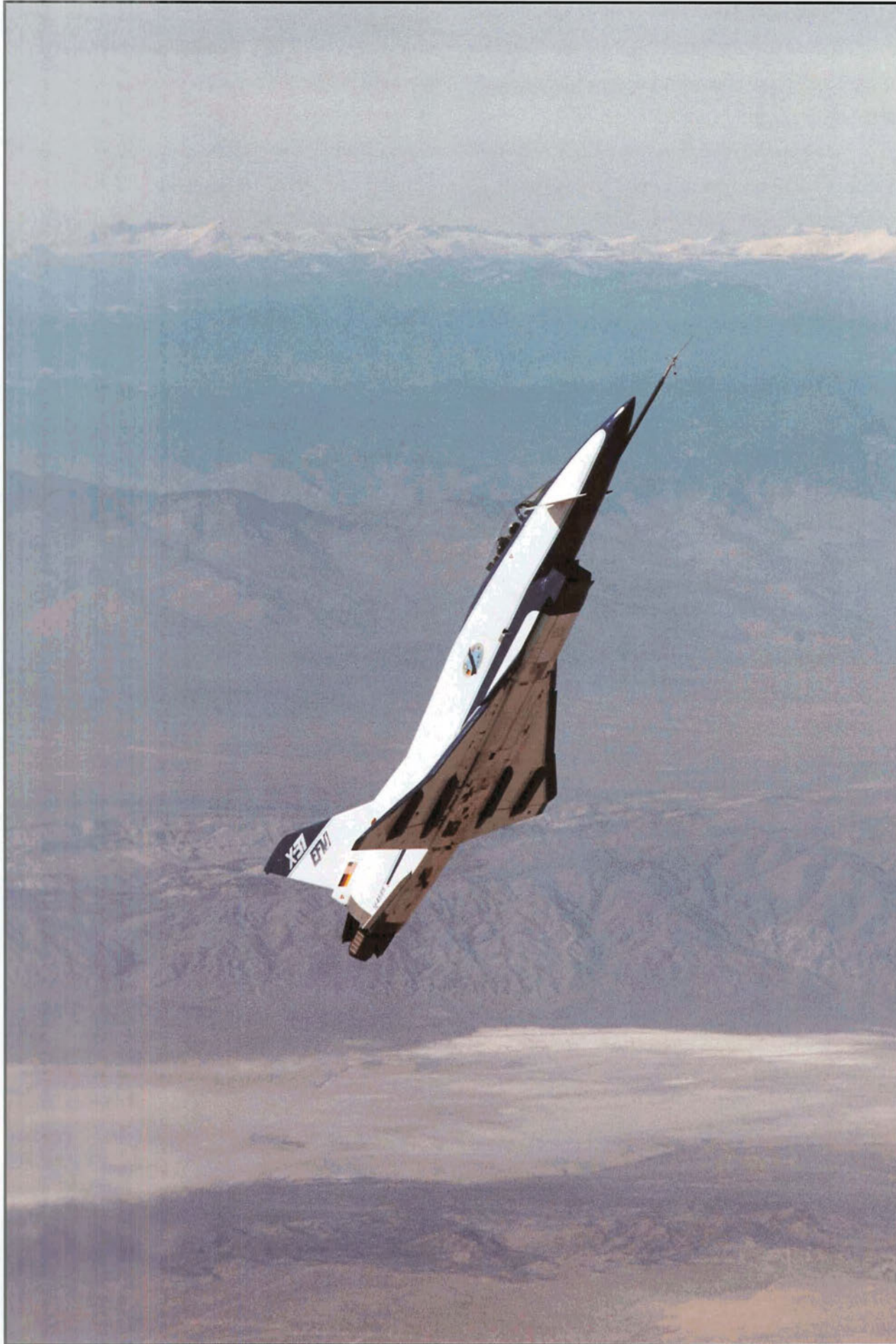
X-31 flying at a high angle of attack and demonstrating an entry into a Herbst maneuver—a rapid, 180-degree turn at an extremely high angle of attack, named after the German originator of the X-31 program, Wolfgang Herbst (NASA Photo EC94 42478-4)
