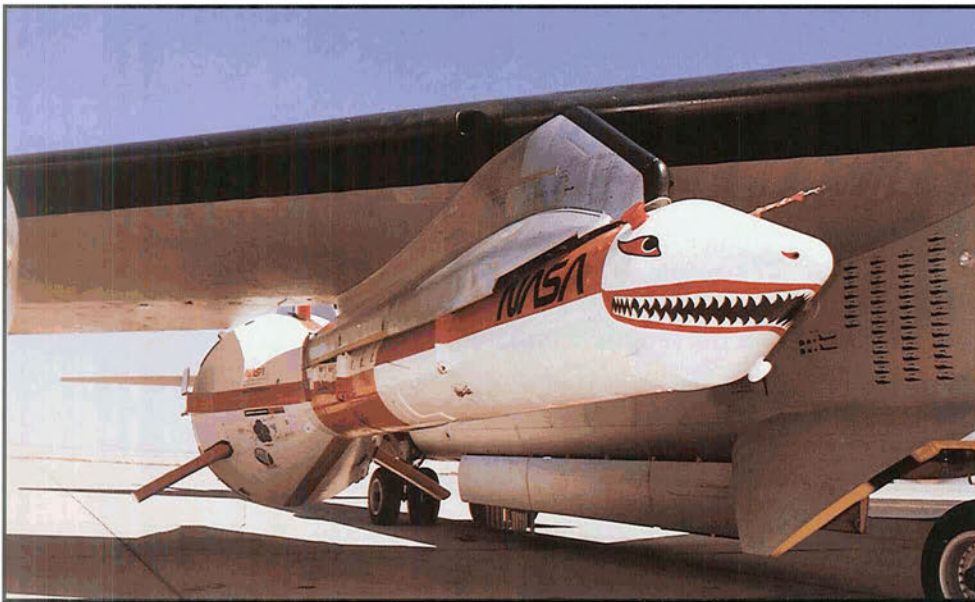
A simulated (smaller) version of the Shuttle's solid rocket booster (SRB) mounted under the wing of NASA's B-52 in preparation for the flight testing of the parachute system to be used in SRB recovery (NASA Photo ECN 9874)
