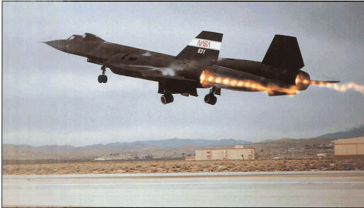
SR-71B take-off from Edwards with "shock diamonds" in the exhaust (NASA Photo EC92 1284-01)
