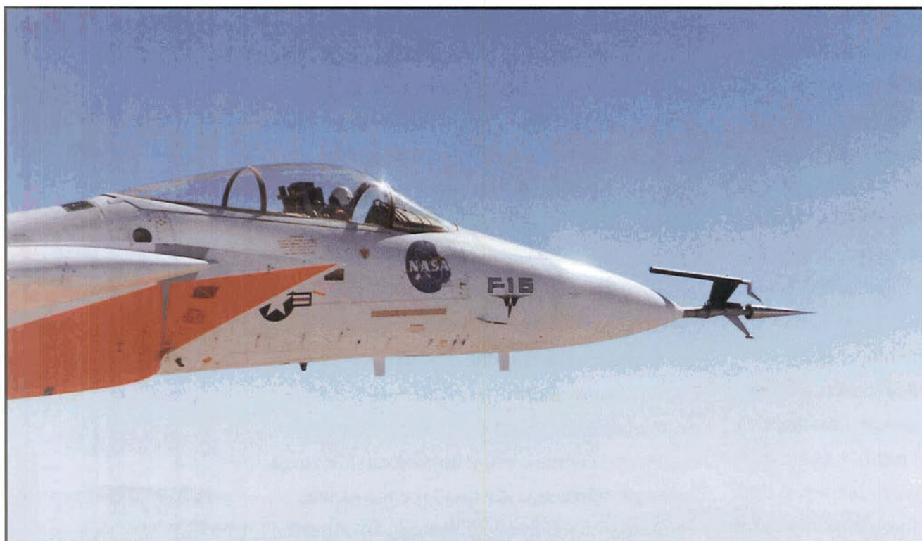
Close-up of F-15 10-degree cone experiment. (NASA Photo ECN 9811)
