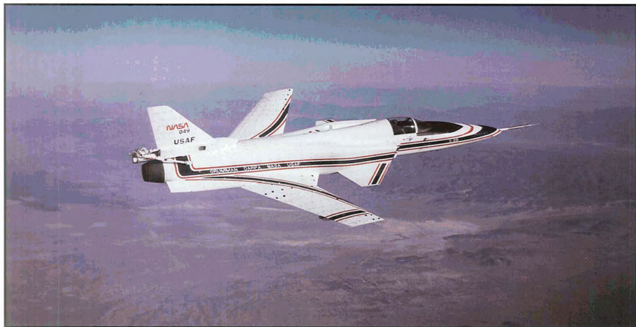
X-29 in flight at an angle that highlights the forward swept wings (NASA Photo EC90 039-4)
