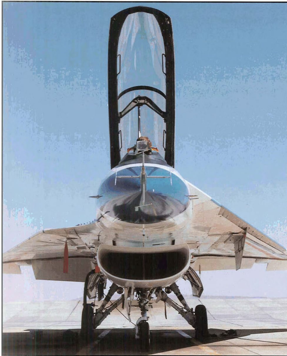
Two-seat F-16XL, showing asymmetric wings and (on the left wing, as viewed by the pilot) the bottom portion of the Supersonic Laminar Flow Control (SLFC) glove designed to help keep air flow smooth. (NASA Photo EC95 43267-2)
