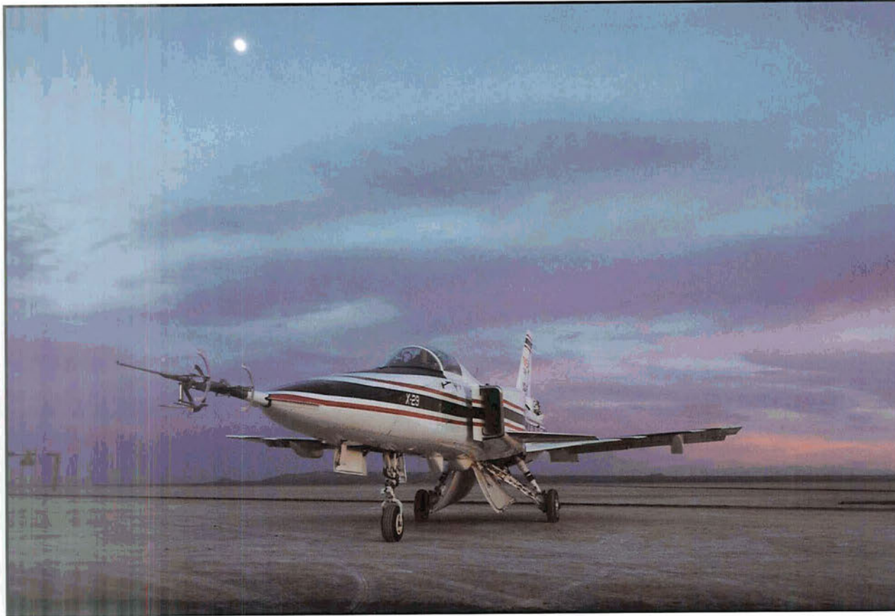
X-29s on lakebed near sunrise with the Moon still visible. (Pitot tube of second aircraft at viewer's left.) Both of these forward-swept-wing aircraft were flown at Dryden from 1984 to 1992 as technology demonstrators to investigate a host of advanced concepts and technologies. These included advanced composite materials, the forward-swept wing, and a computerized fly-by-wire flight control system that overcame the aircraft's inherent instability. The 434 total missions flown by the two X-29s provided an engineering data base that is available in the design and development of future aircraft. (NASA Photo EC90 357-7)
