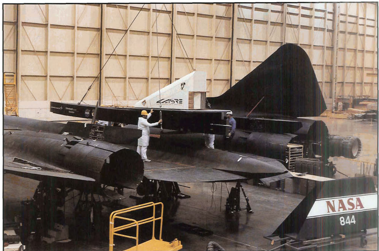
Side-view of the Linear Aerospike SR-71 Experiment (LASRE) pod on NASA SR-71, tail number 844. This photo was taken during the fit-check of the pod on 15 February 1996, at Lockheed Martin's Skunkworks in Palmdale, California. The LASRE will be flight tested during 1996 at Dryden. LASRE is designed to flight test the linear aerospike rocket engine mounted on a 10-percent-scale, half-span model of Lockheed Martin's X-33 Reusable Launch Vehicle concept. Among other partners involved in the project are Rockwell's Rocketdyne Division, builder of the aerospike engine, the Marshall Space Flight Center, Dryden, the Air Force's Phillips Lab, and Lockheed Martin Astronautics. (NASA Photo EC96 43419-25)
