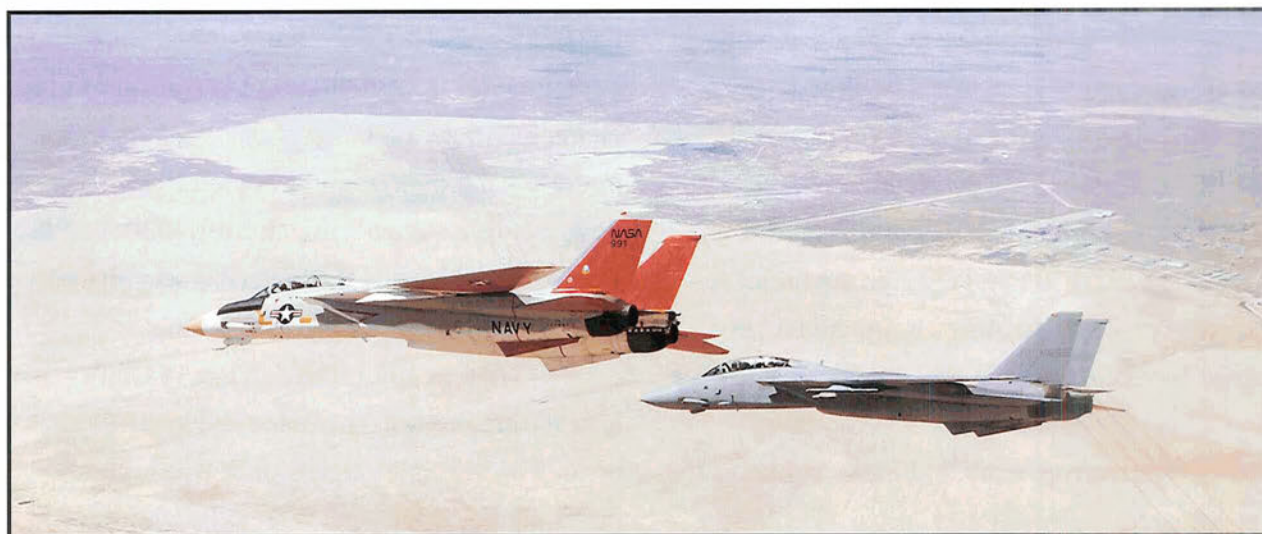
F-14s in formation above Rogers Dry Lakebed testing a new control law to improve the aircraft's spin response, 1982 (NASA Photo 20325)
