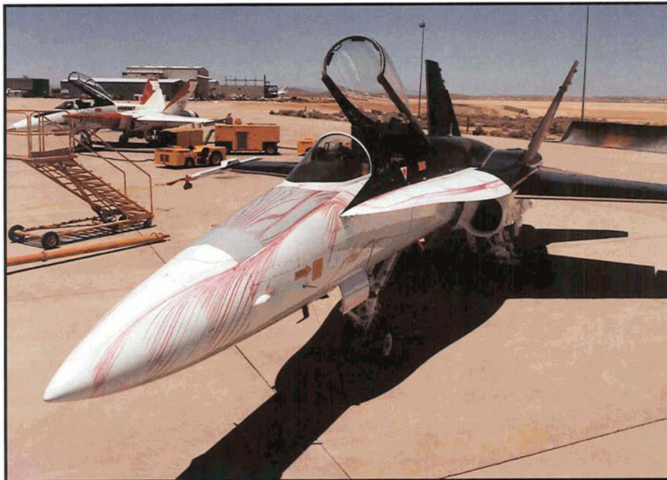
F/A-18 High Angle-of-Attack Research Vehicle showing the results of releasing a glycol-based liquid dye from very small holes around the nose of the aircraft during flight at about 30 degrees angle of attack. The airflow pattern revealed by the lines on the fuselage and wing helped researchers from Dryden, Ames and Langley research centers to visualize what was happening in flight and to compare forebody flows with predictions obtained from wind-tunnel testing and computational fluid dynamics simulations. (NASA Photo EC88 0115-79)
