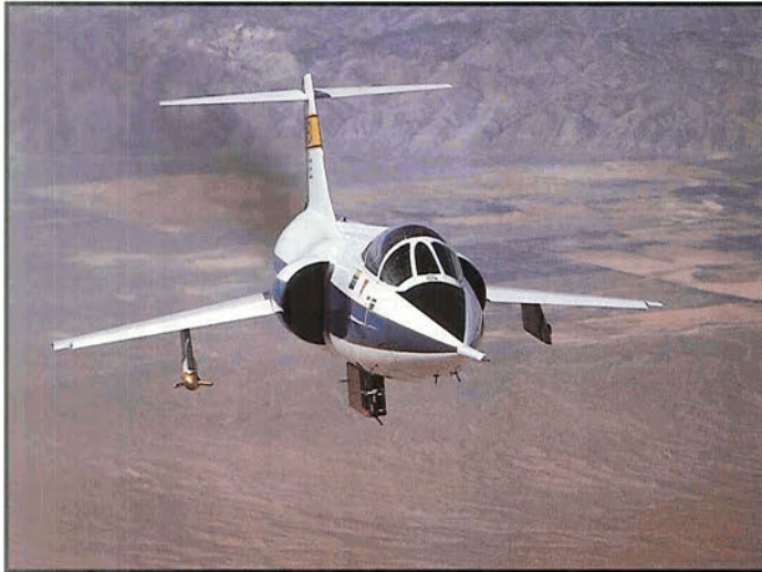
Top: F-104 shown head-on while engaged in Space Shuttle tile research. Flights of this aircraft in rain and through clouds provided valuable data on the extent to which the tiles could withstand rainy conditions during launch. (NASA Photo EC90 224)
