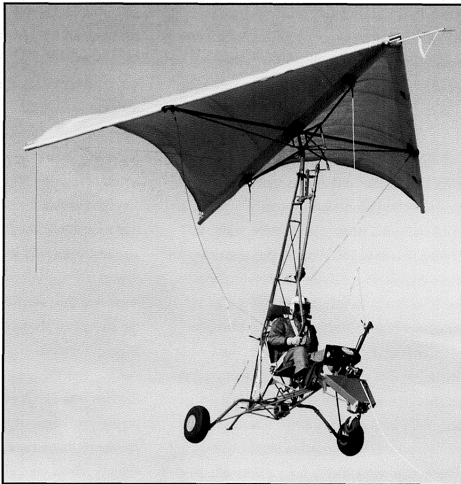
Paresev in flight, providing a low-cost way to test the flight-control issues of a parawing concept for possible use in returning spacecraft to Earth (NASA Photo E 8013)
