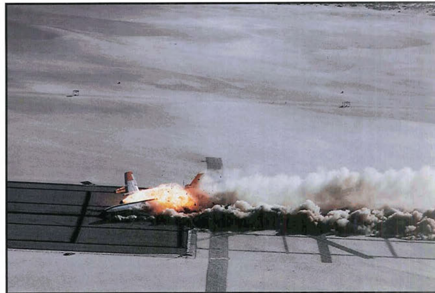
Above Left: Remotely piloted Boeing 720 Controlled Impact Demonstration aircraft following impact with iron posts (cutters) implanted in the lakebed to pierce the fuel tanks and test an anti-misting fuel for its ability to prevent fuel fires during airplane crashes (NASA Photo EC84 31806)
