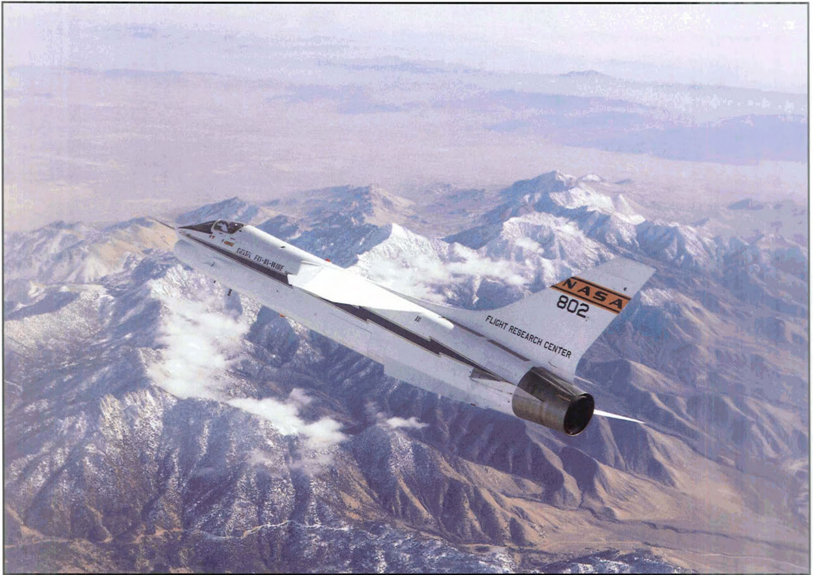
F-8 Digital Fly-By-Wire (DFBW) aircraft flying over the mountains near the Dryden Flight Research Center. The DFBW project at Dryden demonstrated the feasibility of computerized, fly-by-wire flight control, which reduced the weight and maintenance costs of airplanes and made such inherently unstable aircraft as the F-16, X-29, and X-31 possible for pilots to fly with the aid of their flight-control computers. (NASA Photo ECN 3478)
