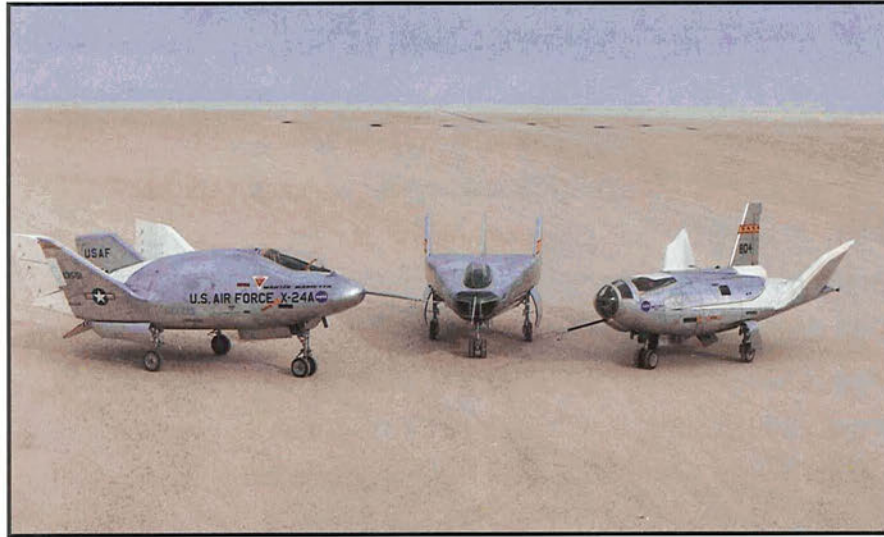
These wingless, lifting-body aircraft sitting on Rogers Dry Lakebed are, from left to right, the X-24A, M2-F3, and HL-10. The lifting-body aircraft studied the feasibility of maneuvering and landing an aerodynamic craft designed for reentry from space. Launched by a B-52 mothership, the lifting bodies flew, powered by their own rocket engines, before making an unpowered approach and landing. They helped validate the concept that a Space Shuttle could make safe, accurate, landings without power. (NASA Photo ECN 2359)
