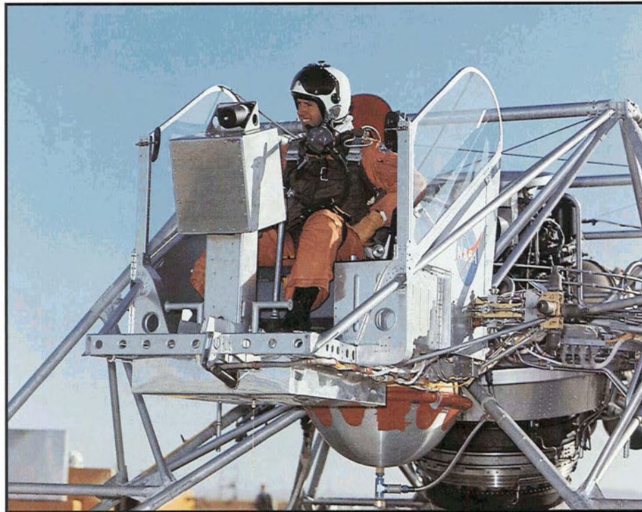
Joe Walker in a Lunar Landing Research Vehicle (LLRV) (NASA Photo ECN 453)
