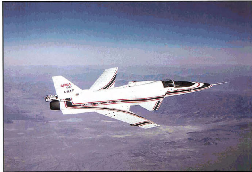
The No. 2 X-29 technology demonstrator aircraft, flown by NASA's Dryden Flight Research Center in a joint NASA-Air Force program to investigate the unique design's high angle-of-attack characteristics and its military utility. Angle of attack is the angle of an aircraft's body and wings relative to its actual flight path. This aircraft was flown at Dryden from May 1989 until August 1992. (NASA Photo EC90 0039-4)
