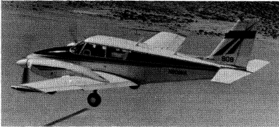
The Flight Research Center's Piper Twin Comanche, which helped validate the RPRV concept, descends to a remotely controlled landing on Rogers Dry Lake, unassisted by the onboard pilot.
