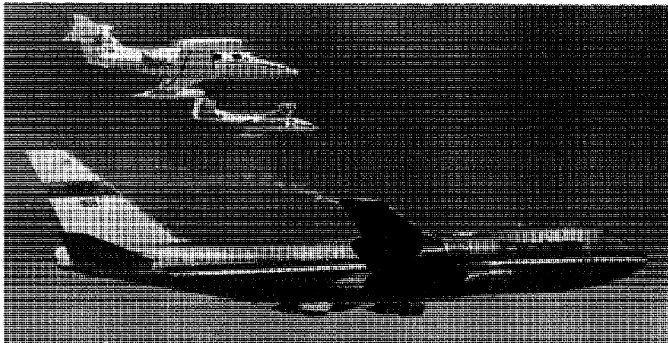
NASA's Boeing 747, used on wake vortex alleviation studies, is followed by a Gates Learjet (left) and Cessna T-37 that penetrate the 747's wake to analyze its turbulence and strength.
