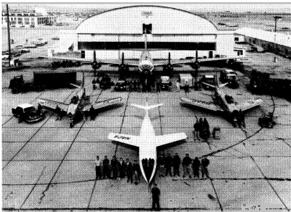
These personnel members and this equipment were used by the NACA High-speed Flight Station to support one flight of the NACA D-558-2 Skyrocket. Note the two Sabre chase planes, the modified B-29 launch aircraft, and the profusion of ground support equipment, including communications, tracking, maintenance, and rescue vehicles. Research pilot A. Scott Crossfield stands in front of the Skyrocket.
