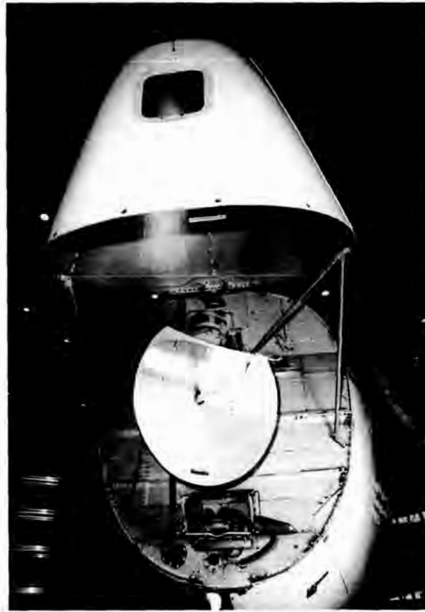
Radome of the Boeing 737 testbed aircraft, used to provide information to the helmet mounted display.
