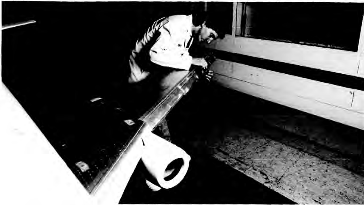
A Langley technician works on the wing of the model Boeing 737 in the 14 by 22 foot subsonic wind tunnel.
