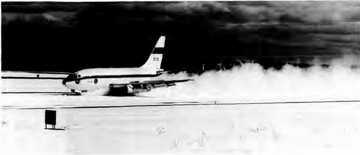
The Boeing 737 testbed during runway friction tests at Brunswick Naval Air Station, Maine, in 1985.
