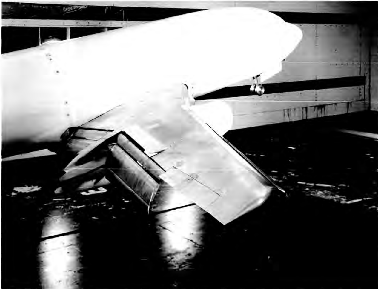
A 1/8th scale model of the Boeing 737 undergoing wing tests in the Langley Research Center wind tunnel. This research tested flow physics over the aircraft wing. Over 700 pressure ports were placed on the right-hand wing to measure airflow.
