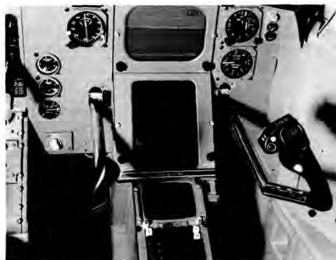
Close-up of co-pilot's position on the aft flight deck of the NASA 737 research aircraft showing "Brolly Handle" flight controls and color CRT displays.
