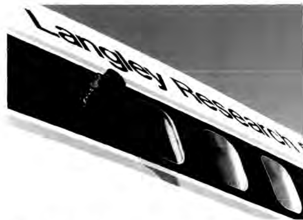
Close-up of the side-mounted infrared sensor used in the windshear detection program.
