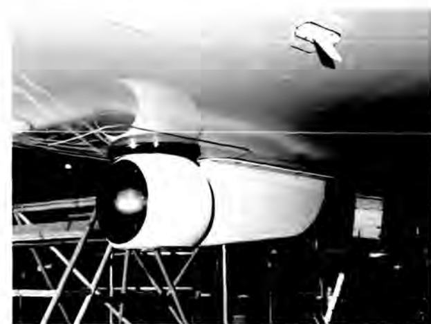
Close-up of the Light Detection and Ranging (LIDAR) radar mounted on the lower fuselage.
