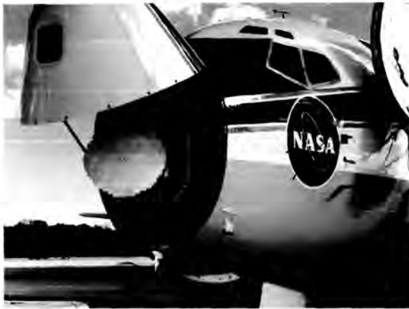
A flat plate airborne radar used in the microburst windshear detection research program was housed in the nose of the NASA 737 aircraft.
