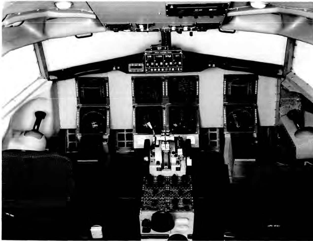
The aft flight deck of the NASA 737 with both sets of "Brolly Handles" replaced with McFadden sidestick controllers and color displays.
