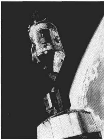
Once in orbit, the Apollo spacecraft separated from the S-IVB stage, then doubled back to dock with the docking module (DM) poised on the S-IVB (watercolor conception by Paul Fjeld). After collecting the DM, Apollo fired up for rendezvous with Soyuz. The first problem of the flight occurred when Brand found he could not remove the docking probe from the tunnel entrance to the DM. Troubleshooters found that an improperly installed pyrotechnic connector (shown in this Rockwell photo taken before acceptance of the probe) had eluded Rockwell and NASA inspectors.
