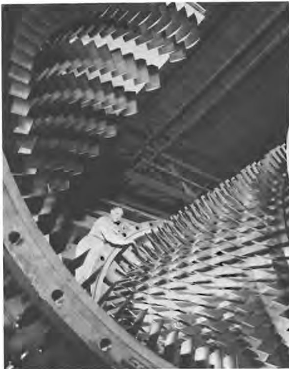
With the stationary housing blades removed, a technician inspects the rotor blades of the compressor in Langley's 4-foot supersonic wind tunnel. (LaRC)
