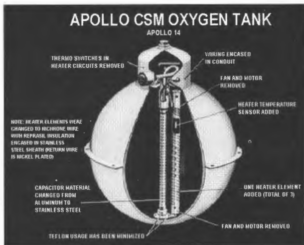
Diagram of CSM oxygen tank modified following the Apollo 13 accident (NASA S71-16745).
