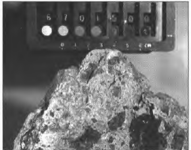
Lunar sample 67015. The white matrix consists of finely fractured and crushed mineral and rock detritus, predominantly feldspar (NASA S72-37216).
