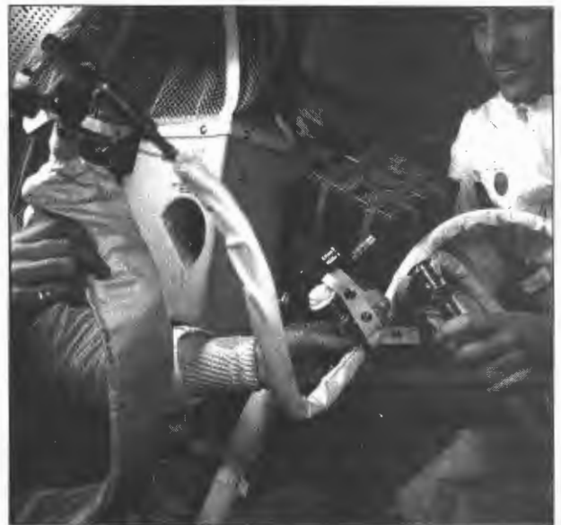
Swigert with temporary hose connections and apparatus required when the crew moved from the CM to the LM (NASA AS13-62-9004).
