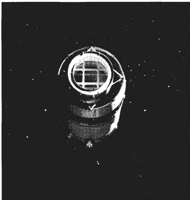
View of Saturn V stage following separation from the CSM (NASA AS08-16-2583).
