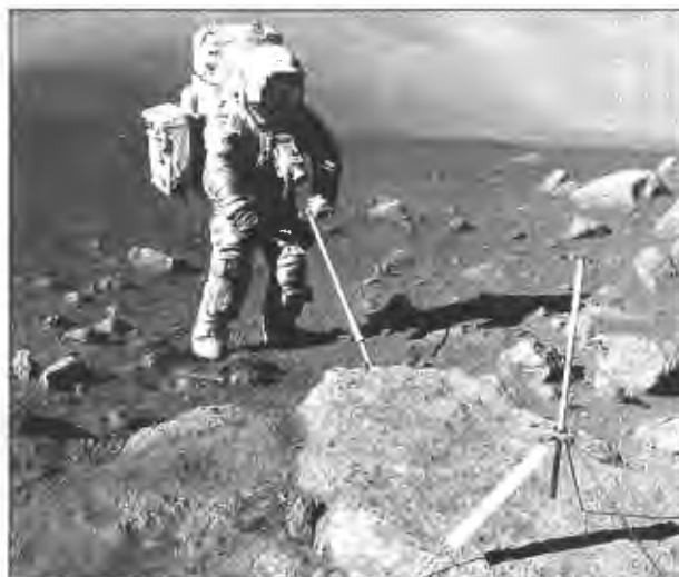
Schmitt uses a "lunar scoop" to retrieve soil samples at station 5 during EVA-2 (NASA AS17-145-22157).
