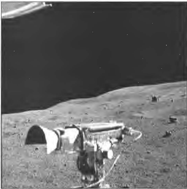
Close-up of the RCA television camera affixed to the LRV. The LM is up slope (NASA AS16-115-18549).
