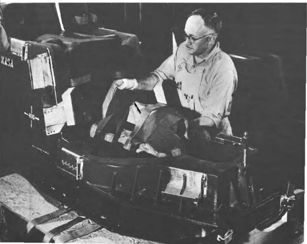
After the plastic mold had hardened, it was finished with fibrous material (above). Then the contour couch was clamped to the metal seat and fitted with harness and restraining straps (below) in preparation for installation in Mercury spacecraft.
