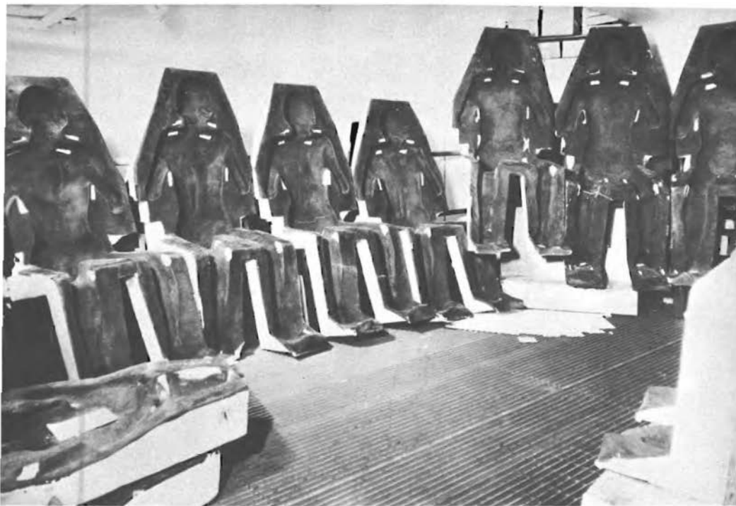
After the plastic mold had hardened, it was finished with fibrous material (above). Then the contour couch was clamped to the metal seat and fitted with harness and restraining straps (below) in preparation for installation in Mercury spacecraft.
