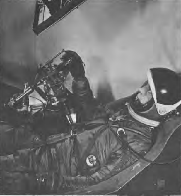
Astronauts had to learn to live with and operate in their life-support equipment. Above, Astronaut Shepard lies on a contour couch in his MC-IV pressure suit and practices navigation on the Langley Research Center simulator. Astronaut Cooper (right) is lifted in his pressure suit into a prototype net couch in Hangar S at Cape Canaveral, Florida.
