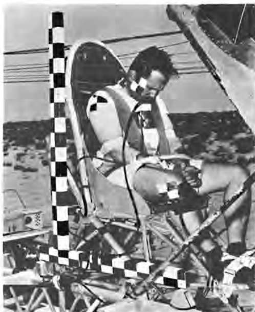
Lt. Col. John P. Stapp, USAF (MC), was a pioneer in the development and use of the research sled for deceleration tests. He is shown here just before a run on the deceleration sled at Edwards AFB, Calif., with accelerometers at mouth, chest, and knee.
