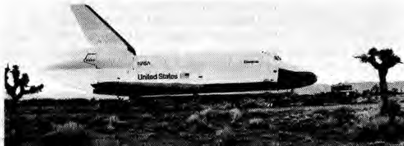
Space Shuttle orbiter Enterprise, with tailcone covering engine-nozzle location, moves on a 90-wheel rig January 31 from the Rockwell plant to DFRC 35mi away in preparation for approach and landing tests. (NASA 77-H-77)
