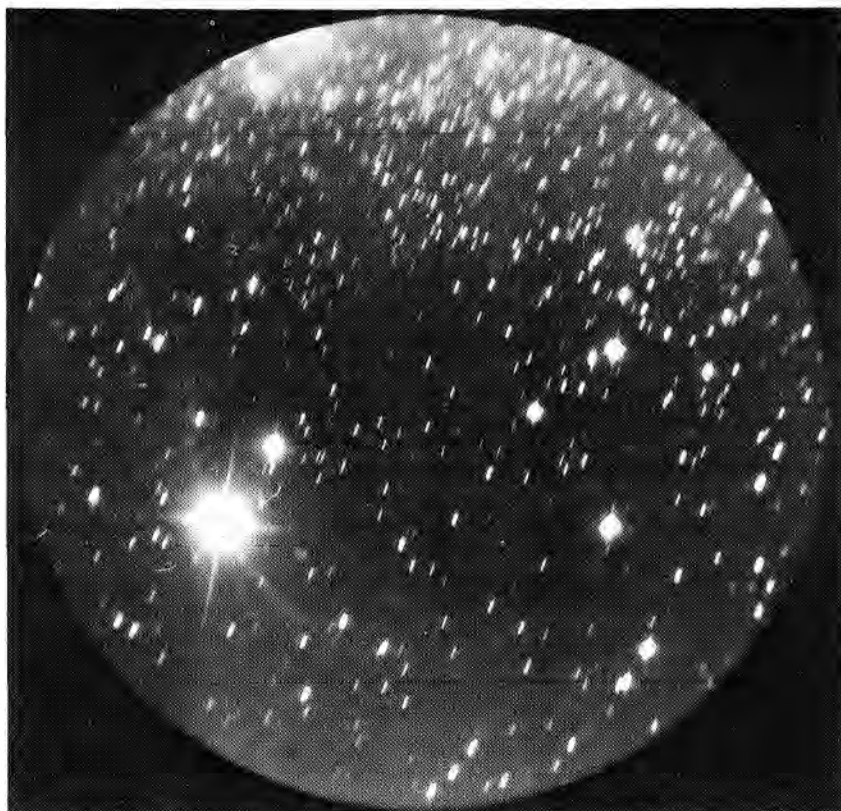
April 16-27: Stars near the center of the Milky Way galaxy were photographed from the surface of the moon during Apollo 16. An ultraviolet camera/spectrograph, designed and built by the Naval Research Laboratory, made photos in far ultraviolet light with hydrogen light filtered out, recording only the very hot, blue stars (streaked in the photo because of the moon's rotation during the 30-minute exposure).
