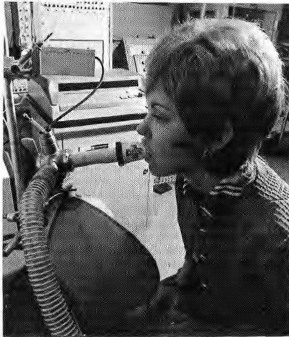
July 4: NASA's mid-year review of collateral space technology benefits on the earth described a compact, fully automatic, mobile medical gas analyzer (above). The analyzer measured composition of air breathed in and exhaled from the lungs to monitor pulmonary and cardiovascular activity in patients. Industrial items included an ultrathin, two-volt switching circuit for buildings. Low-volt circuits were displayed at the Second Annual Urban Technology Conference in San Francisco July 24-26.
