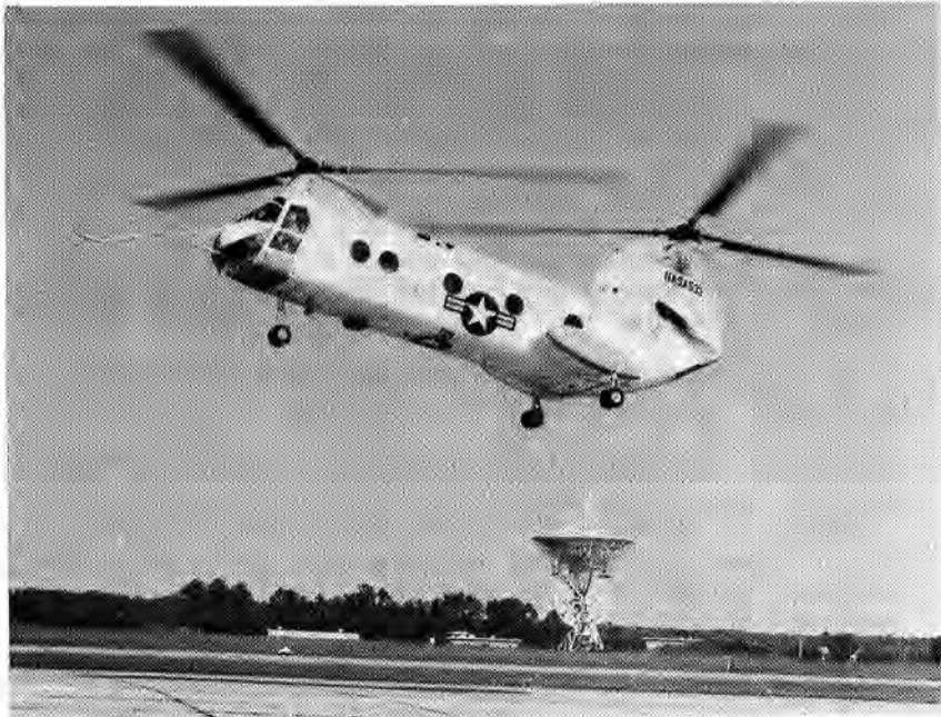
February 17: The first fully automatic landings by a manned helicopter at a predetermined spot were announced by NASA. A Langley Research Center team had made the landings at Wallops Station the second week in February in a research program to permit helicopters and future VTOL aircraft to fly under conditions of poor visibility.
