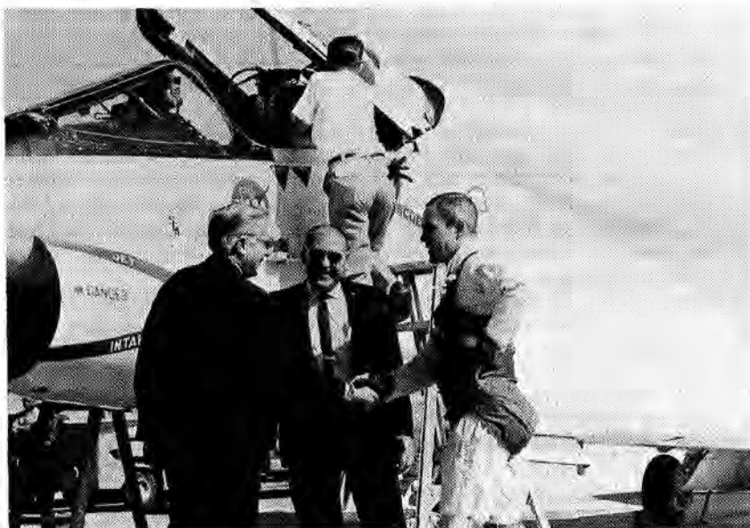
March 9: Dr. Richard T. Whitcomb (left), developer of NASA's supercritical wing, congratulated test pilot Thomas C. McMurtry after the successful first flight of the wing on the TF-8A jet aircraft. Program Manager John G. McTigue looked on. The new airfoil shape, undergoing tests at the Flight Research Center, was designed to reduce buffeting at high subsonic speeds and permit increased aircraft performance.
