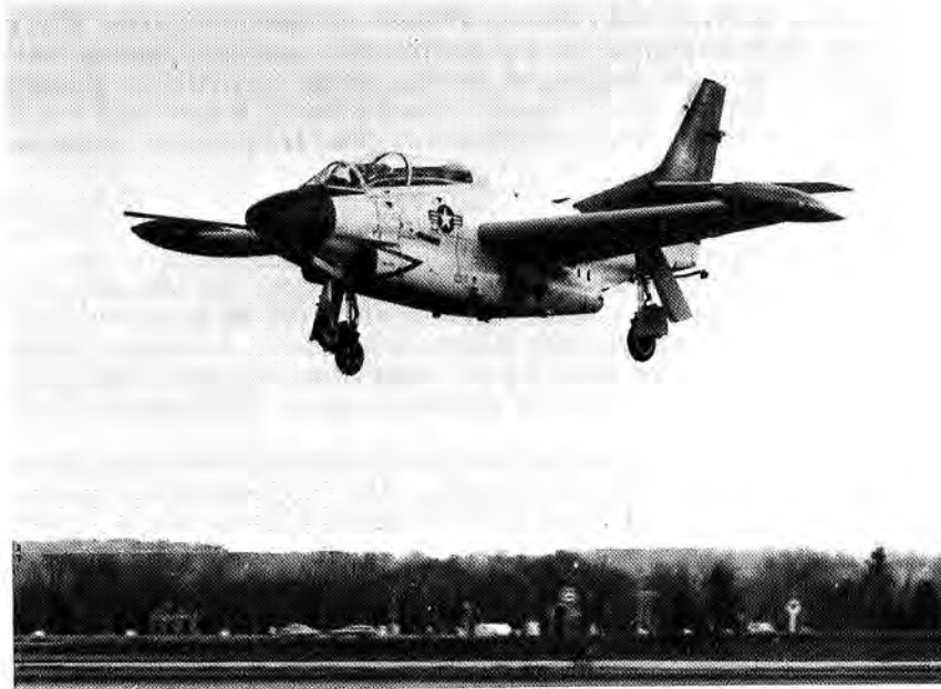
November 24: NASA's thick supercritical test wing was flight-tested on a USN T2-C aircraft for the first time, in flight from the North American plant in Columbus, Ohio. Joint NASA-USN program was testing the new airfoil that might save structural weight on moderate-speed aircraft. Thin version of the airfoil for maximum-speed performance, fitted to a modified F-8 jet fighter (below), was delivered to the Flight Research Center Nov. 3 for test flights beginning in the spring of 1971.
