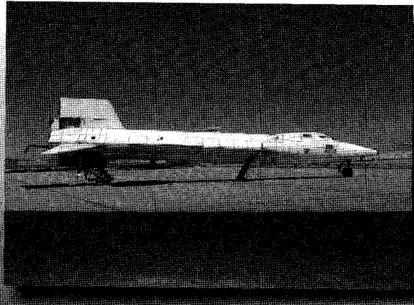
The X-15A-2 after Knight's Mach 6.7 flight. Unexpected heating burned through both the spray-on heat shield and the metal fuselage. The vehicle never flew again. (ECN-1834)
