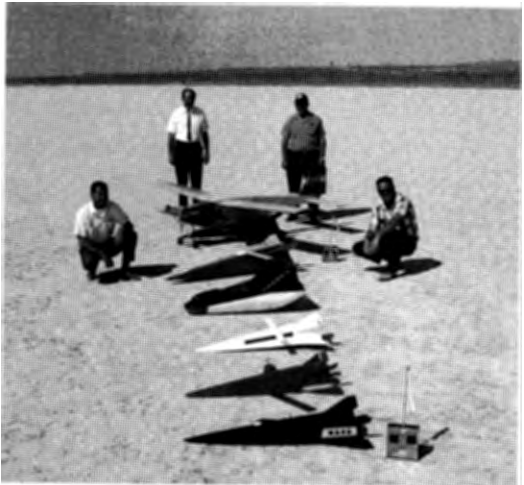
From left, Richard C. Edredge, Dale Reed, James O. Newman and Bob McDonald with several of Reed's research models. Throughout his years at Dryden, Reed made extensive use of model aircraft to test new concepts. This began with the early lifting bodies and continued on through the X-33 and X-38 vehicles. (ECN-2059)
