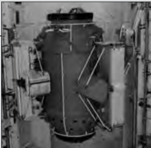
The Russian-built Docking Module (DM) sits in the back of Atlantis 's payload bay. It was attached to Mir during STS-74. (KSC-95EC-1616)
