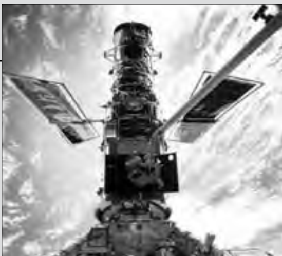
Astronaut John Grunsfeld, positioned on a foot restraint on the end of Discovery's Remote Manipulator System (RMS), prepares to replace a radio transmitter in one of the Hubble Space Telescope's electronics bays on mission STS-103. (STS103-713-048)
