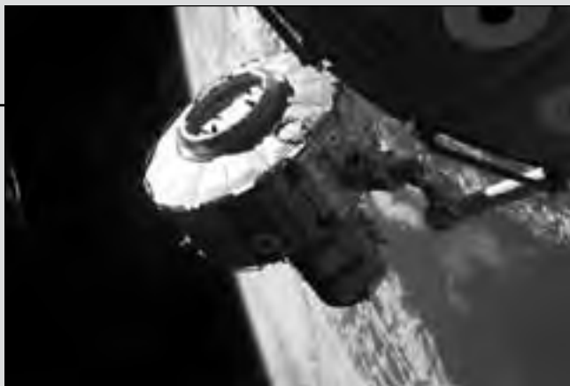
STS-104, backdropped against the blue and white Earth some 237 miles below, the Quest Airlock is in the process of being installed onto the starboard side of Unity Node 1 of the ISS. Astronaut Susan Helms, Expedition 2 flight engineer, used controls on board the Station to maneuver the airlock into place with the Canadarm 2, or Space Station Remote Manipulator System. (STS104-E-5068)
