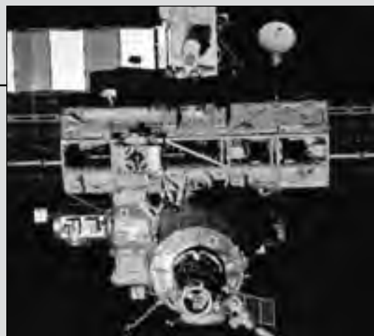
This close-up view of the ISS, newly equipped with the 12,247-kilogram (27,000-pound) S0 truss, was photographed by one of the astronauts on board Space Shuttle Atlantis during STS-110. S0 is the first segment of the Station's truss structure, which will ultimately expand the Station to the length of a football field. (STS110-729-055)
