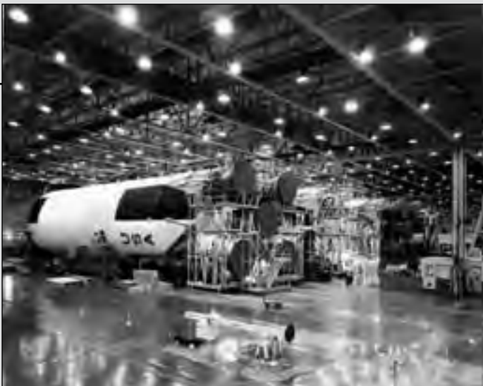
The Saturn V first stages, S-1C-10, S-1C-11, and S-1C-9, are in the horizontal assembly area for the engine (five F-1 engines) installation at Michoud Assembly Facility. (GPN-2000-000048)
