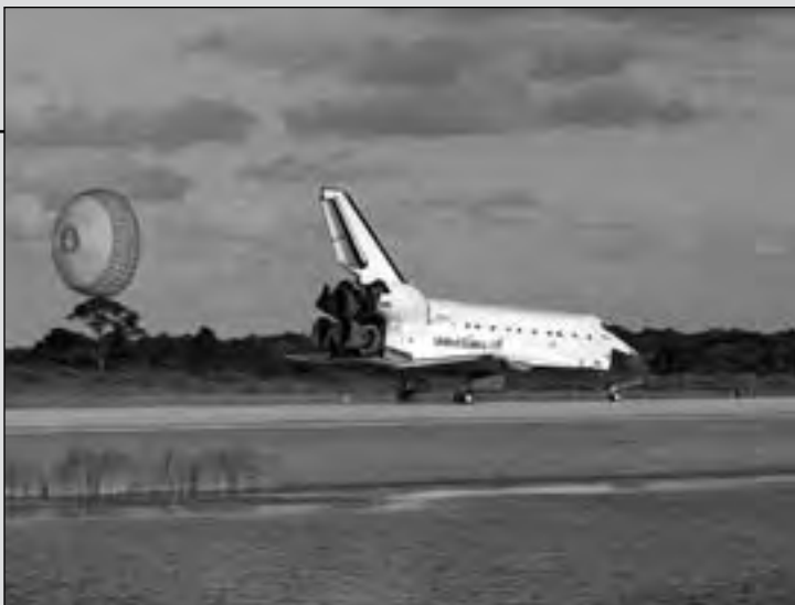
The orbiter drag chute deploys after Space Shuttle Atlantis lands on runway 15 of the Kennedy Space Center Shuttle Landing Facility (SLF) after STS-86. (97PC-1492)
