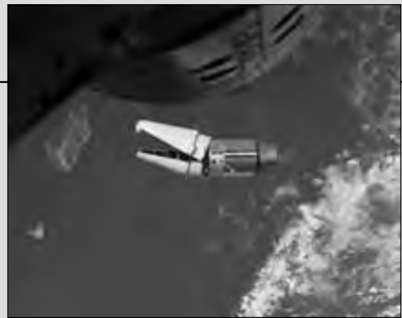
The Augmented Target Docking Adapter (ATDA) as seen from the Gemini IX spacecraft during one of their three rendezvous in space. Failure of the docking adapter protective cover to fully separate on the ATDA prevented the docking of the two spacecraft. The ATDA was described by the Gemini IX crew as an "angry alligator." (S66-37923)
