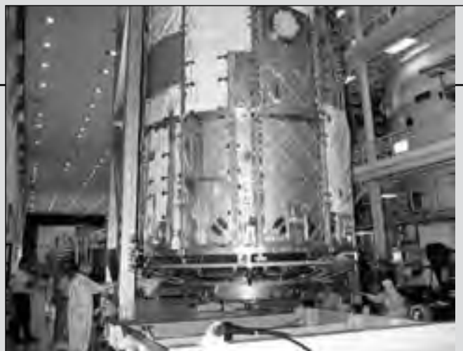
In the Operations and Checkout Building, the U.S. Lab named Destiny reaches the open floor after being lifted out of the vacuum chamber where it was tested for leaks. During STS-98, the crew installed the Lab on the Space Station during a series of three spacewalks in February of 2001. (KSC-00PP-0870)
