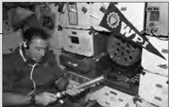
Payload specialist Albert Sacco, Jr., inspects a crystal in a cylindrical autoclave on the middeck of the Earth-orbiting Space Shuttle Columbia , mission STS-73. (STS073-353-018)
