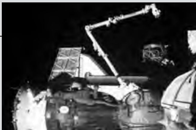
Moments prior to the undocking of Space Shuttle Atlantis from the ISS, an Expedition 4 crew member took this digital still photograph from a window in the Pirs Docking Compartment. Visible in this image are the Soyuz spacecraft, Space Station Remote Manipulator System (SSRMS)/Canadarm 2, and Pressurized Mating Adapter 3. (ISS004-E-10071)
