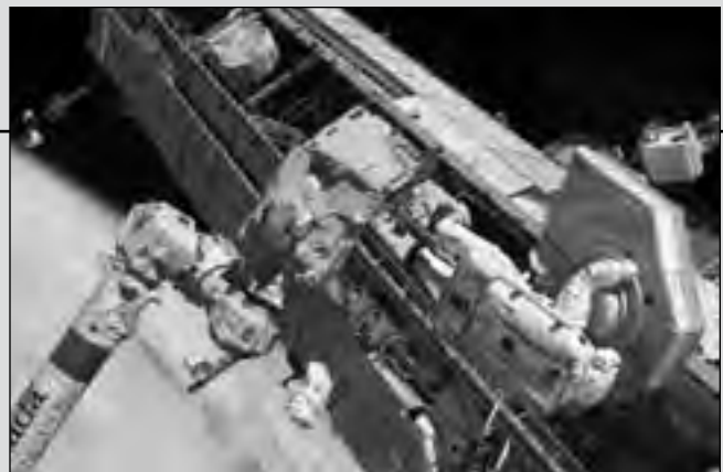
STS-121 mission specialists Michael Fossum and Piers Sellers (out of frame) install the new trailing umbilical system in the mobile transporter on the International Space Station during the mission's second session of extravehicular activity. (S121-E-06211)
