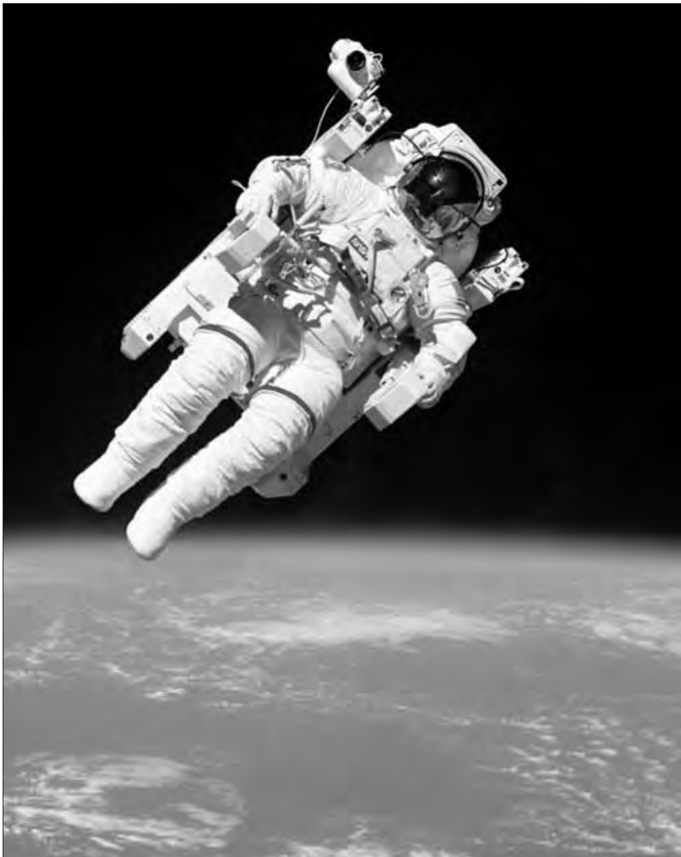
Mission specialist Bruce McCandless II ventured further away from the confines and safety of his ship than any previous astronaut ever had. This space first was made possible by the Manned Manoeuvring Unit (MMU), a nitrogen-jet-propelled backpack. After a series of test maneuvers inside and above Challenger's payload bay, McCandless went "free-flying" to a distance of 320 feet away from the orbiter. The MMU is controlled by joysticks positioned at the ends of the armrests. Moving the joysticks left or right or by pulling them fires nitrogen jet thrusters propelling McCandless in any direction he chooses. A still camera is mounted on the upper right portion of the MMU. This stunning view shows McCandless with the MMU amongst the black and blue of Earth and space. (S84-27017)
