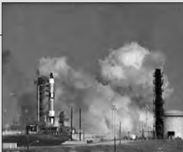
NASA attempted to launch Gemini VI at 9:54 a.m., 12 December 1965. However, seconds after ignition, the first-stage engine of the Gemini Launch Vehicle shut down due to the faulty release of a liftoff umbilical plug. (S65-59967)
