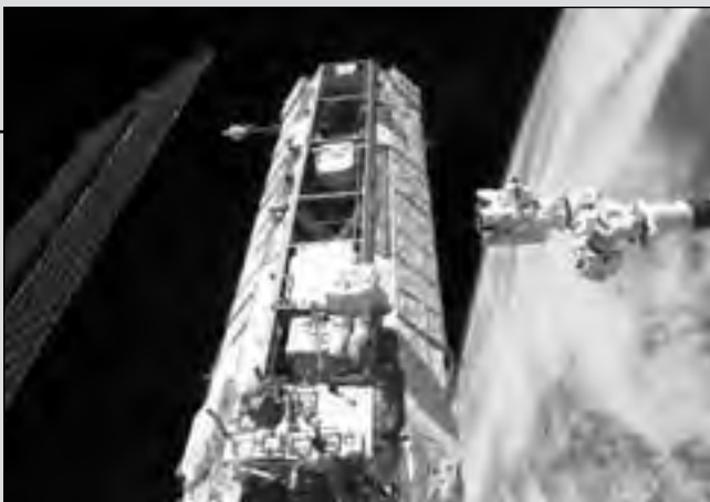
Astronaut Michael Lopez-Alegria, STS-113 mission specialist, works on the newly installed P1 truss on the International Space Station during a session of extravehicular activity. (ISS005-E-21771)
