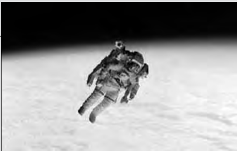
Astronaut Bruce McCandless, mission specialist, participates in an extravehicular activity (EVA) during STS-41B. He is using a nitrogen-propelled, hand-controlled manned maneuvering unit (MMU). He is performing this EVA without being tethered to the Shuttle and is approaching his maximum distance from Challenger . Below him is a cloudy view of Earth. (S84-27019)
