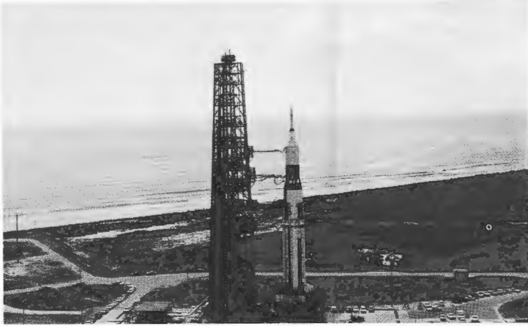
Saturn I being readied for launch from Cape Kennedy with boilerplate model of the Apollo spacecraft.
