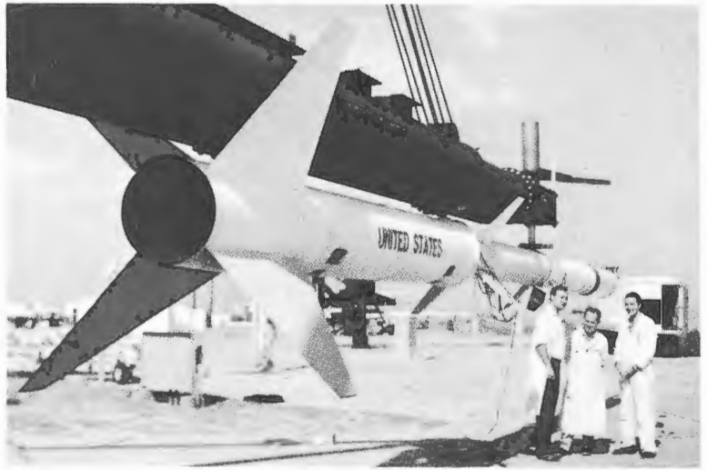
Javelin in horizontal position on the launcher, for last-minute checks during prelaunch operations.
