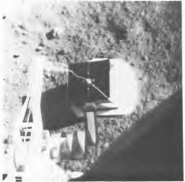
The Surveyor spacecraft, designed to make a softlanding on the moon. Surveyor 5's alpha-backscattering instrument, in the lower photo, analyzed chemical composition of the lunar surface after the 10 September 1967 landing.
