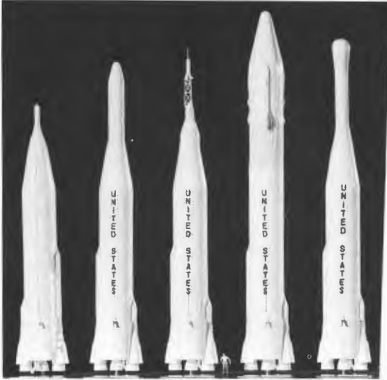
Models of Atlas upper-stage configurations. Left to right: Atlas, Atlas-Agena, Mercury-Atlas, Atlas-Centaur, Atlas-Able.
