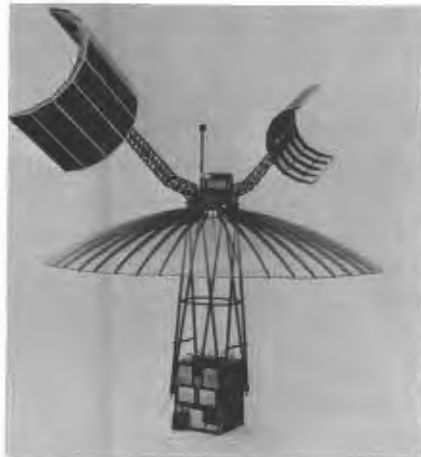
ATS 3, at left, suspended during antenna pattern testing. The model of ATS 6, below, shows the nine-meter reflector deployed.
