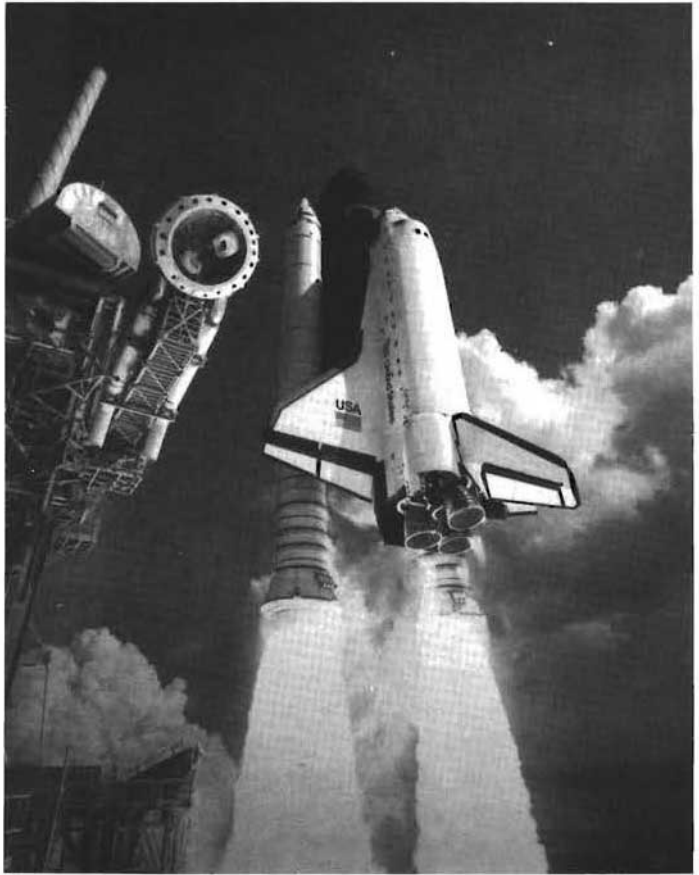
Space Shuttle Atlantis blasts toward orbit on two powerful solid rocket boosters. After they are dropped, the three main engines continue to fire, fueled by the large external fuel tank.
