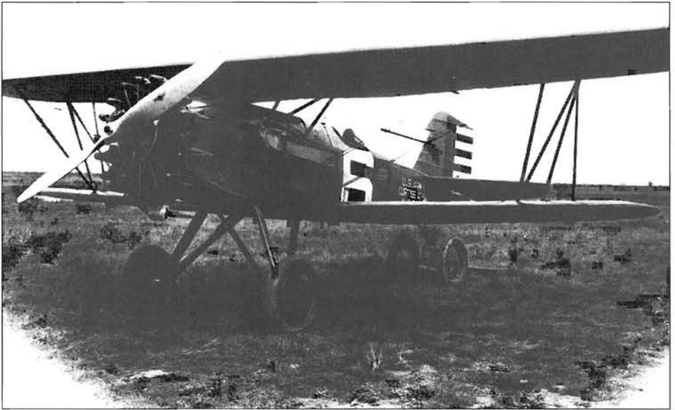
The Curtiss Hawk used in NACA Tests, in November 1928, before (above) and after (below) installation of the cowling. (NACA Photo 3018)
