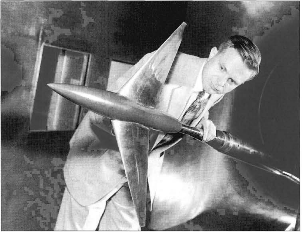
NACA/NASA Langley engineer Richard T. Whitcomb was awarded the 1954 Collier Trophy for his development of the "area rule," an innovation that revolutionized the design of virtually every transonic and supersonic aircraft ever built. Here Whitcomb inspects a research model in the 8-Foot Transonic Tunnel at Langley. (NASA photo no. LAL 89118).
