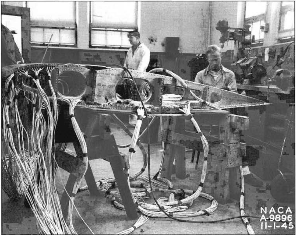
A laboratory test section of an electrically-heated airfoil for the C-46, in November 1945, with the thermocouples and nichrome electrical heating elements already installed. (NASA photo no. Ames A-9896).
