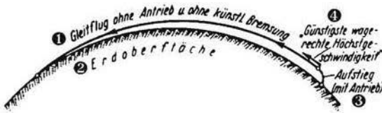
Figure 53. The most advantageous way of implementing an "express flight at a cosmic velocity" is as follows: the highest horizontal velocity is—corresponding to the distance—selected so large ("optimum horizontal velocity") that the entire long-distance trip can be made in gliding flight without power and without artificial braking (see Figure 50 for a diagram).
