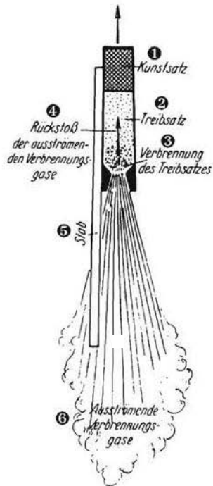
Figure 15. Fireworks rocket in a longitudinal section. The attached guide stick serves to inhibit tumbling of the rocket.
