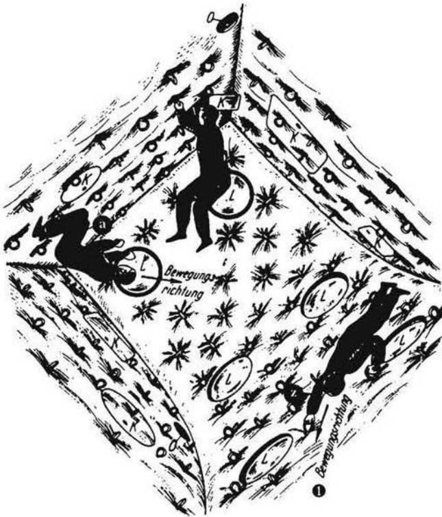
Figure 60. A room of the space station in which a weightless state exists and which is furnished accordingly: the walls are completely cushioned and equipped with straps. No loose object is present.
