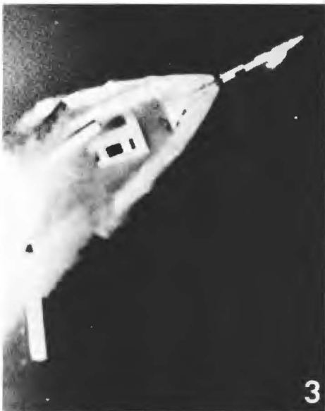
This spectacular series of photos shows the breakup of the A-003 Little Joe II at top left. The photos at top right, bottom left, and bottom right show the launch escape system lifting the boilerplate spacecraft safely away from the disintegrating booster.
