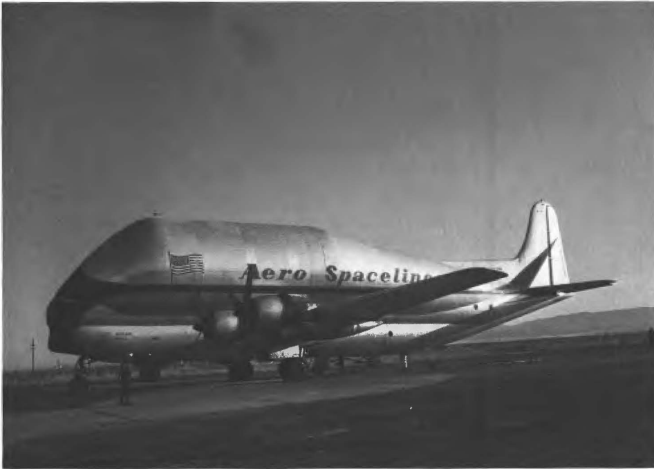
The Pregnant Guppy aircraft, which was used extensively by NASA to transport spacecraft during all phases of the Apollo program.
