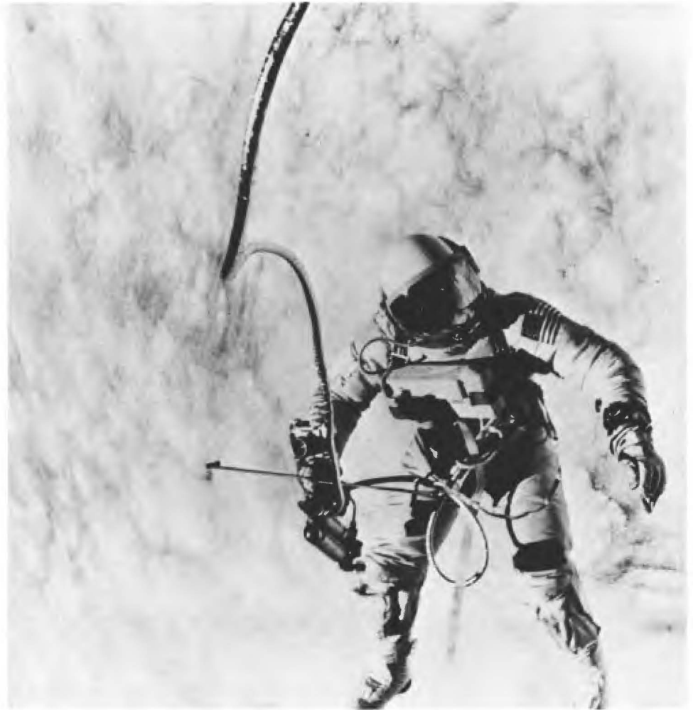
Astronaut Edward H. White II is shown during the third orbit of the Gemini IV flight as he floated in space, attached to the spacecraft by a 7.6-m (25-ft) umbilical line. His right hand gripped a hand-held self-manuevering unit which he used to propel himself during the 21-min "space walk."
