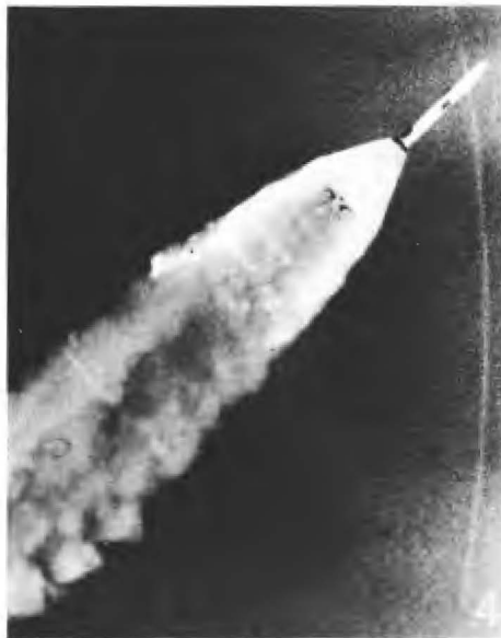
This spectacular series of photos shows the breakup of the A-003 Little Joe II at top left. The photos at top right, bottom left, and bottom right show the launch escape system lifting the boilerplate spacecraft safely away from the disintegrating booster.
