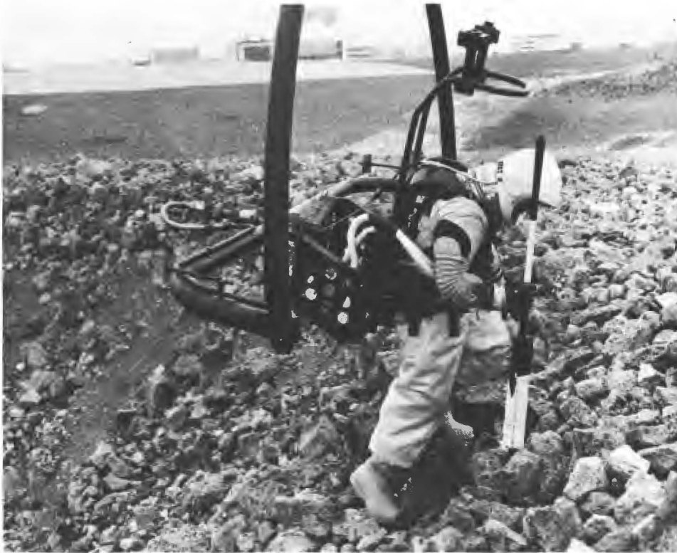
MSC test engineer Jack Slight is shown climbing out of a crater at the Center's Lunar Topographical Simulation Area. The six-degrees-of-freedom simulator in which he is strapped produces the effect of one-sixth earth gravity on his body. Slight is wearing an Apollo pressure suit and has a Jacob's staff in his hand.
