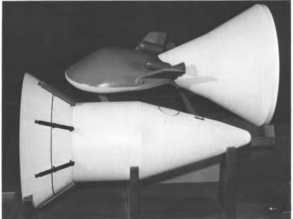
Models of two spacecraft concepts for Apollo. The designs, a semiballistic reentry vehicle and a winged glide-type spacecraft, resulted from the Project Apollo G.E. feasibility study in late 1960 and early 1961. (G.E. photo)
