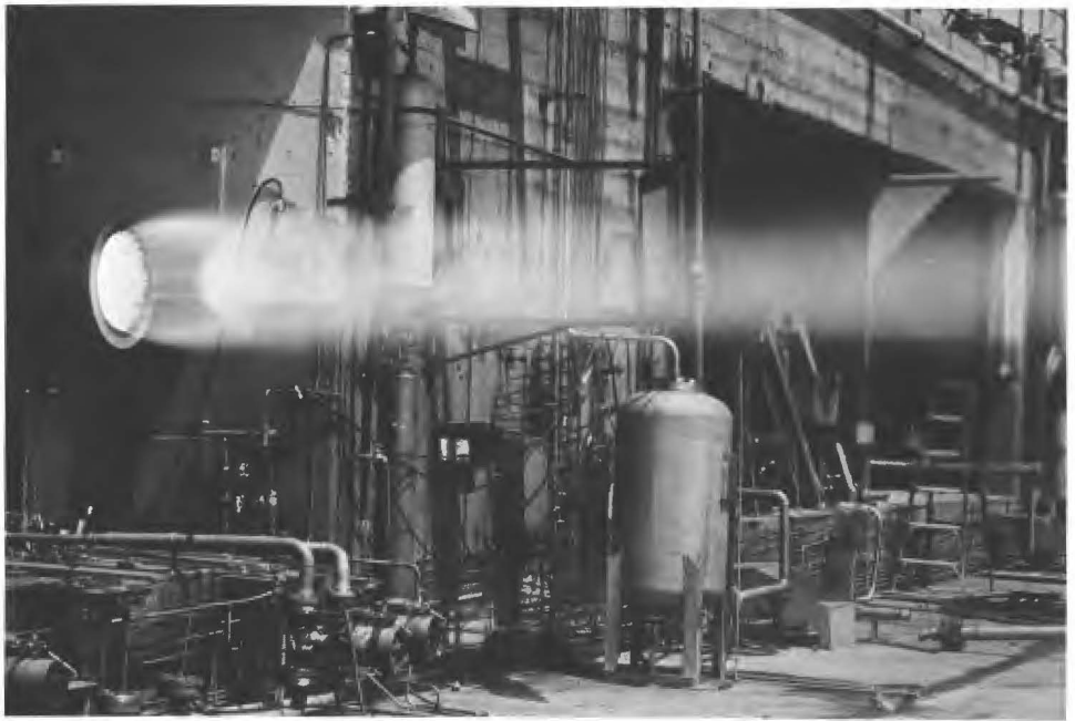
A prototype of the main engine of the Apollo service module test-fired at Aerojet-General Corporation's Azusa, Calif., plant in August 1962. The engine used storable liquid propellants and had an ablative thrust chamber assembly. (Aerojet-General photo)
