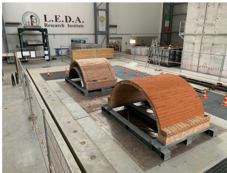
Figure 1. Photographic image of the unreinforced (UV) and reinforced (RV) masonry vaults fixed on the shaking table system of LEDA Laboratory of Enna Kore University.
