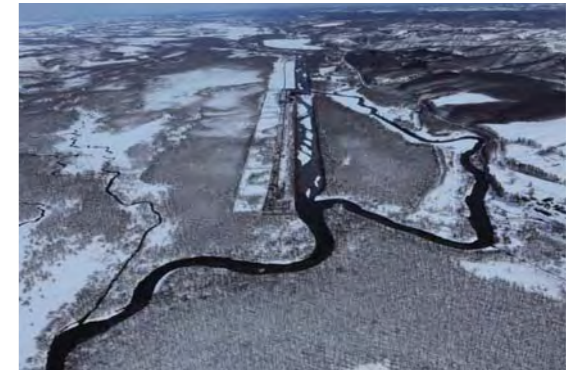
農地開発等のため直線化した河道を蛇行河川に復元 A part of river channel in Kushiro River was restored as a meandering river, which was once straightened for developing farmlands.
