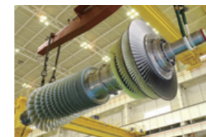
2011 World's most-efficient J-series gas turbine achieves record turbine inlet temperature of 1,600°C during demonstration test
