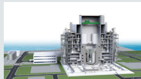
Sodium-cooled tank-based fast reactor (includes research results from projects commissioned by the Ministry of Economy, Trade and Industry)
